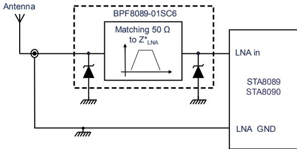
**Figure 2. Solution for active antenna**
