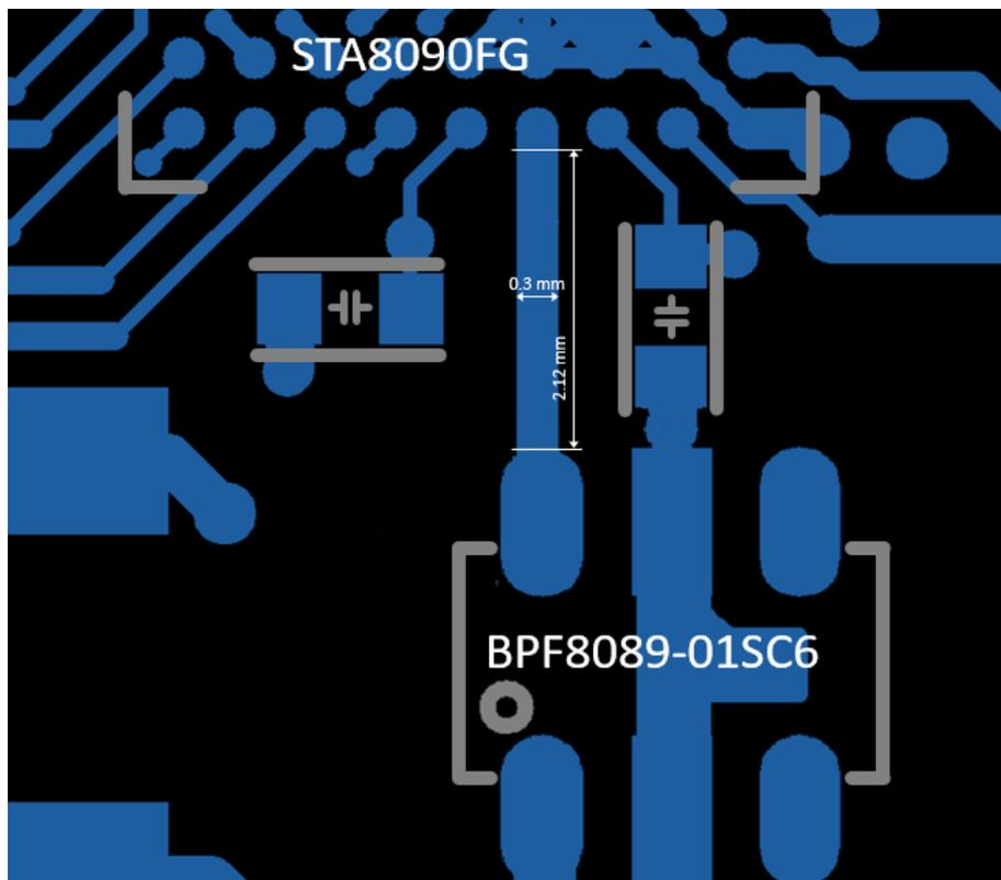
**Figure 8. Recommended layout for STA8089WG**
