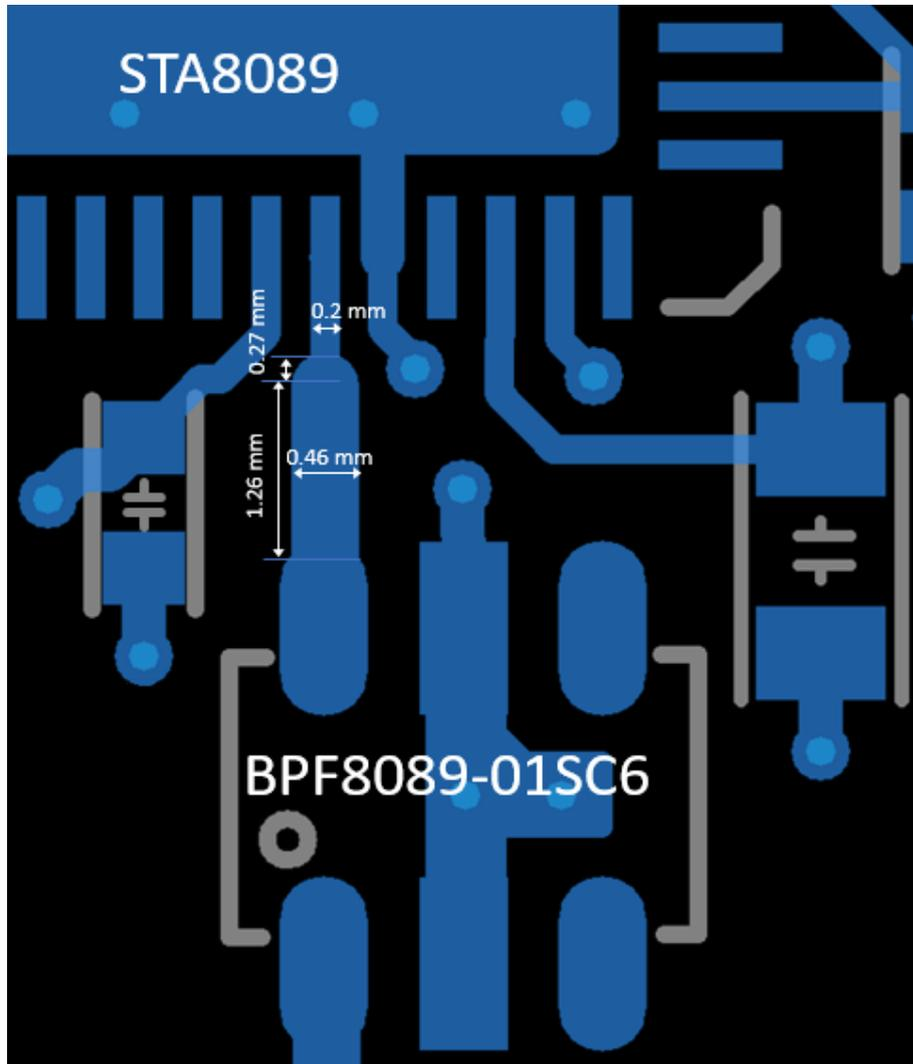
**Figure 7. Recommended layout for STA8089FG**
