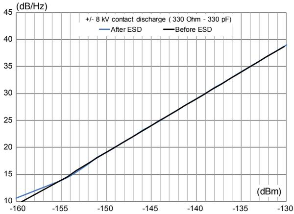
**Figure 4. Response to IEC 61000-4-2 (C = 150 pF, R = 330 Ω, -8 kV contact discharge)**
