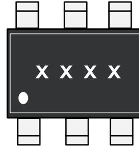
**Figure 14. Package orientation in reel**
