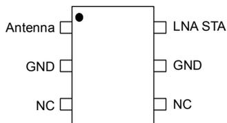
NC: pin internally not connected and not to be connected on PCB
