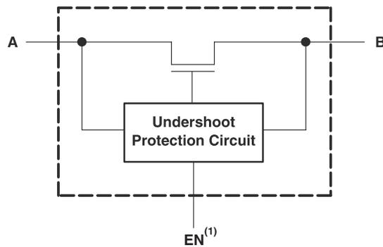
(1) EN is the internal enable signal applied to the switch.
