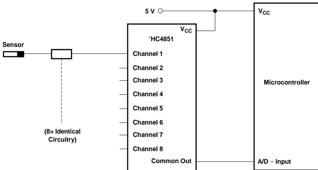
Figure 3. Solution by Applying the 'HC4851 Multiplexer
