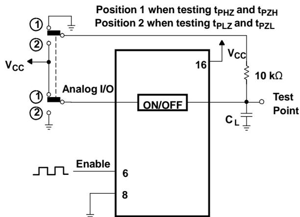
**Figure 14. Propagation-Delay Test Setup, Enable to Analog Out**
