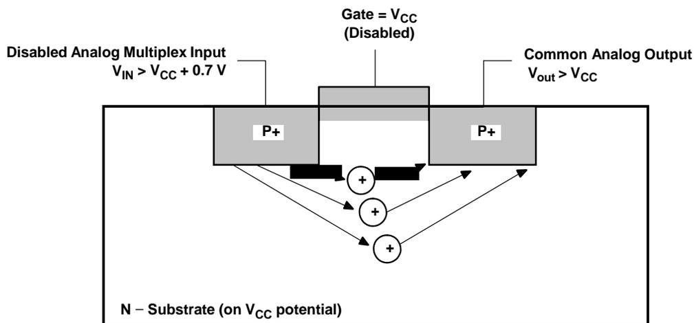
Figure 4. Diagram of Bipolar Coupling Mechanism
