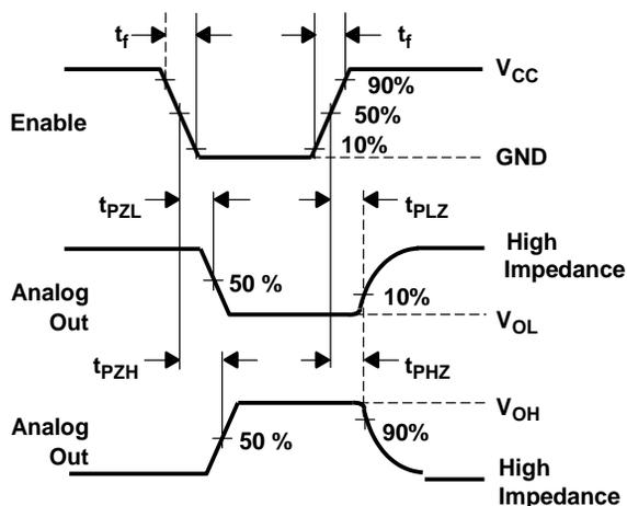
**Figure 13. Propagation Delays, Enable to Analog Out**
