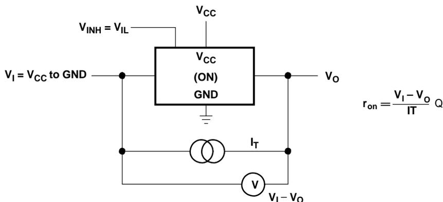
Figure 5. On-State-Resistance Test Circuit
