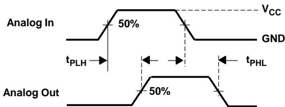
Figure 11. Propagation Delays, Analog In to Analog Out
