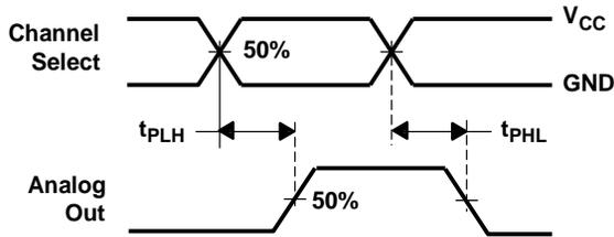
Figure 9. Propagation Delays, Channel Select to Analog Out
