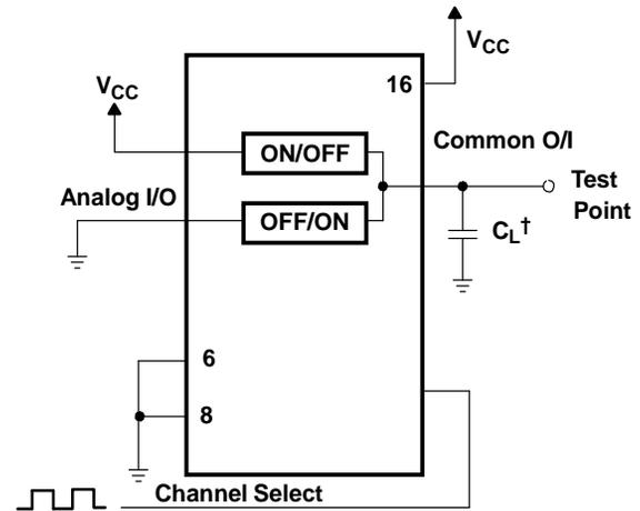
† Includes all probe and jig capacitance
