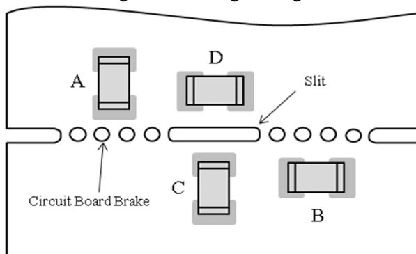
Stress strength according to the mounting position:
