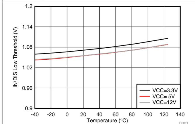
Figure 20. IN/DIS Low Threshold
