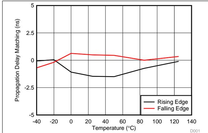
Figure 16. Propagation Delay Matching (t<sub>DM</sub>) vs. Temperature
