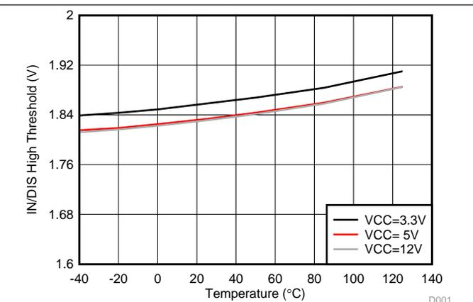
Figure 21. IN/DIS High Threshold
