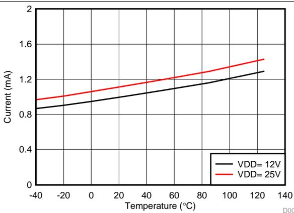
Figure 8. Per Channel ( $I_{VDDA/B}$ ) Quiescent Supply Current vs Temperature (No Load, Input Low, No Switching)
