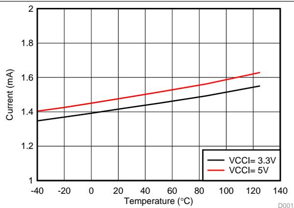
Figure 9.  $I_{VCCI}$  Quiescent Supply Current vs Temperature (No Load, Input Low, No Switching)
