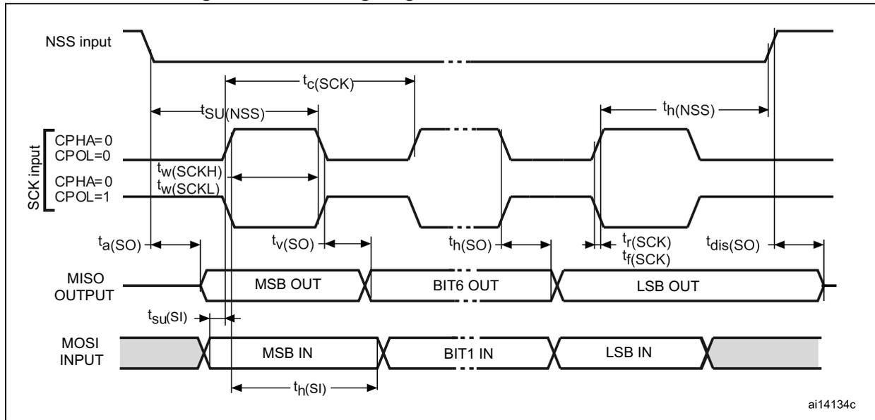
Figure 25. SPI timing diagram - slave mode and CPHA = 1
