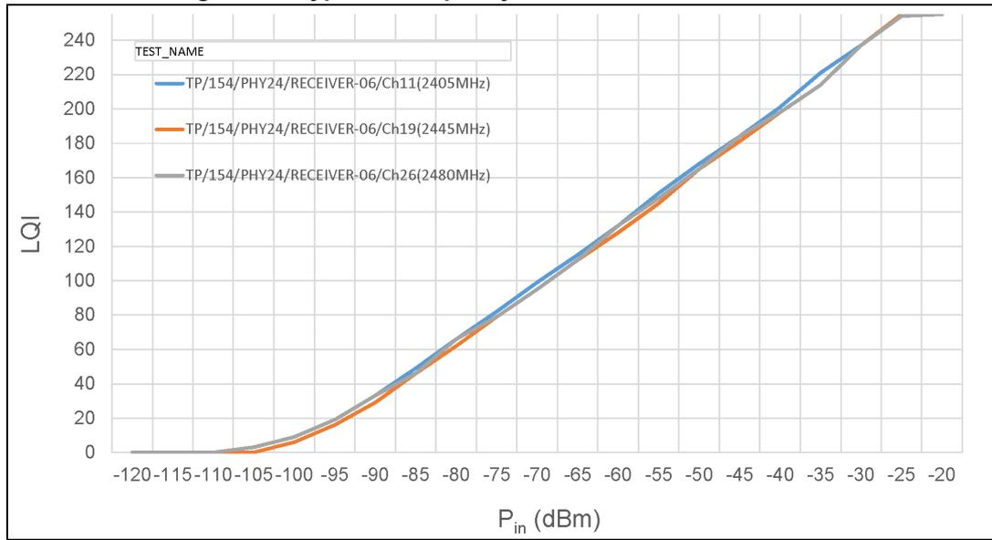
Figure 14. Typical energy detection (T = 27°C, V<sub>DD</sub> = 3.3 V)
