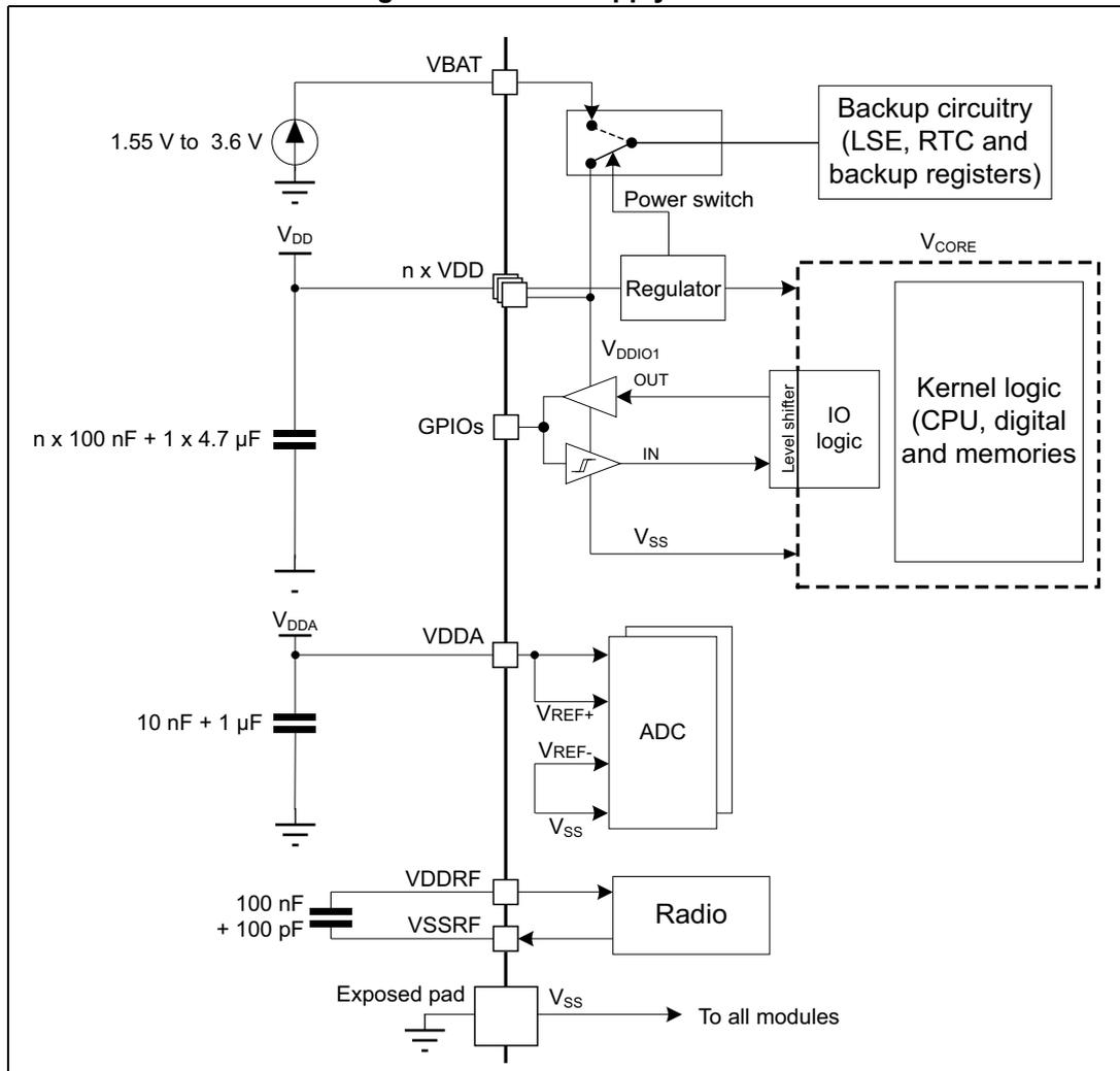
**Caution:** Each power supply pair (such as  $V_{DD} / V_{SS}$ ,  $V_{DDA} / V_{SS}$ ) must be decoupled with filtering ceramic capacitors as shown in [Figure 11](#). These capacitors must be placed as close as possible to (or below) the appropriate pins on the underside of the PCB to ensure the good functionality of the device.
