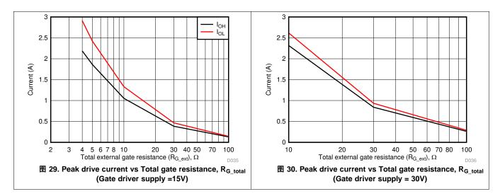
Use  $\frac{1}{8}$  6 to find the minimum gate resistance to be used with UCC23511 when driving a power switch. The values shown includes the power switch internal gate resistance  $R_{G_{int}}$ . Hence,  $R_{G_{int}}$  must be subtracted from the values shown to determine the value of the resistor to populate on the printed circuit board.
