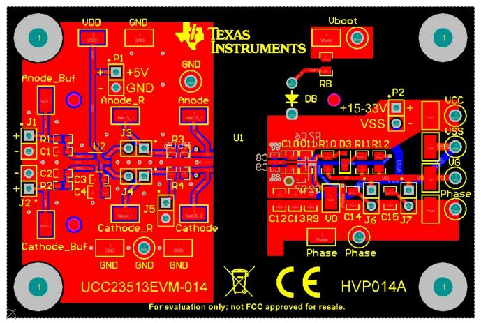
(1) No PCB traces or copper are located between the primary and secondary side, which ensures isolation performance.
