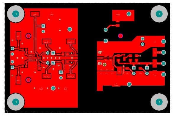
图 32. Top-Layer Traces and Copper
