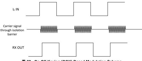
图 20. On-Off Keying (OOK) Based Modulation Scheme
