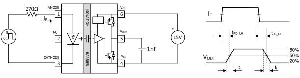
图 16.  $I_F$  to  $V_{OUT}$  Propagation Delay, Rise Time and Fall Time
