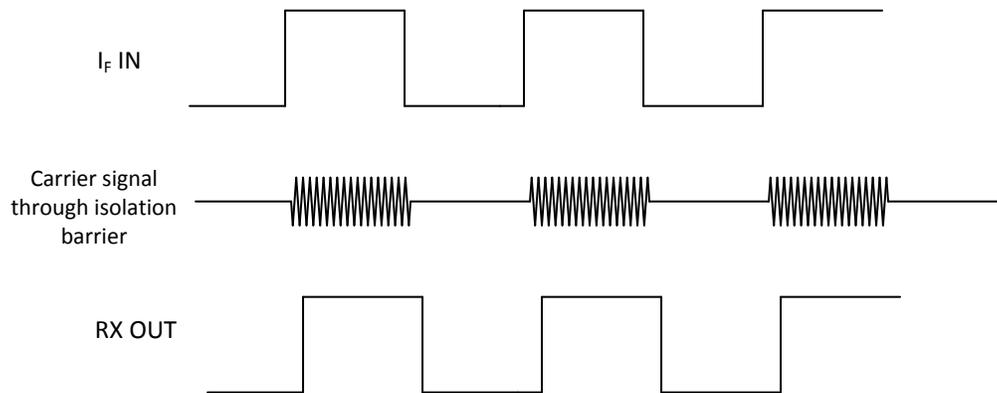
**Figure 8-2. On-Off Keying (OOK) Based Modulation Scheme**
