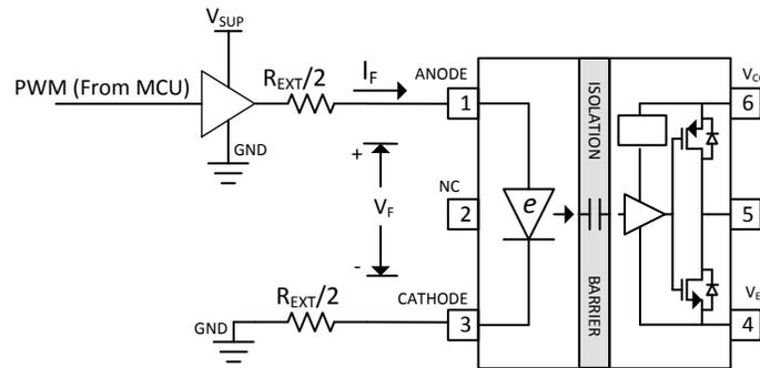
$$R_{EXT} = \frac{V_{SUP} - V_F}{I_F} - R_{OH\_buf}$$
