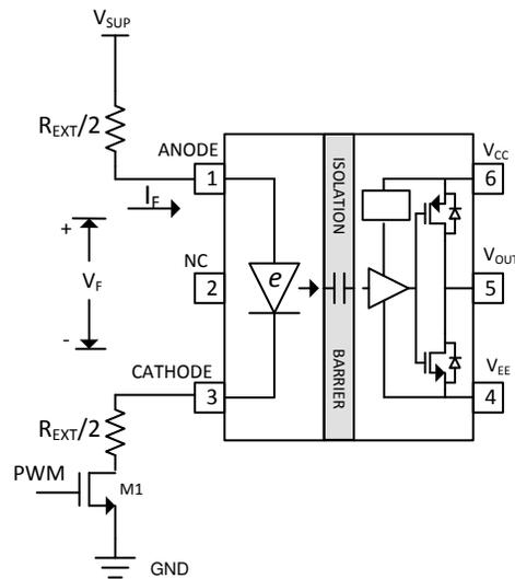
$$R_{EXT} = \frac{V_{SUP} - V_F}{I_F} - R_{M1}$$
