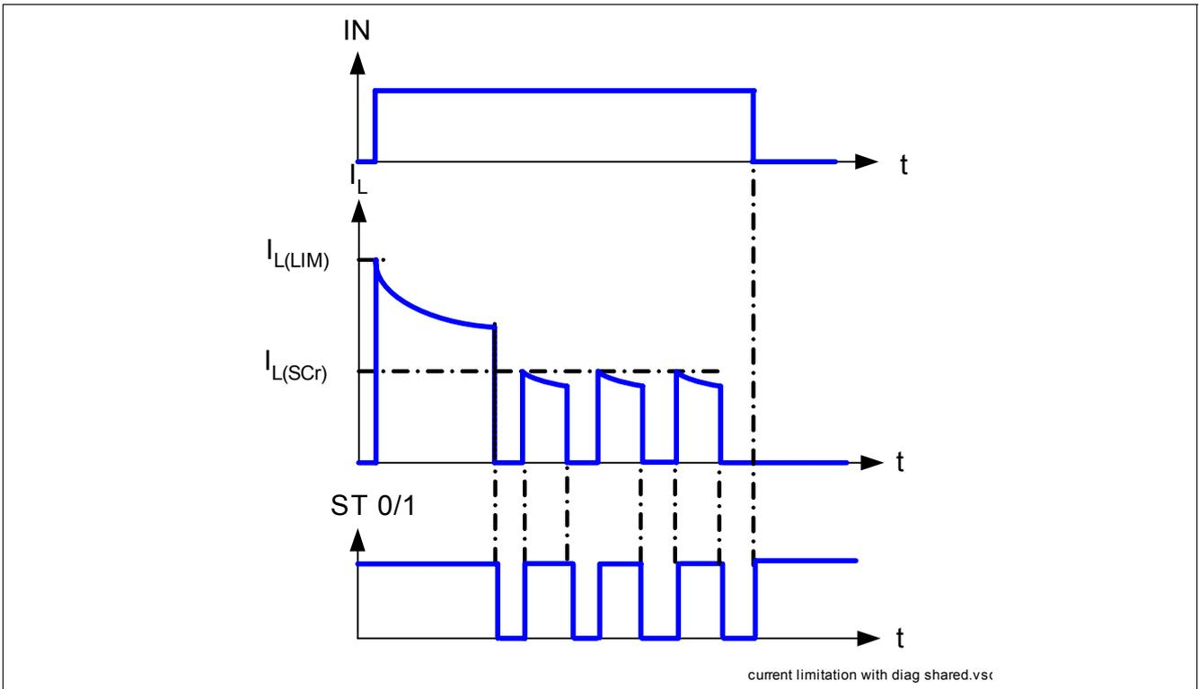
**Figure 11** Current limitation function of the time
