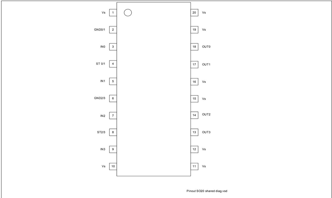
Figure 2 Pin Configuration
