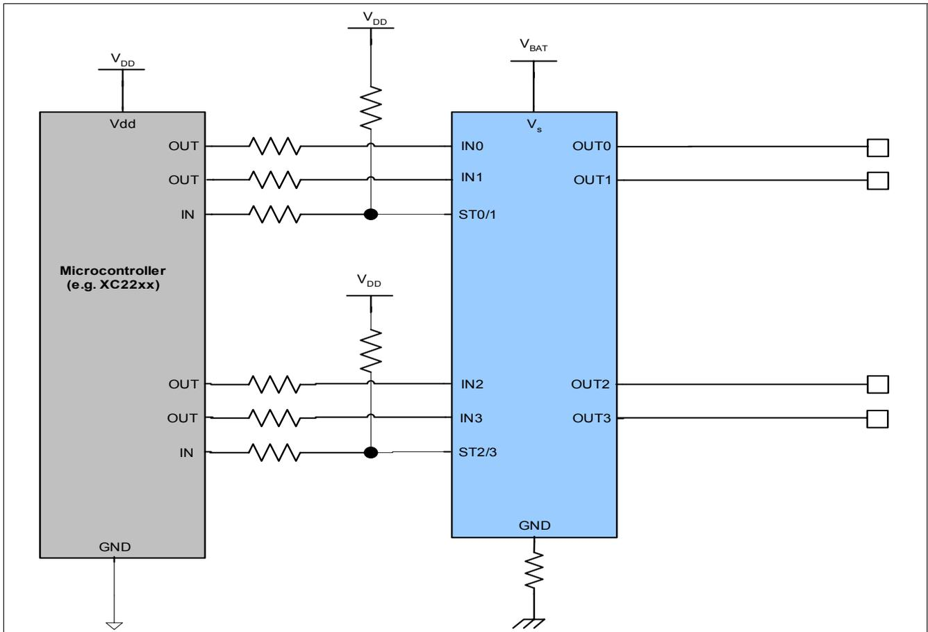
**Figure 17 Application diagram with BTS4130QGA**
