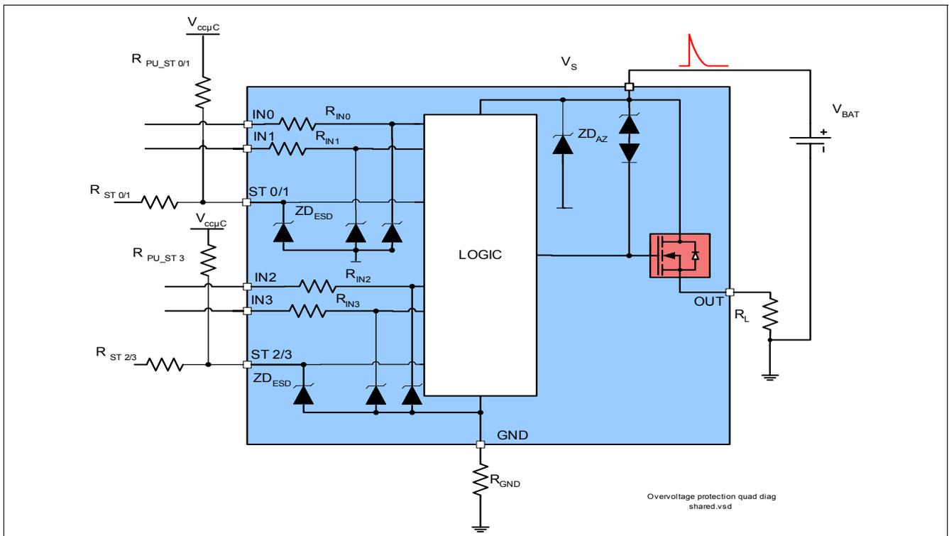
**Figure 9** Over voltage protection with external components
