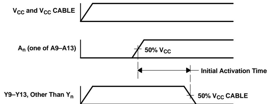
One of pins A9–A13 is switched as shown above, and the other four inputs are forced at low state.
