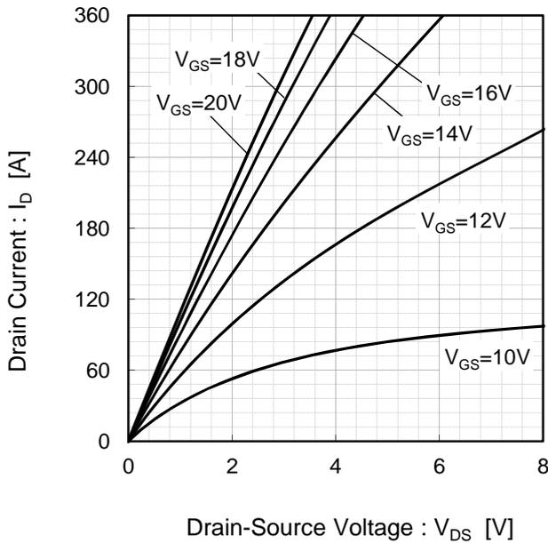
Fig.2 Drain-Source Voltage vs. Drain Current [  $T_j=25^\circ\text{C}$  ]
