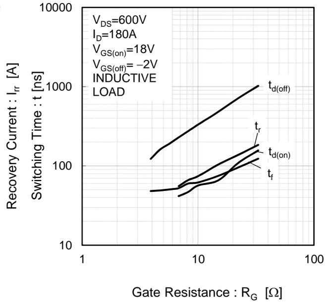
Fig.19 Switching Characteristics vs. Gate Resistance [  $T_j=125^{\circ}\text{C}$  ]
