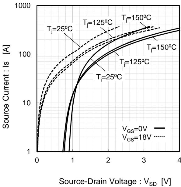
Fig.6 Forward characteristic of Diode
