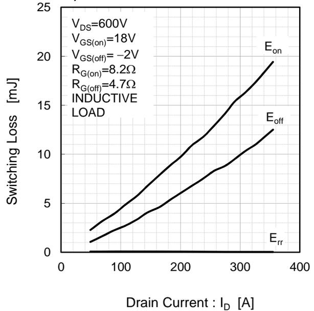
Fig.15 Recovery Characteristics vs. Drain Current [  $T_j=25^{\circ}\text{C}$  ]
