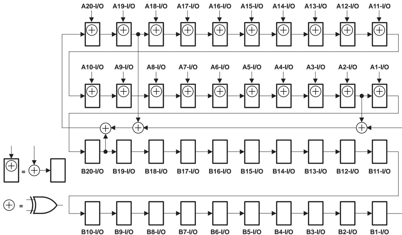
**Figure 7. 40-Bit PSA Configuration ( $\overline{OEAB} = 0$ ,  $\overline{OEBA} = 1$ )**
