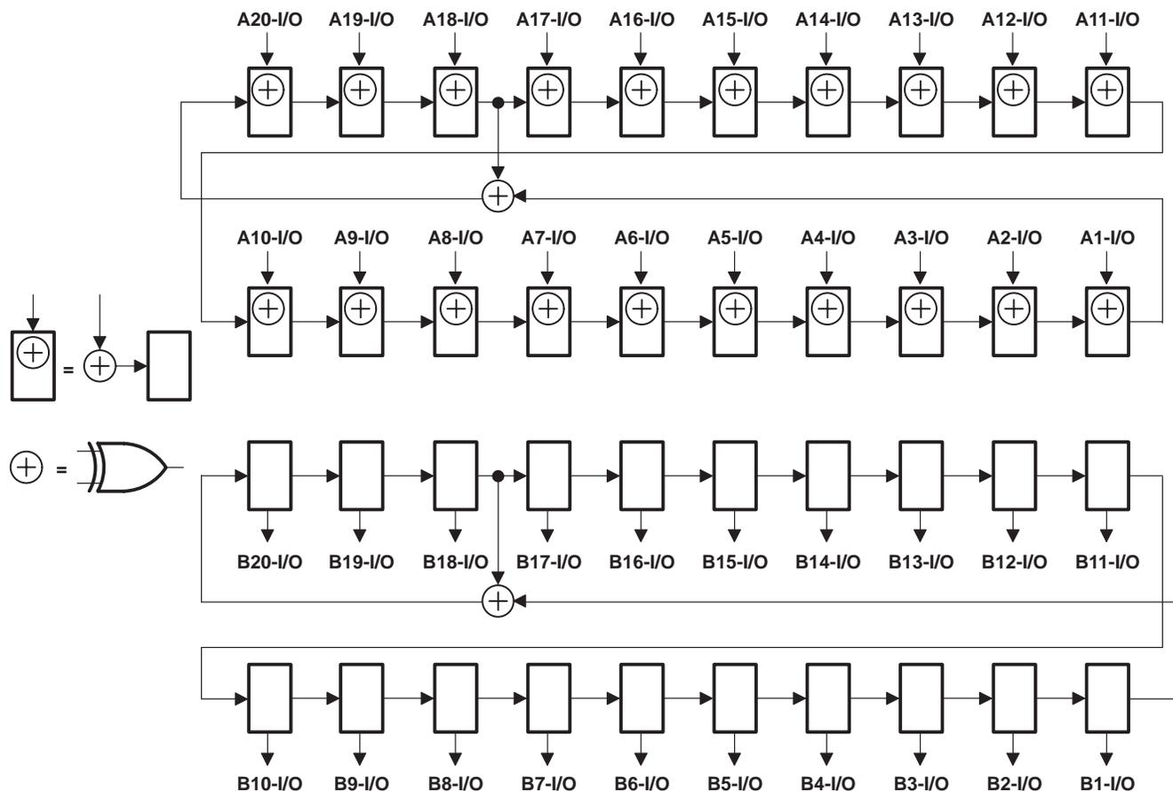
**Figure 9. 20-Bit PSA/PRPG Configuration ( $\overline{OEAB} = 0, \overline{OEBA} = 1$ )**
