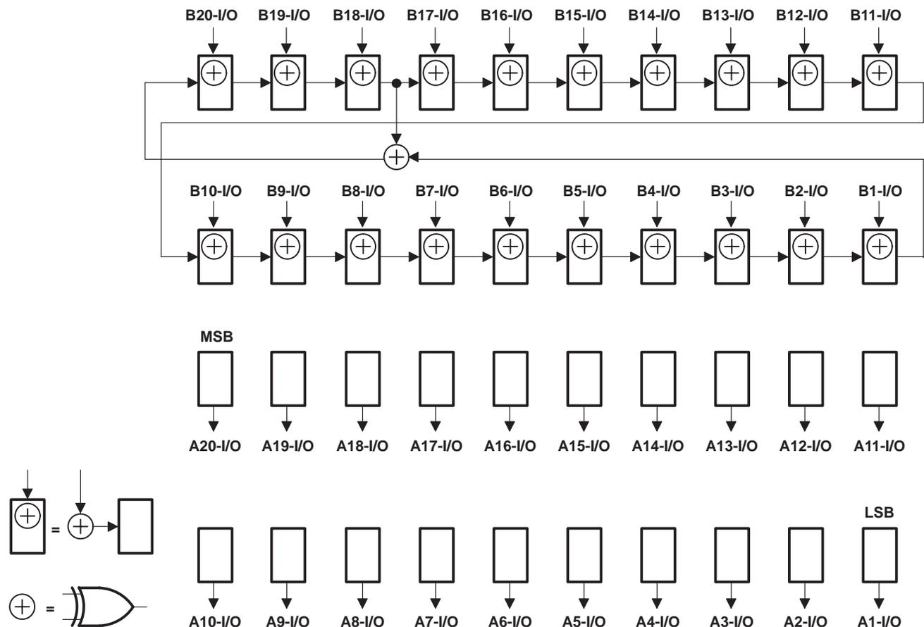
Figure 12. 20-Bit PSA/COUNT Configuration ( $\overline{OEAB} = 1, \overline{OEBA} = 0$ )
