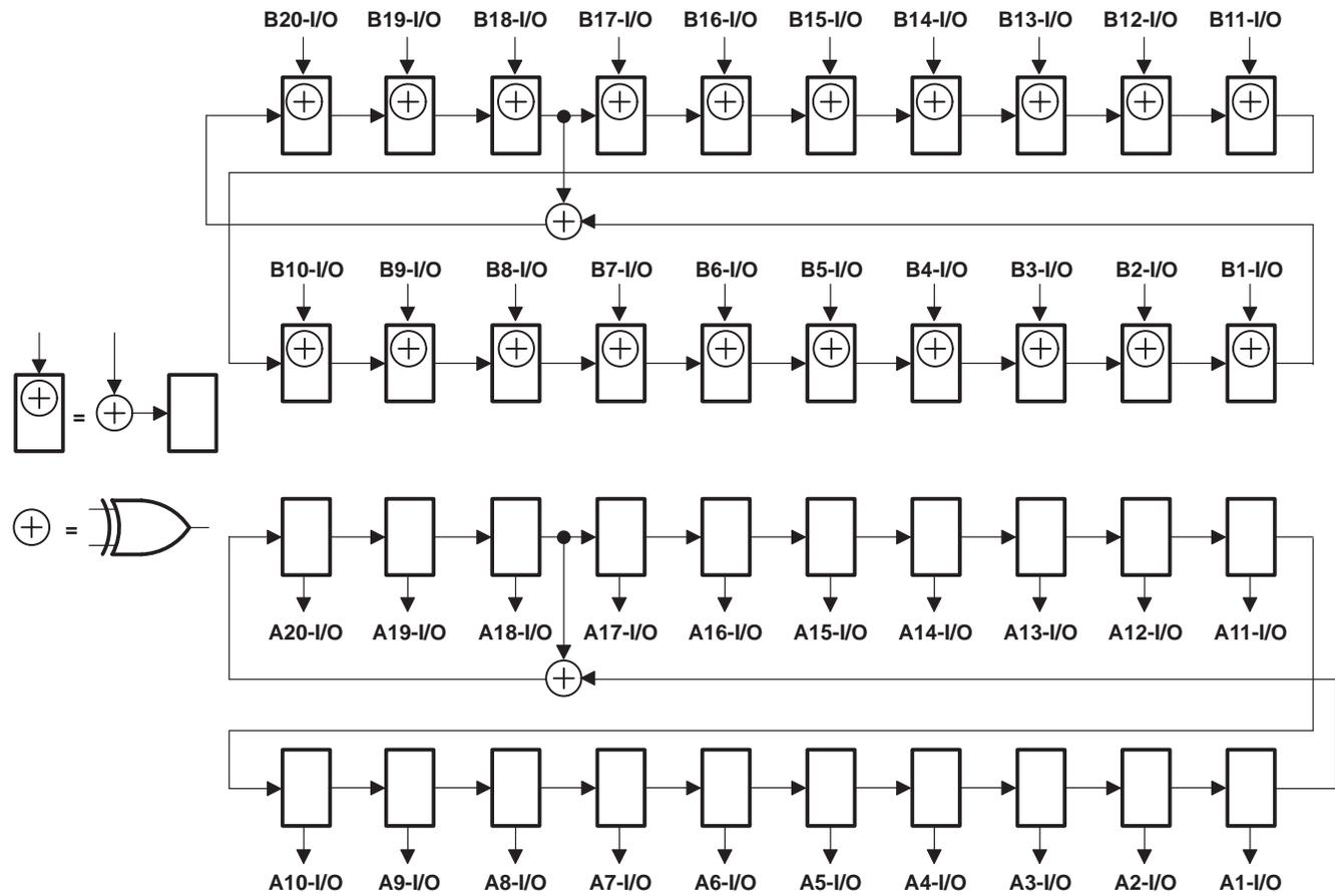
Figure 10. 20-Bit PSA/PRPG Configuration ( $\overline{OEAB} = 1$ ,  $\overline{OEBA} = 0$ )
