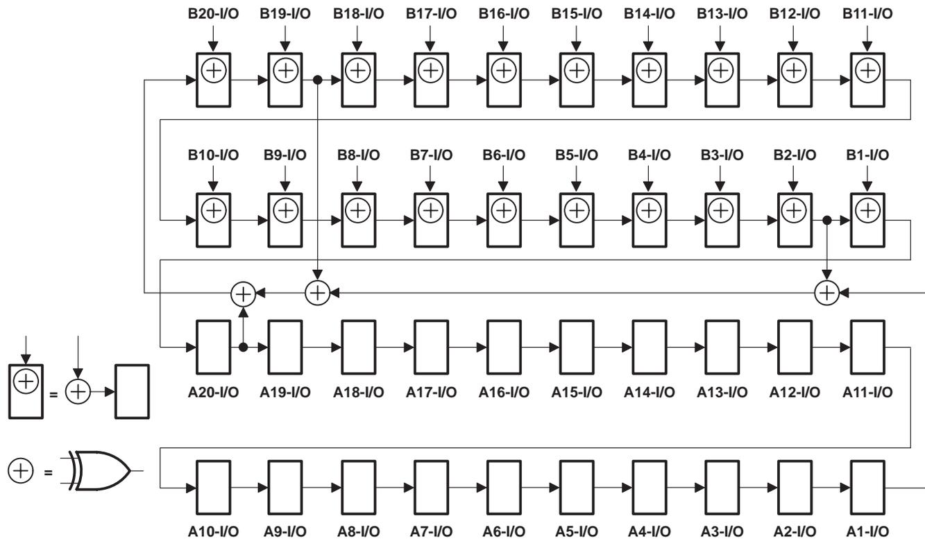
Figure 8. 40-Bit PSA Configuration ( $\overline{OEAB} = 1, \overline{OEBA} = 0$ )
