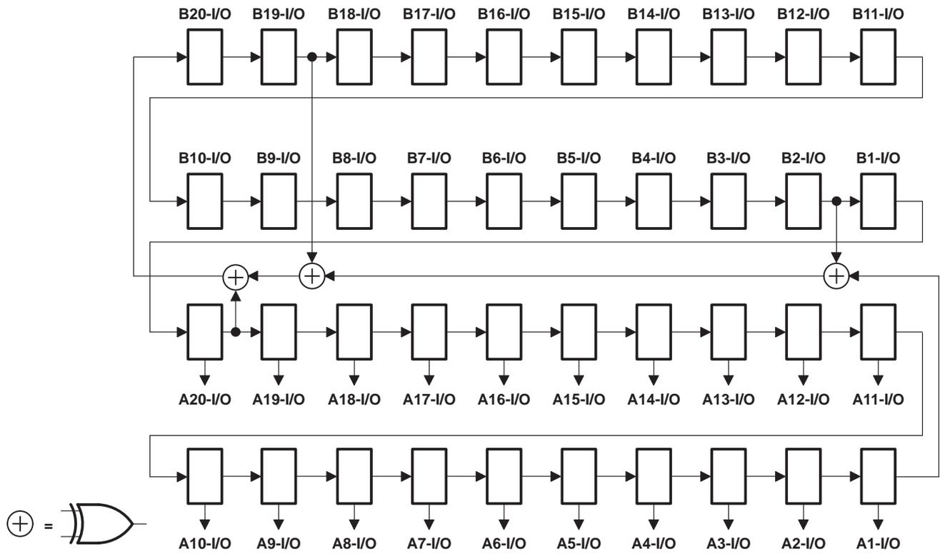
Figure 6. 40-Bit PRPG Configuration ( $\overline{OEAB} = 1, \overline{OEBA} = 0$ )
