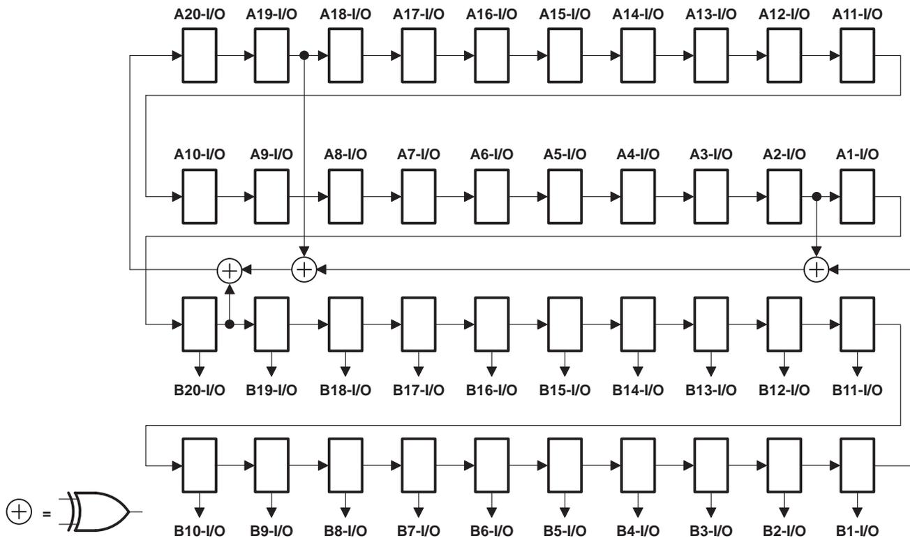
Figure 5. 40-Bit PRPG Configuration ( $\overline{OEAB} = 0$ ,  $\overline{OEBA} = 1$ )
