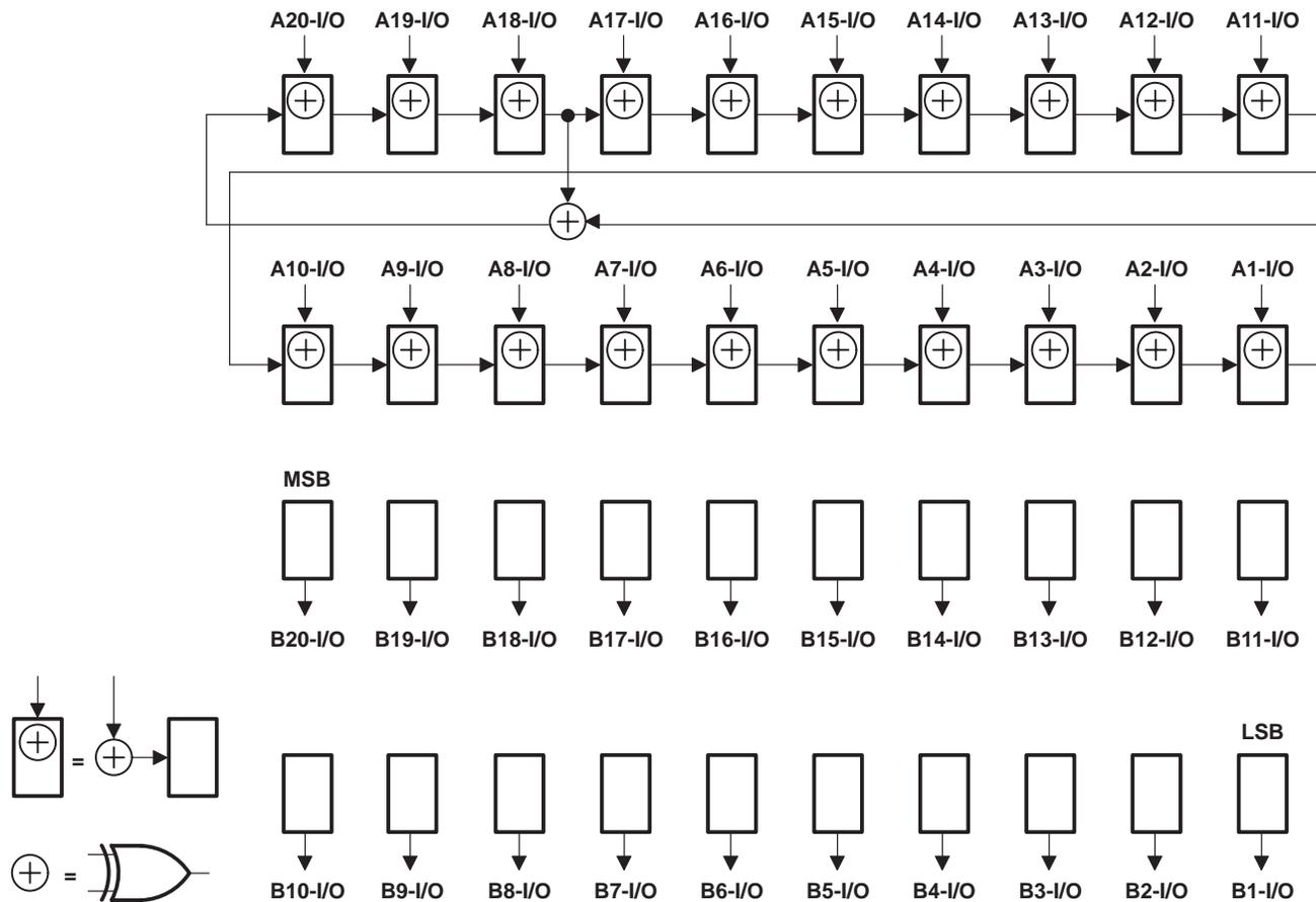
**Figure 11. 20-Bit PSA/COUNT Configuration ( $\overline{OEAB} = 0, \overline{OEBA} = 1$ )**
