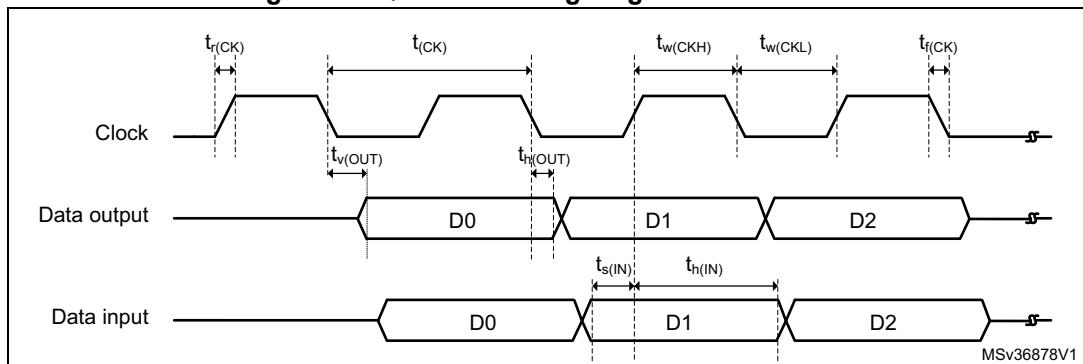
**Figure 53. Quad SPI timing diagram - DDR mode**
