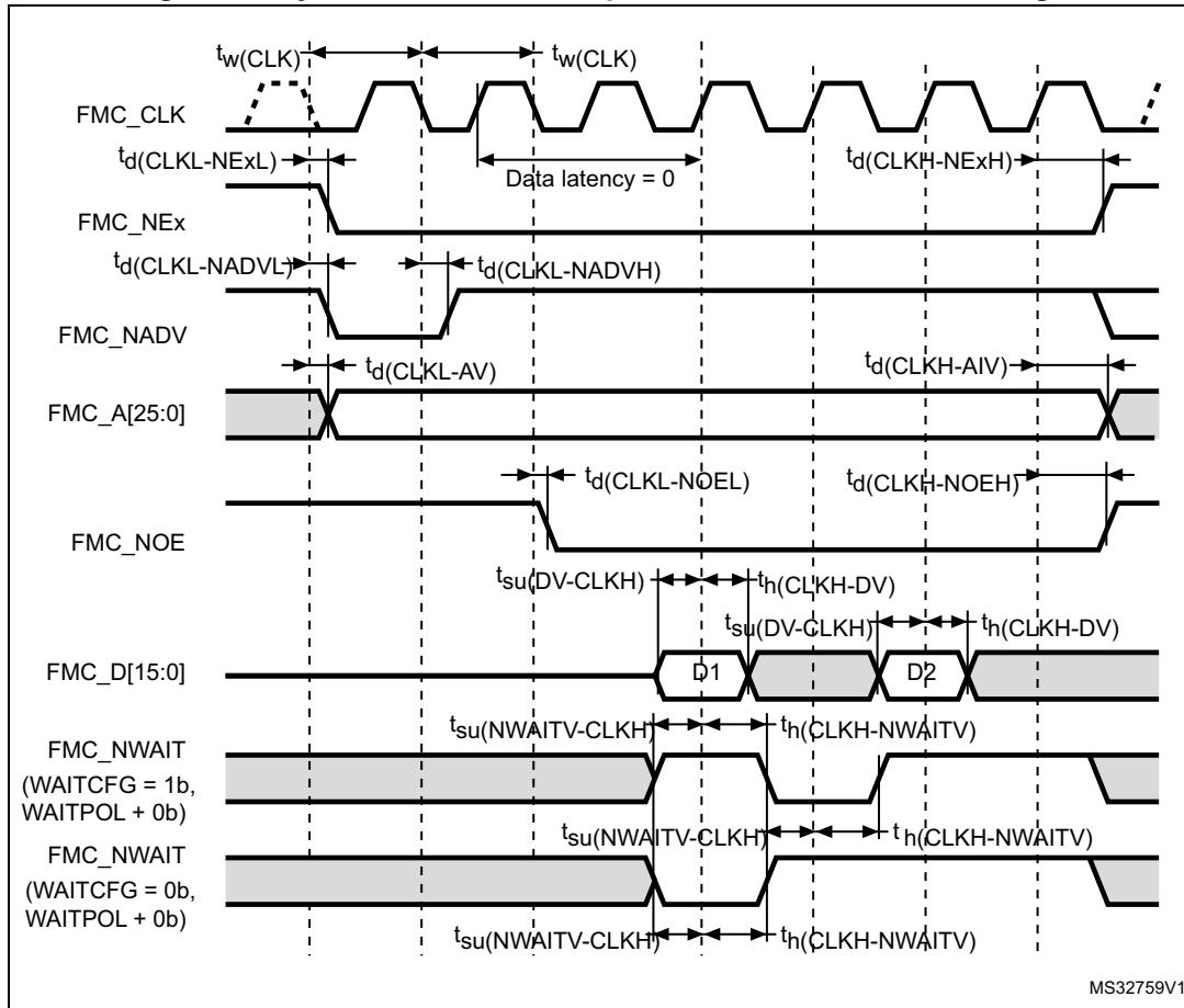
Table 99. Synchronous non-multiplexed NOR/PSRAM read timings<sup>(1)(2)(3)</sup>
