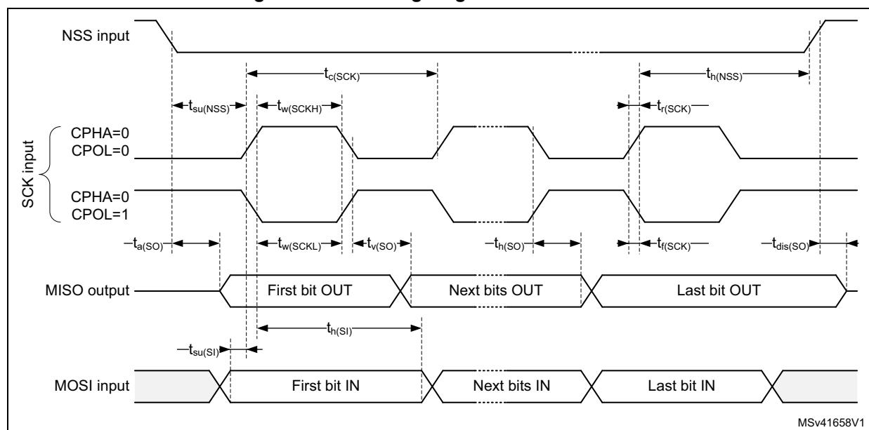
Figure 36. SPI timing diagram - slave mode and CPHA = 1
