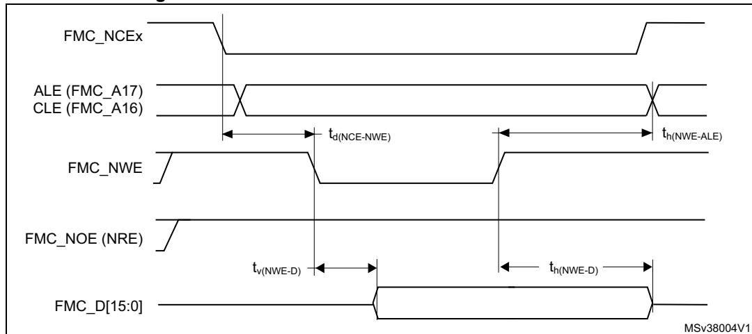
**Figure 50. NAND controller waveforms for common memory read access**
