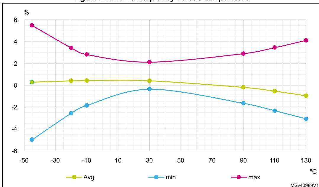
**Low-speed internal (LSI) RC oscillator****Table 45. LSI oscillator characteristics<sup>(1)</sup>**
