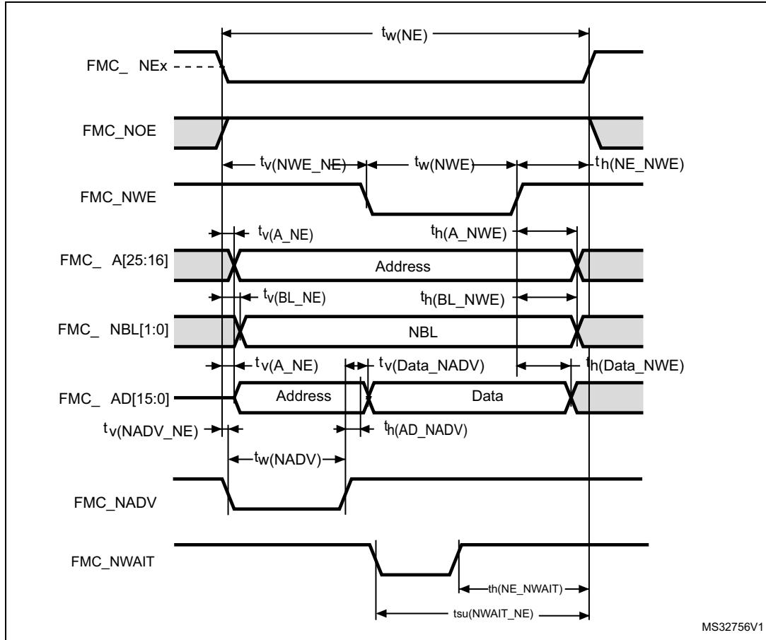
**Table 95. Asynchronous multiplexed PSRAM/NOR write timings<sup>(1)(2)</sup>**
