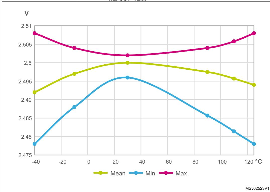
**Figure 33.  $V_{REFOUT\_TEMP}$  in case VRS = 10**
