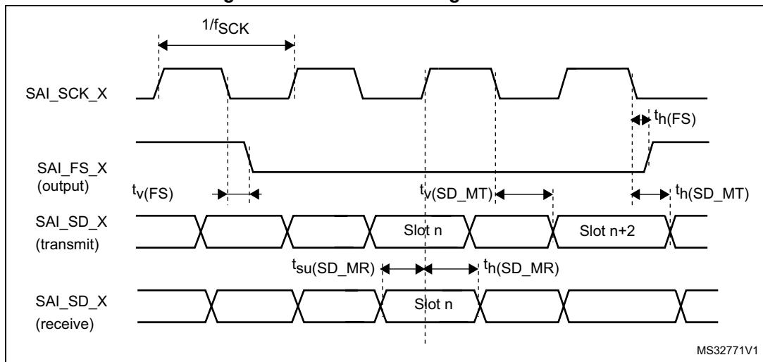
**Figure 39. SAI slave timing waveforms**
