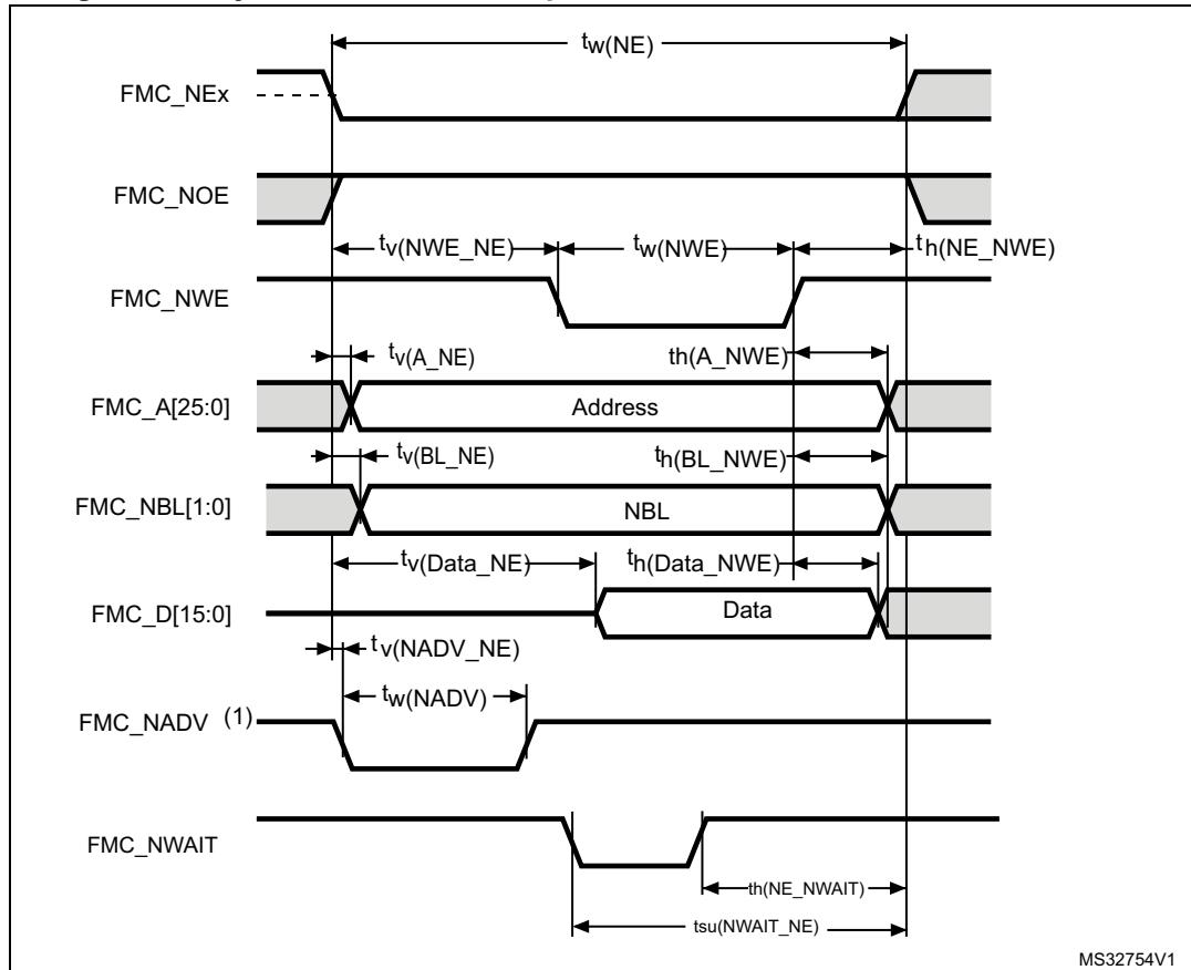
**Table 91. Asynchronous non-multiplexed SRAM/PSRAM/NOR write timings<sup>(1)(2)</sup>**
