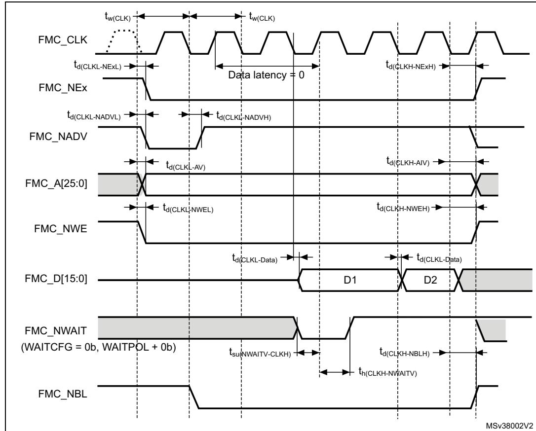
**Table 100. Synchronous non-multiplexed PSRAM write timings<sup>(1)(2)(3)</sup>**
