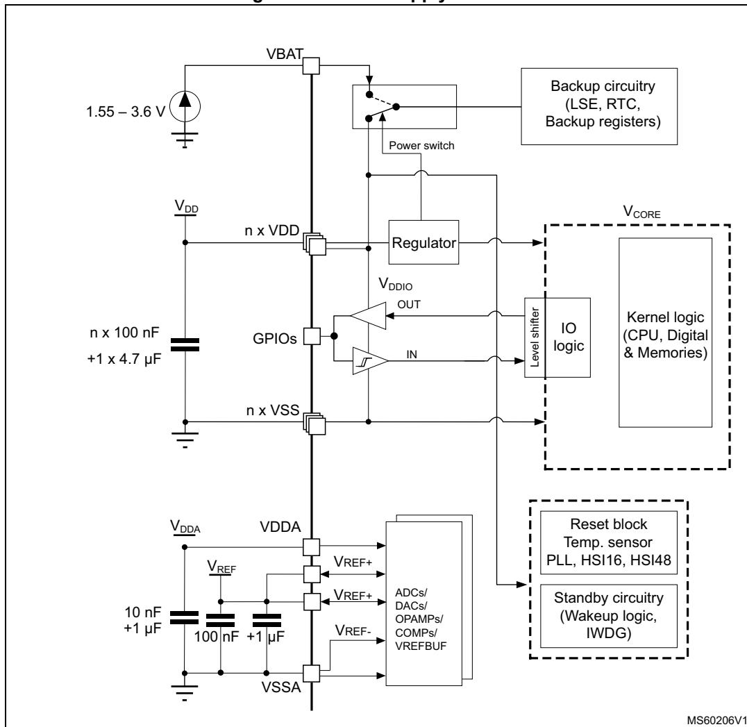
**Caution:** Each power supply pair (V<sub>DD</sub>/V<sub>SS</sub>, V<sub>DDA</sub>/V<sub>SSA</sub> etc.) must be decoupled with filtering ceramic capacitors as shown above. These capacitors must be placed as close as possible to, or below, the appropriate pins on the underside of the PCB to ensure the good functionality of the device.
