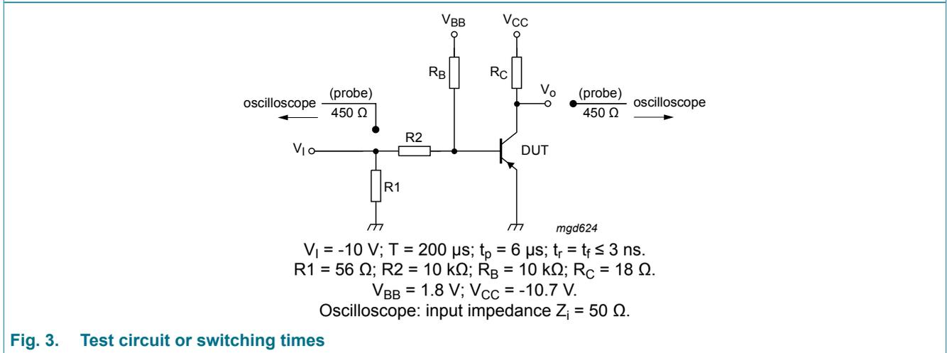
Fig. 3. Test circuit or switching times
