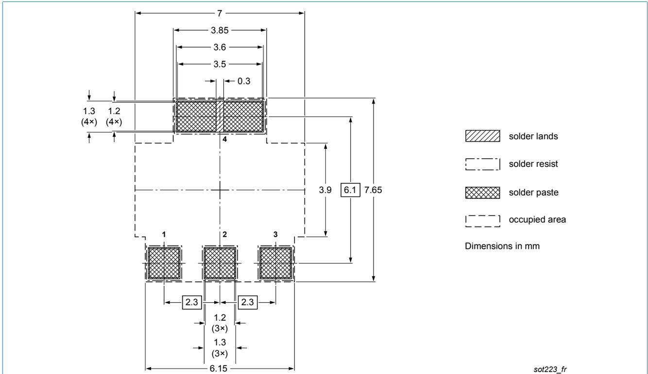
Fig. 5. Reflow soldering footprint for SC-73 (SOT223)
