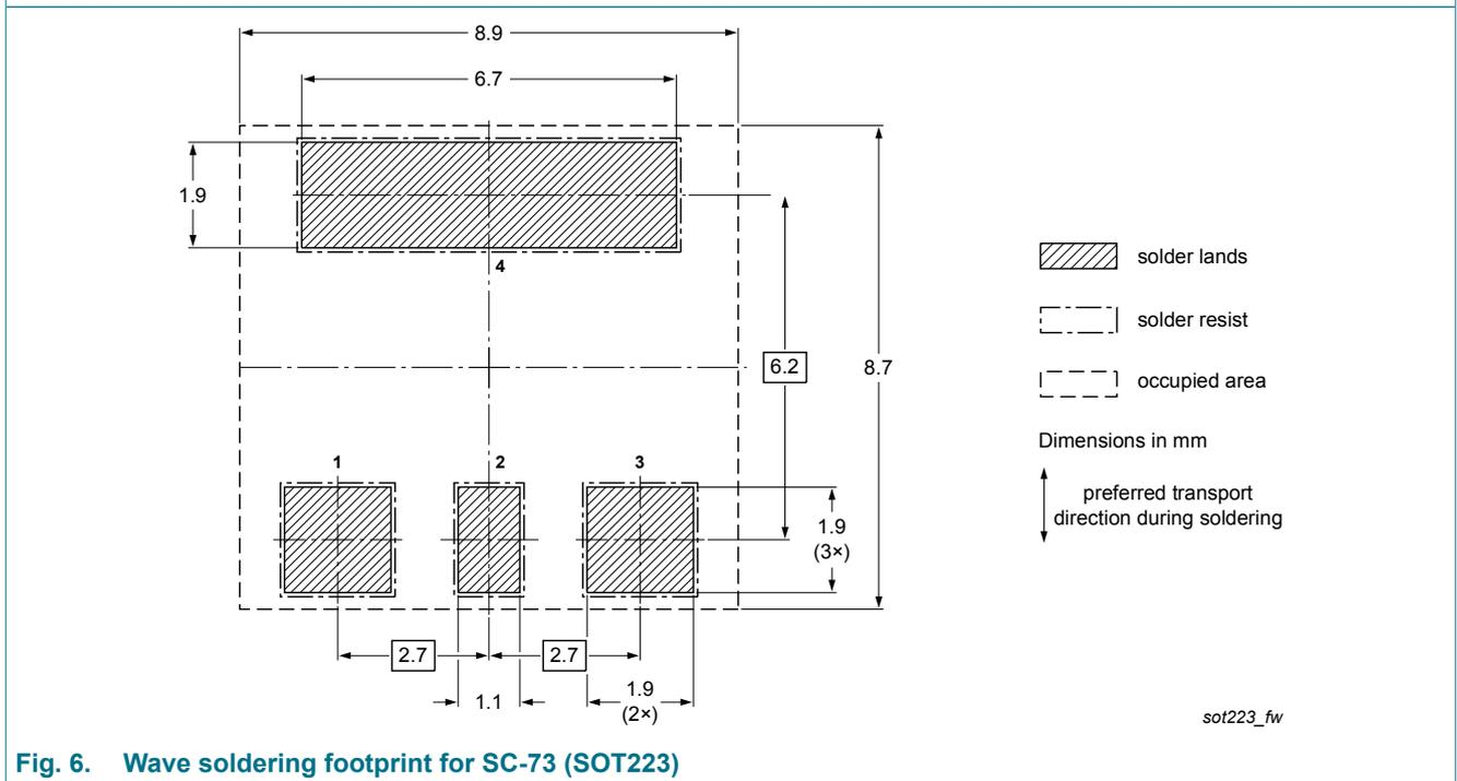
Fig. 6. Wave soldering footprint for SC-73 (SOT223)
