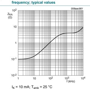
Fig. 18. Dynamic cathode-anode impedance as a function of frequency; typical values
