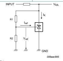
$V_{KA} = V_{ref} x (1 + R1/R2) + I_{ref} x R1$
