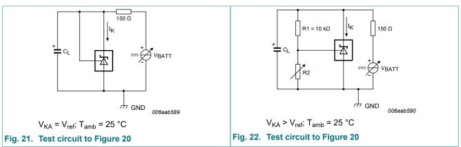
Figures 20, 21 and 22 show the stability boundaries and test circuits for the worst case conditions with a load capacitance mounted as close as possible to the device. The required load capacitance for stable operation varies depending on the operating temperature and capacitor Equivalent Series Resistance (ESR). Verify that the application circuit is stable over the anticipated operating current and temperature ranges.
