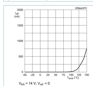
Fig. 10. Off-state current as a function of ambient temperature; typical values
