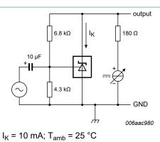
Fig. 17. Test circuit to Figure 16
