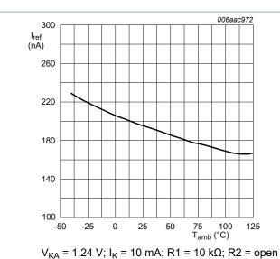
Fig. 7. Reference current as a function of ambient temperature; typical values
