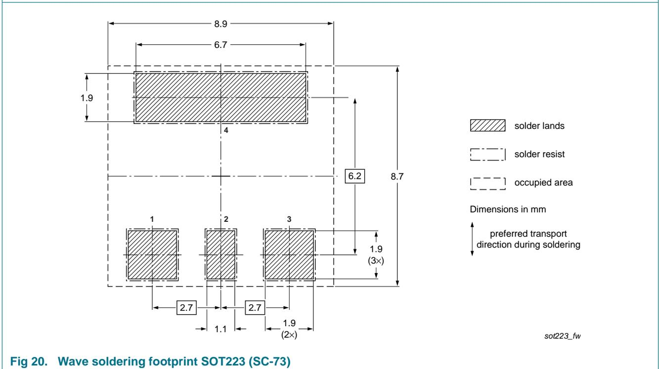
Fig 20. Wave soldering footprint SOT223 (SC-73)
