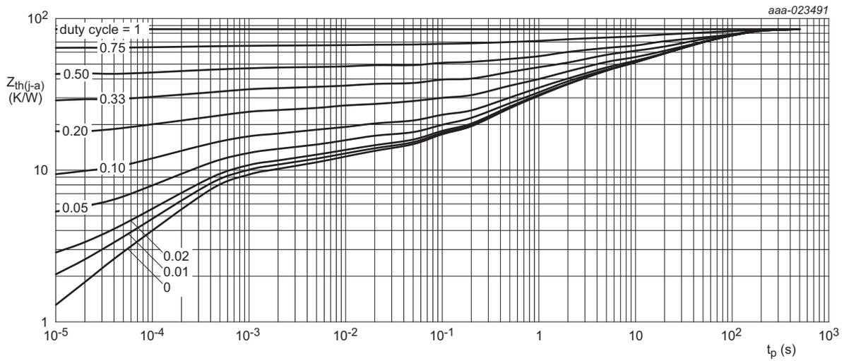
FR4 PCB, single-sided copper, tin-plated; mounting pad for collector 6 cm<sup>2</sup>
