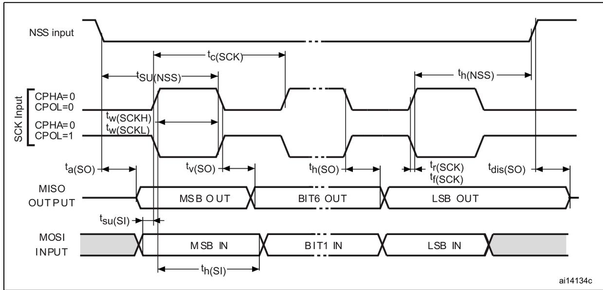
Figure 19. SPI timing diagram - slave mode and CPHA = 1<sup>(1)</sup>
