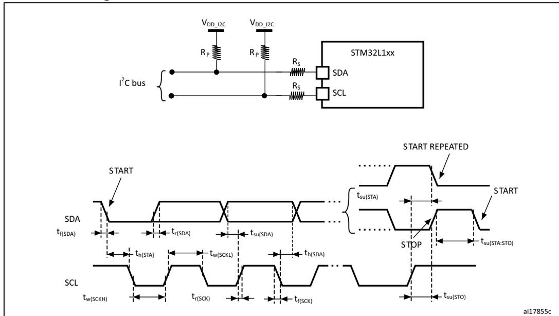
1.  $R_S$  = series protection resistors
