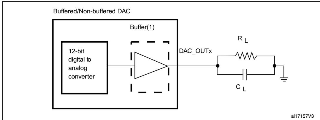
1. The DAC integrates an output buffer that can be used to reduce the output impedance and to drive external loads directly without the use of an external operational amplifier. The buffer can be bypassed by configuring the BOFFx bit in the DAC\_CR register.
