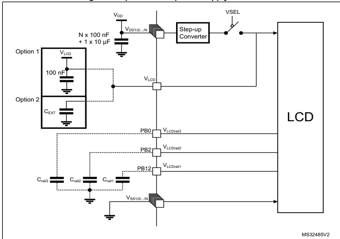
1. Option 1: LCD power supply is provided by a dedicated VLCD supply source, VSEL switch is open.
