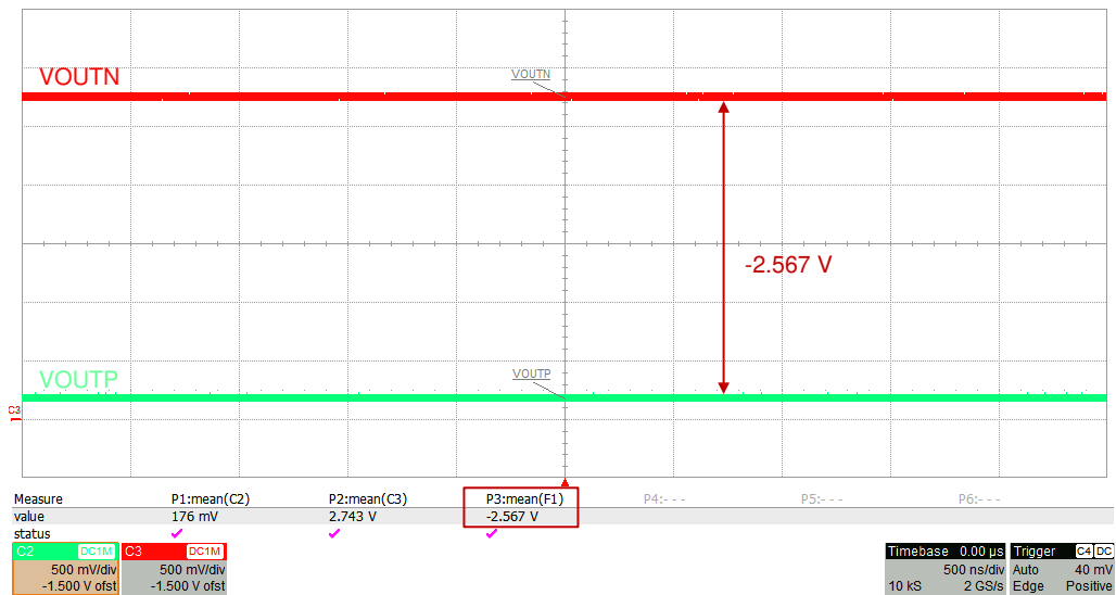
图 7-5. Typical Fail-Safe Output of the AMC3330-Q1
