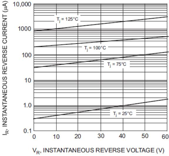
Fig. 7 Typical Reverse Characteristics, SB550 & SB560
