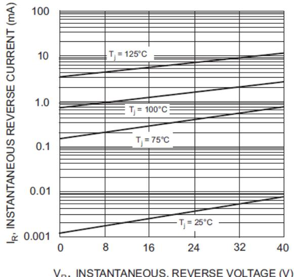
Fig. 6 Typical Reverse Characteristics, SB520 - SB540
