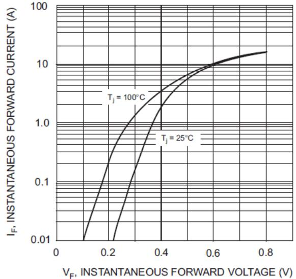
Fig. 2 Typical Forward Characteristics, SB520 - SB540
