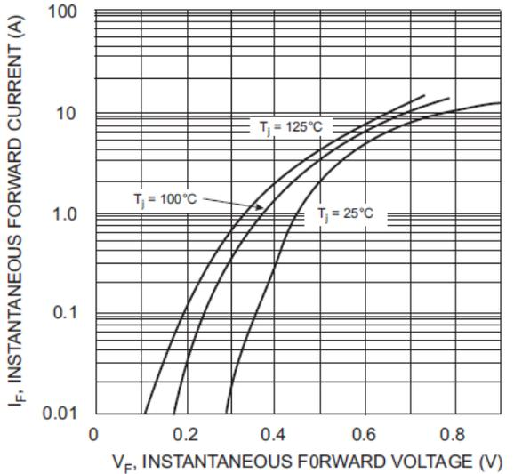
Fig. 3 Typical Forward Characteristics, SB550 & SB560
