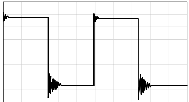
(b) C_L = 130 \text{ pF} , R_L = \text{NO LOAD}
