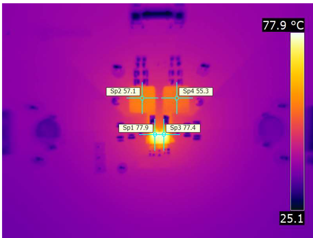
Figure 10-4. Thermal Image at 25°C Ambient - Dual Output Operation, f_{sw} = 1\text{ MHz} , V_{IN} = 12\text{ V} , V_{OUT1} = 1\text{ V} , I_{OUT1} = 6\text{ A} , L_1 = 560\text{ nH} (3.3 mΩ Max), V_{OUT2} = 3.3\text{ V} , I_{OUT2} = 6\text{ A} , L_2 = 1.2\text{ μH} (7.5 mΩ Max)
