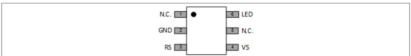
**Figure 2** Pinout BCR431U
