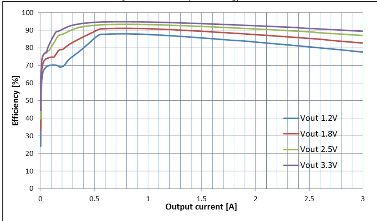
Figure 21. Efficiency curves:  $V_{IN} = 5.0\text{ V}$  (log scale)
