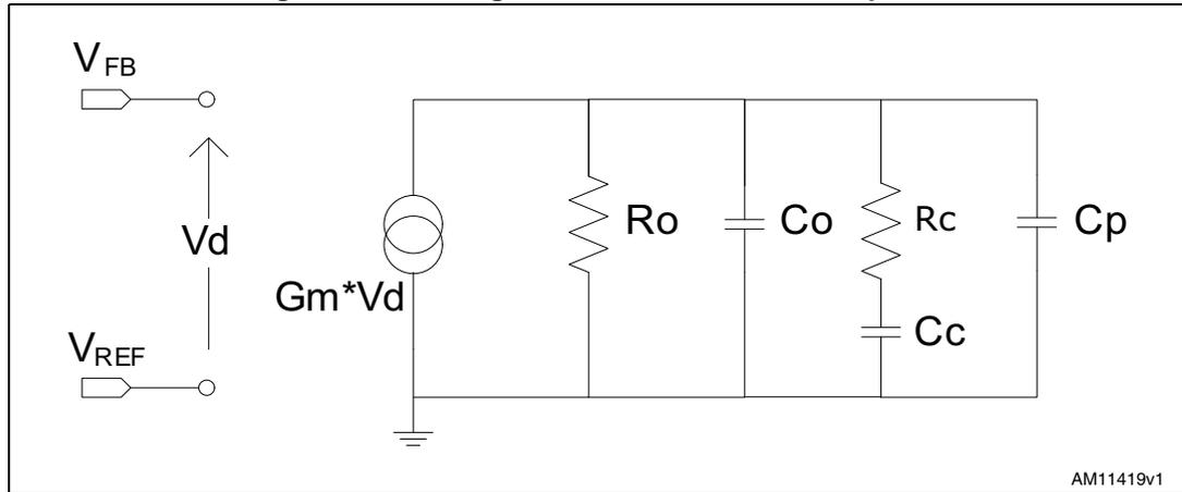
$R_C$  and  $C_C$  introduce a pole and a zero in the open loop gain.  $C_P$  does not significantly affect system stability and can be neglected.
