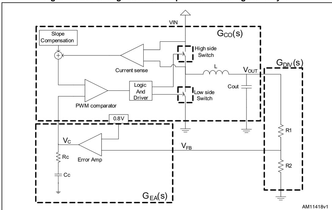
Three main terms can be identified to obtain the loop transfer function:
