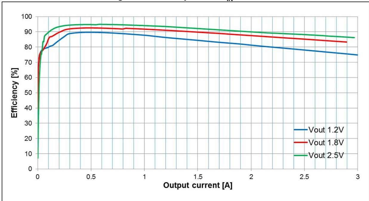
Figure 15. Efficiency curves:  $V_{IN} = 3.3\text{ V}$  (log scale)
