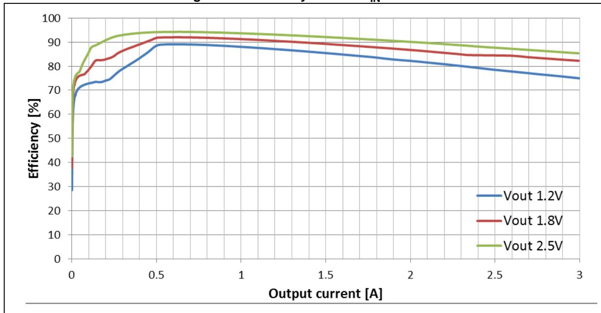
Figure 18. Efficiency curves:  $V_{IN} = 4.0\text{ V}$  (log scale)
