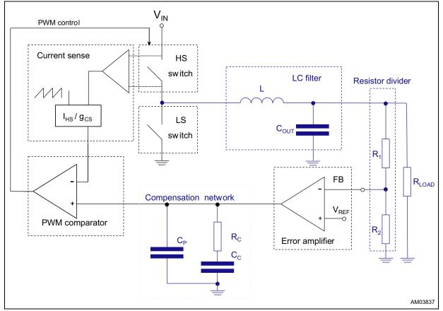
Figure 35. Block diagram of the loop
