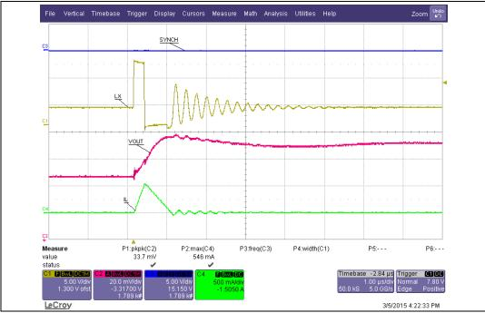
Figure 20. LCM operation with ISKIP<sub>H</sub> = 350 mA typ. at zero load
