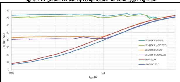
Figure 19. Light-load efficiency comparison at different I<sub>SKIP</sub> - log scale
