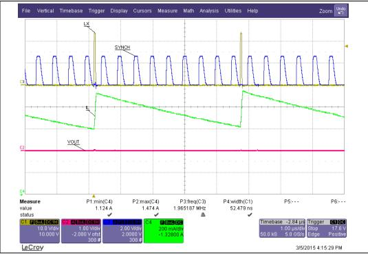
Figure 29. Valley current sense operation in overcurrent condition
