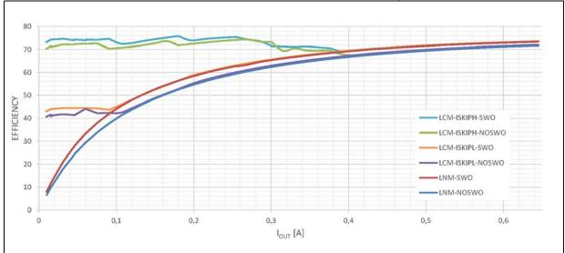
Figure 18. Light-load efficiency comparison at different I<sub>SKIP</sub> - linear scale
