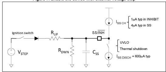
Figure 7. Enable the device with external voltage step
