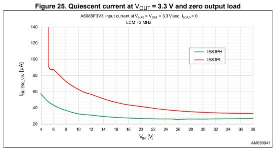
When  $V_{IN}$  is adequately higher than  $V_{OUT}$  (see *Figure 25* and *Figure 26*), the device works in the bursts mode operation, minimizing the power consumption (see *Section 5.8.2: Low consumption mode (LCM)*).
