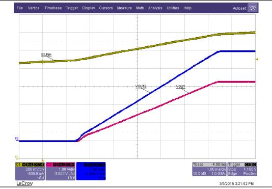
Figure 11. Ratiometric startup operation
