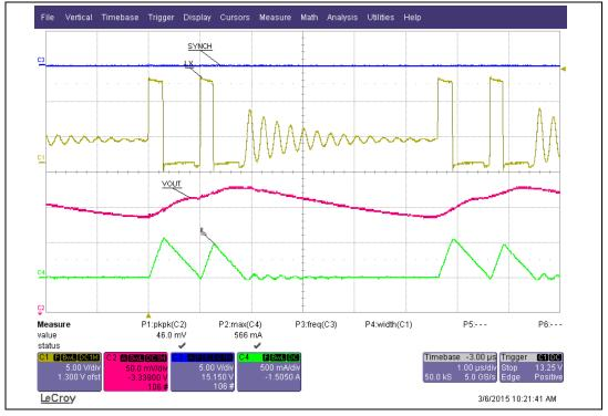
Figure 22. LCM operation over loading condition (part 1)
