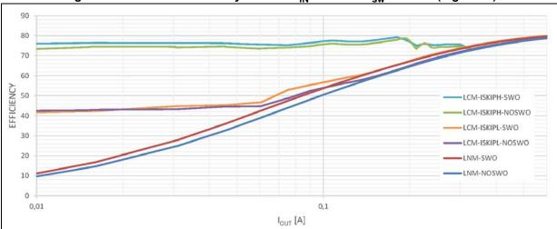
Figure 63. A6985F5V efficiency curves: V<sub>IN</sub> = 13.5 V - f<sub>sw</sub> = 2 MHz (log scale)
