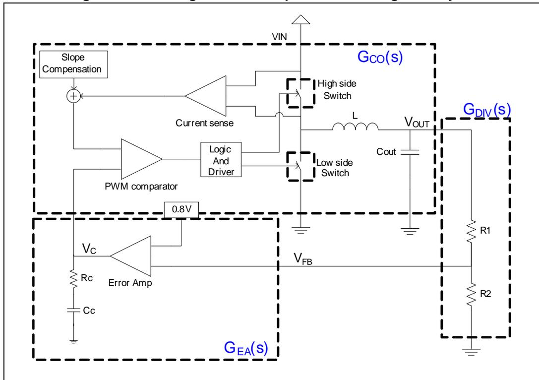
Three main terms can be identified to obtain the loop transfer function:
