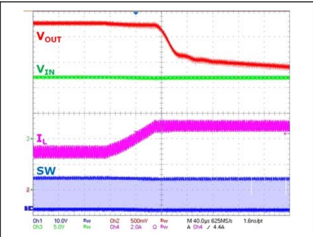
Figure 17. Short-circuit protection
