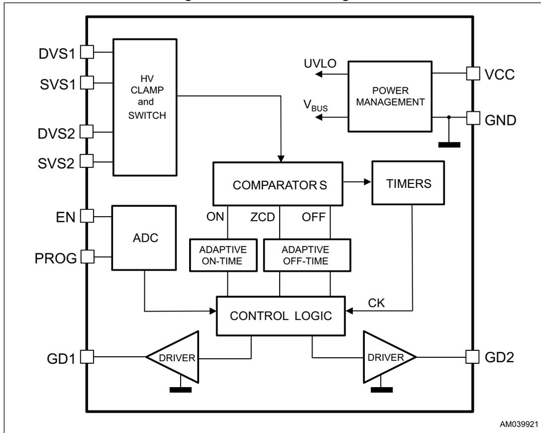
Figure 2. Typical system block diagram
