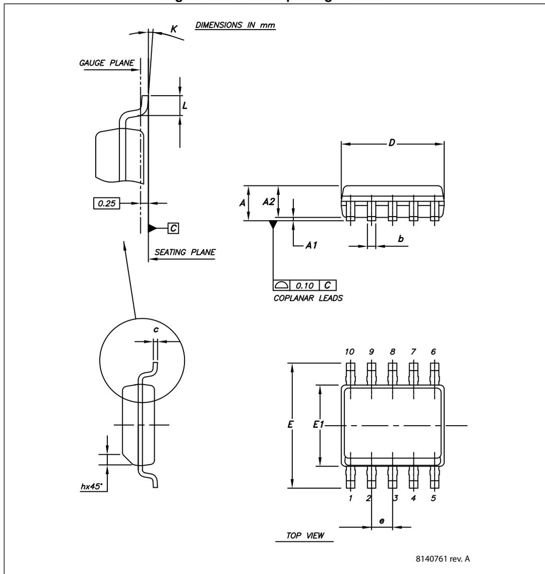
Table 7. SSOP10 package mechanical data
