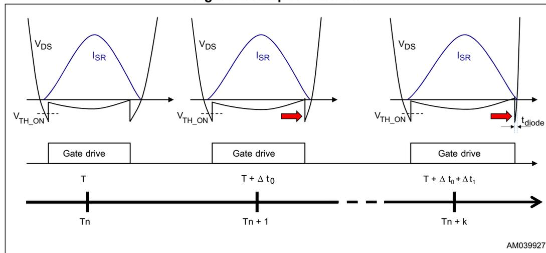
After the turn-on, a blanking time (equal to 50% of the clock period - refer to [Figure 6](#)) masks the adaptive turn-off mechanism in order to avoid an undesired turn-off due to the drain-source voltage drop, consequent to the MOSFET switch-on (the flowing current passes from the body diode to MOSFET channel resistance) or due to the ringing generated at the MOSFET turn-on.
