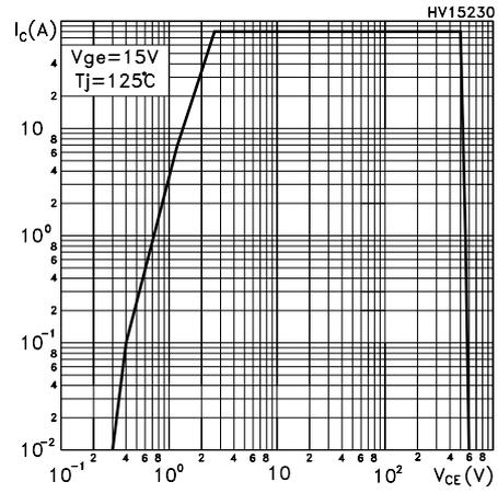
Figure 15. Emitter-Collector Diode Characteristics
