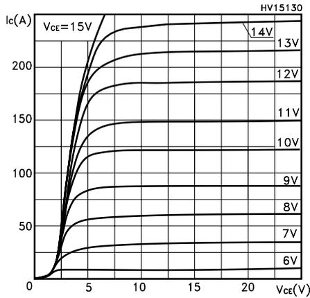
Figure 2. Transfer Characteristics
