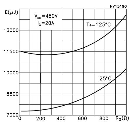
Figure 11. Switching Losses vs Temperature
