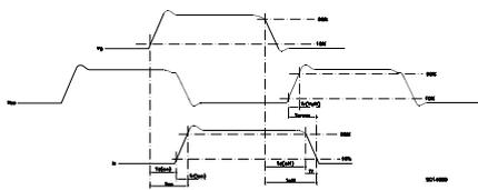
Figure 19. Diode Recovery Time Waveform
