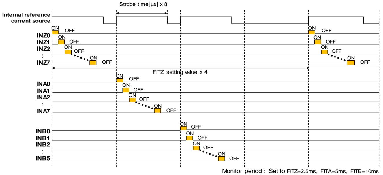
Figure 16. Sequential Monitoring of All Switches Pins Example
