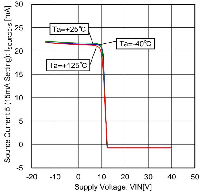
Figure 66. Source Current 5 vs Voltage Characteristic (15mA Setting)
