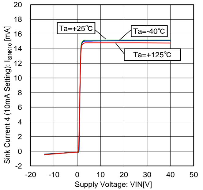
Figure 62. Sink Current 4 vs Voltage Characteristic (10mA Setting)
