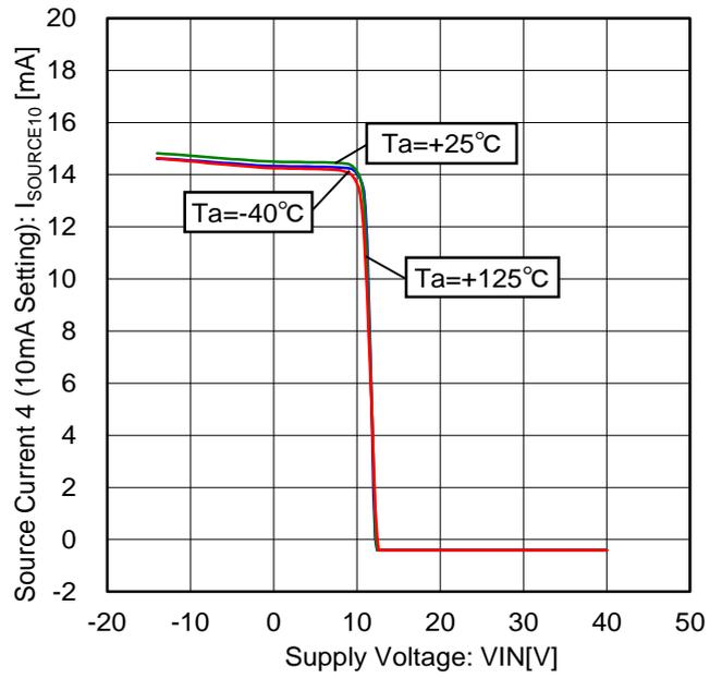
Figure 58. Source Current 4 vs Voltage Characteristic (10mA Setting)
