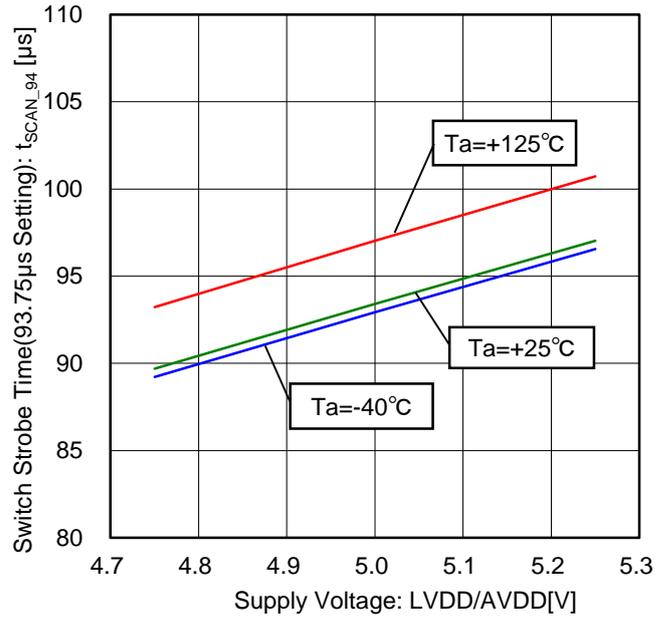
Figure 110. Switch Strobe Time vs Voltage Characteristic (93.75µs Setting)
