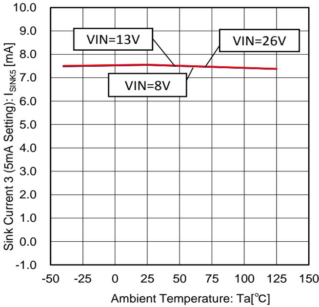
Figure 53. Sink Current 3 vs Temperature Characteristic (5mA Setting)
