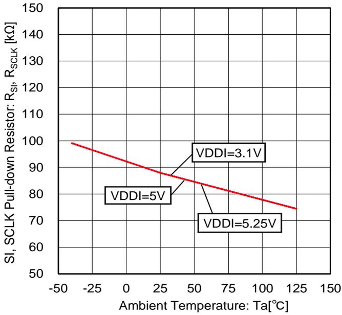
Figure 85. SI, SCLK Pull-down Resistor vs Temperature Characteristic
