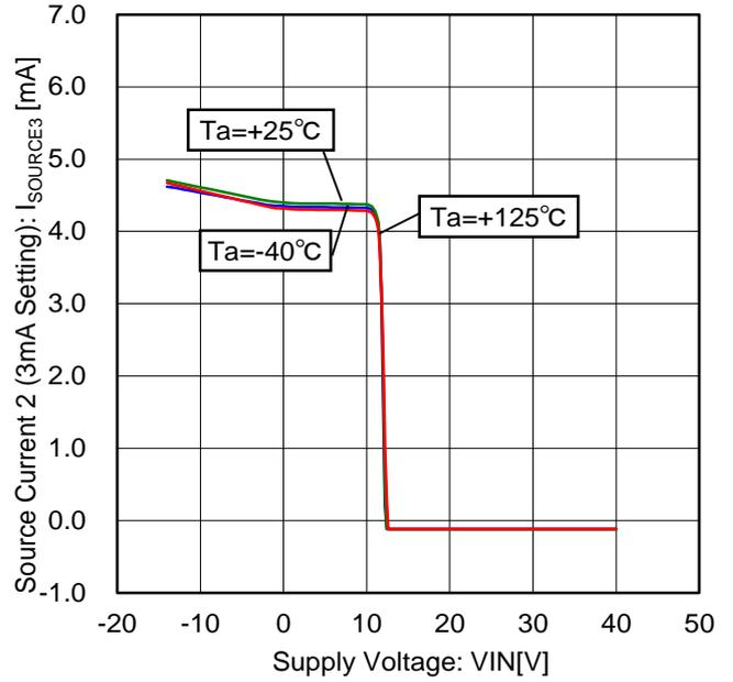
Figure 42. Source Current 2 vs Voltage Characteristic (3mA Setting)
