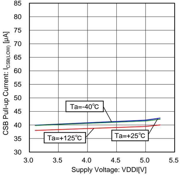
Figure 84. CSB Pull-up Current vs Voltage Characteristic (CSB=0V)
