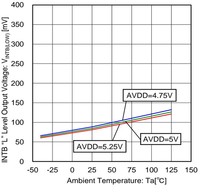
Figure 103. INTB "L" Level Output Voltage vs Temperature Characteristic (I<sub>SINK</sub>=1.0mA)
