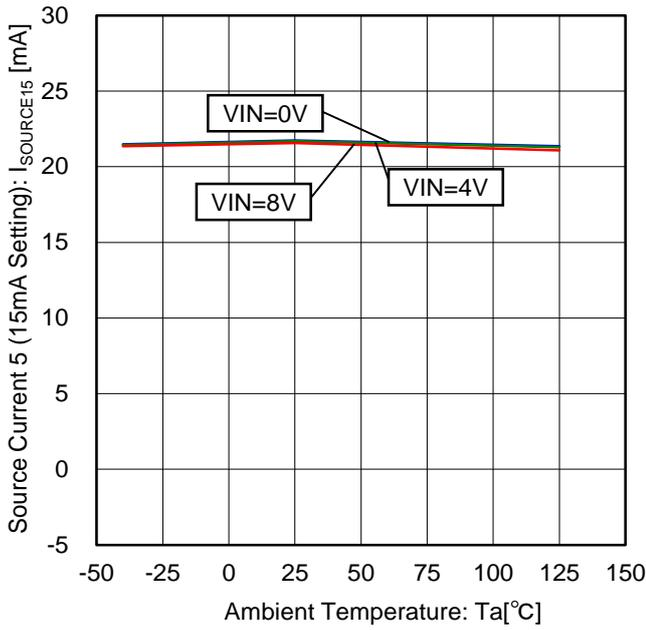
Figure 65. Source Current 5 vs Temperature Characteristic (15mA Setting)
