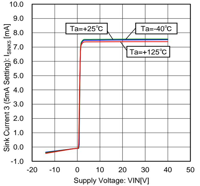
Figure 54. Sink Current 3 vs Voltage Characteristic (5mA Setting)
