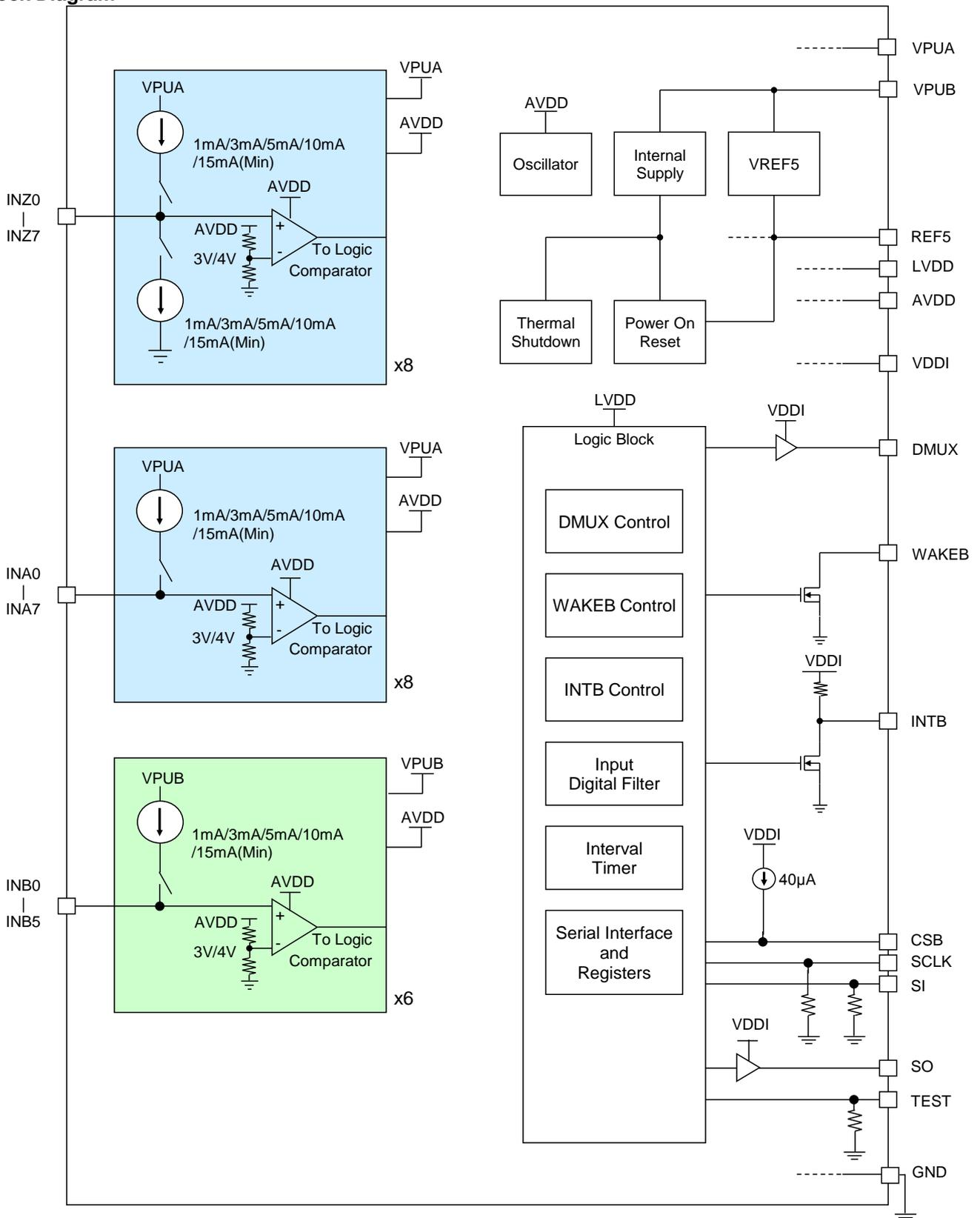
Figure 3. Block Diagram
