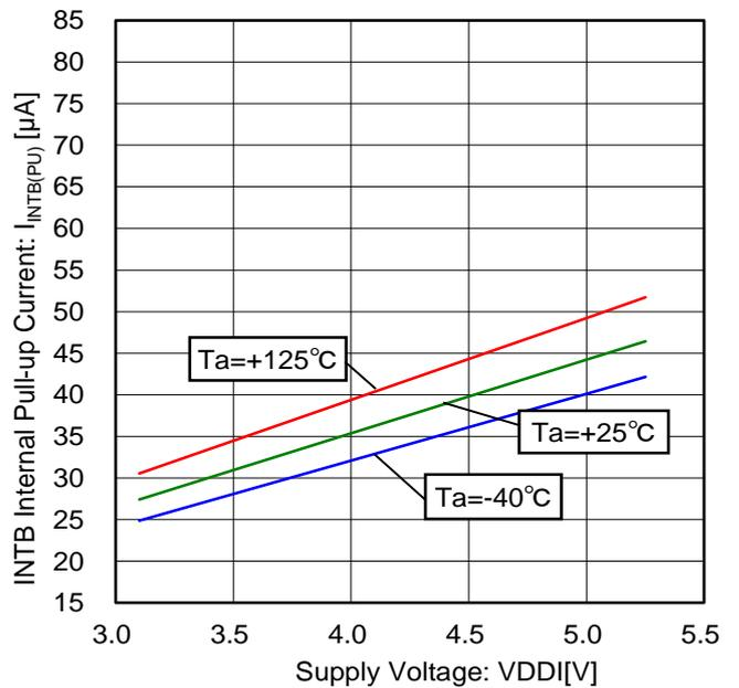
Figure 100. INTB Internal Pull-up Current vs Voltage Characteristic
