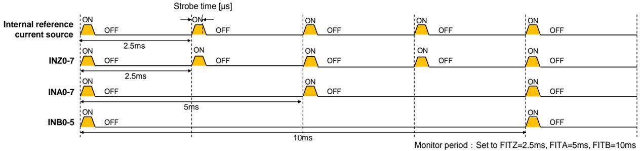
Figure 14. Intermittent Monitoring at the Same Time Example
