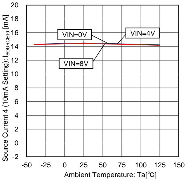
Figure 57. Source Current 4 vs Temperature Characteristic (10mA Setting)
