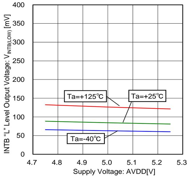
Figure 104. INTB "L" Level Output Voltage vs Voltage Characteristic (I<sub>SINK</sub>=1.0mA)
