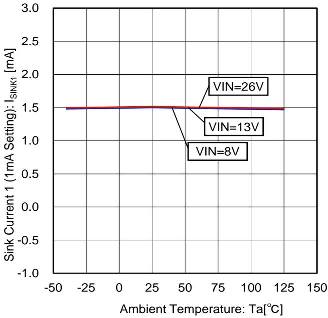
Figure 37. Sink Current 1 vs Temperature Characteristic (1mA Setting)
