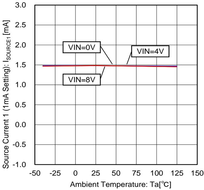
Figure 33. Source Current 1 vs Temperature Characteristic (1mA Setting)
