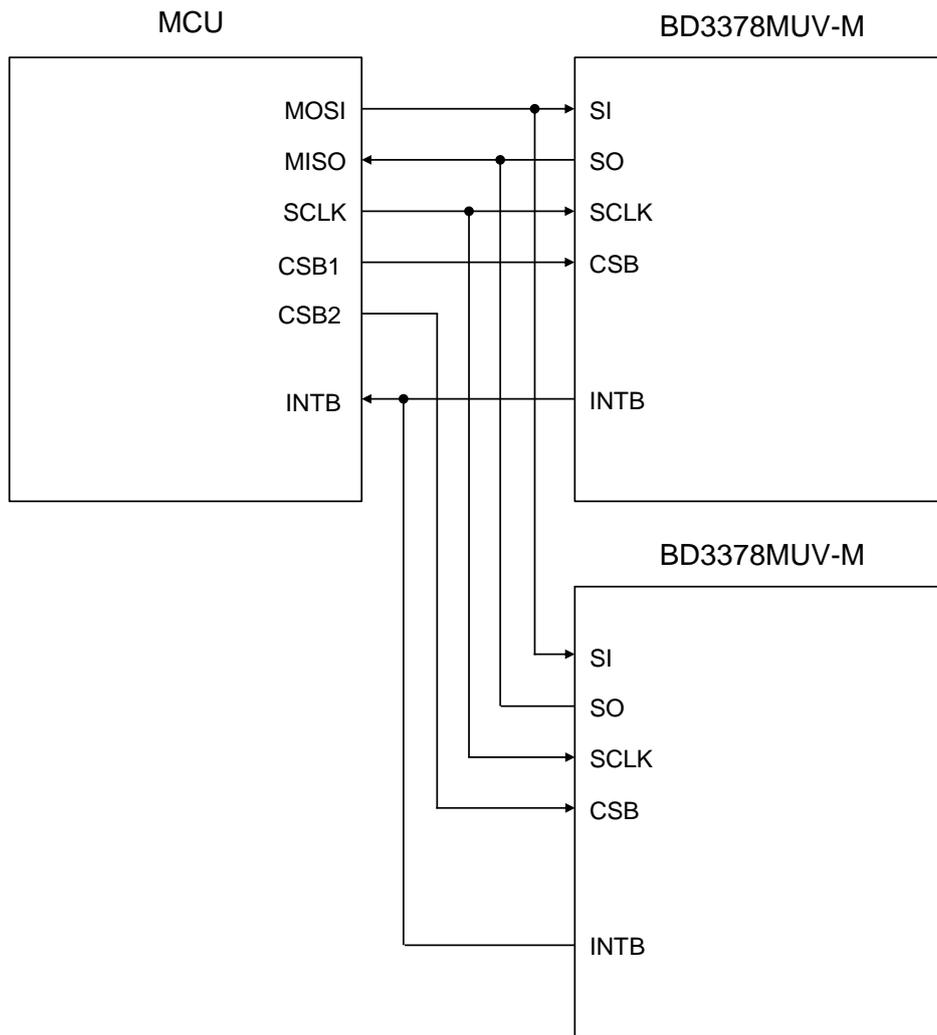
Figure 122. Example of Parallel Connection Circuit
