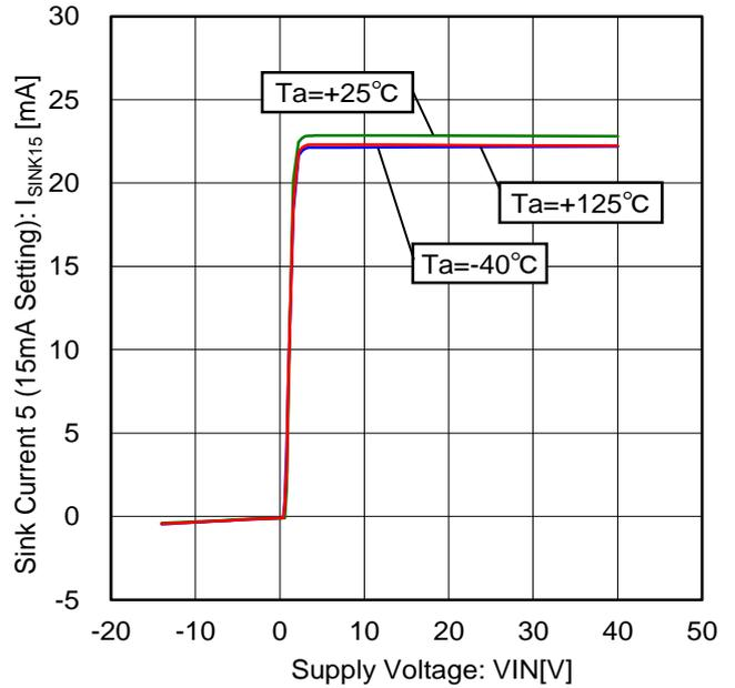
Figure 70. Sink Current 5 vs Voltage Characteristic (15mA Setting)
