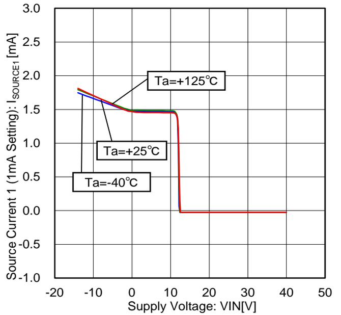
Figure 34. Source Current 1 vs Voltage Characteristic (1mA Setting)
