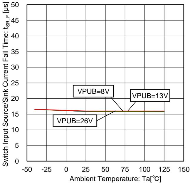
Figure 119. Switch Input Source/Sink Current Fall Time vs Temperature Characteristic (FSQ="0", FSQZ/A/B="0", 10mA Setting, Load Resistance=100 $\Omega$ )
