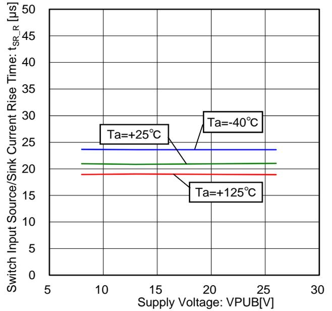
Figure 118. Switch Input Source/Sink Current Rise Time vs Voltage Characteristic (FSQ="0", FSQZ/A/B="0", 10mA Setting, Load Resistance=100 $\Omega$ )
