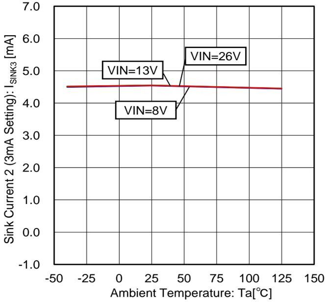
Figure 45. Sink Current 2 vs Temperature Characteristic (3mA Setting)
