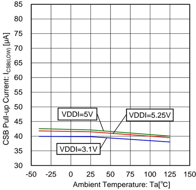
Figure 83. CSB Pull-up Current vs Temperature Characteristic (CSB=0V)
