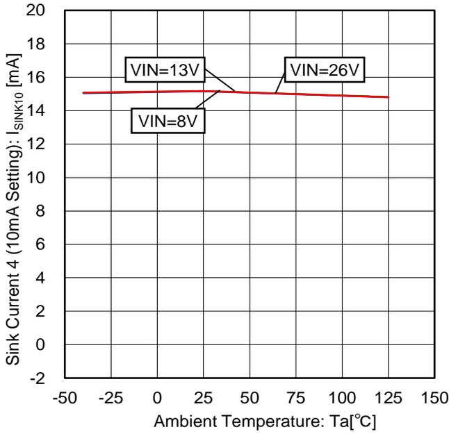
Figure 61. Sink Current 4 vs Temperature Characteristic (10mA Setting)
