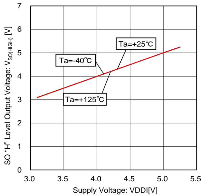
Figure 90. SO "H" Level Output Voltage vs Voltage Characteristic ( $I_{SOURCE}=200\mu A$ )
