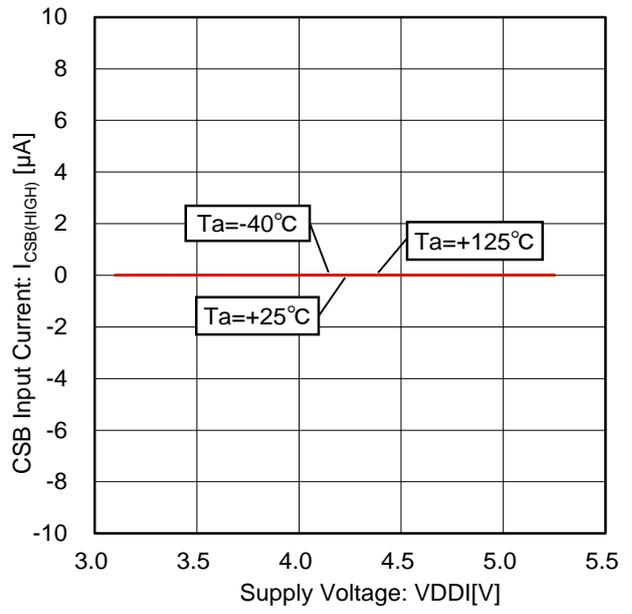
Figure 82. CSB Input Current vs Voltage Characteristic (CSB=VDDI)
