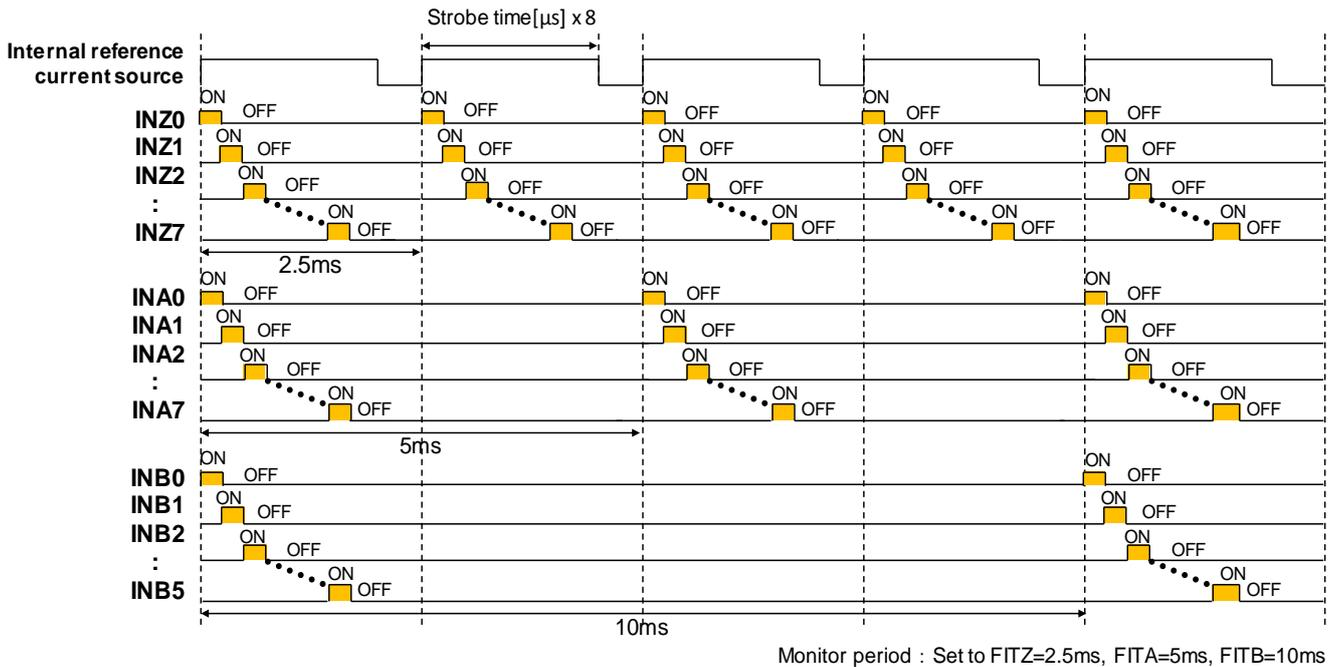
Figure 15. Sequential Monitoring by Power Supply System Example
