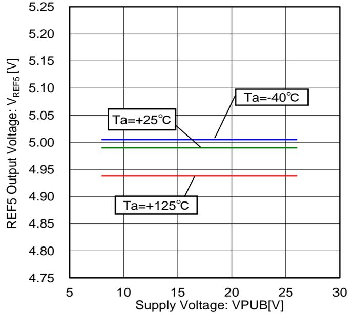
Figure 30. REF5 Output Voltage vs Voltage Characteristic
