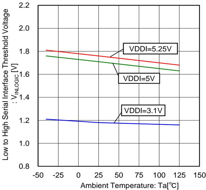
Figure 79. Low to High Serial Interface Threshold Voltage vs Temperature Characteristic
