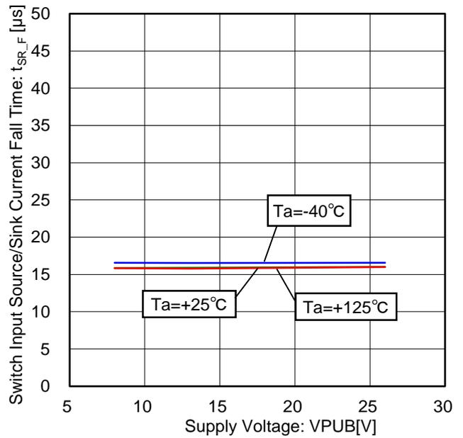
Figure 120. Switch Input Source/Sink Current Fall Time vs Voltage Characteristic (FSQ="0", FSQZ/A/B="0", 10mA Setting, Load Resistance=100 $\Omega$ )
