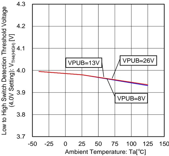
Figure 75. Low to High Switch Detection Threshold Voltage vs Temperature Characteristic (4.0V Setting)
