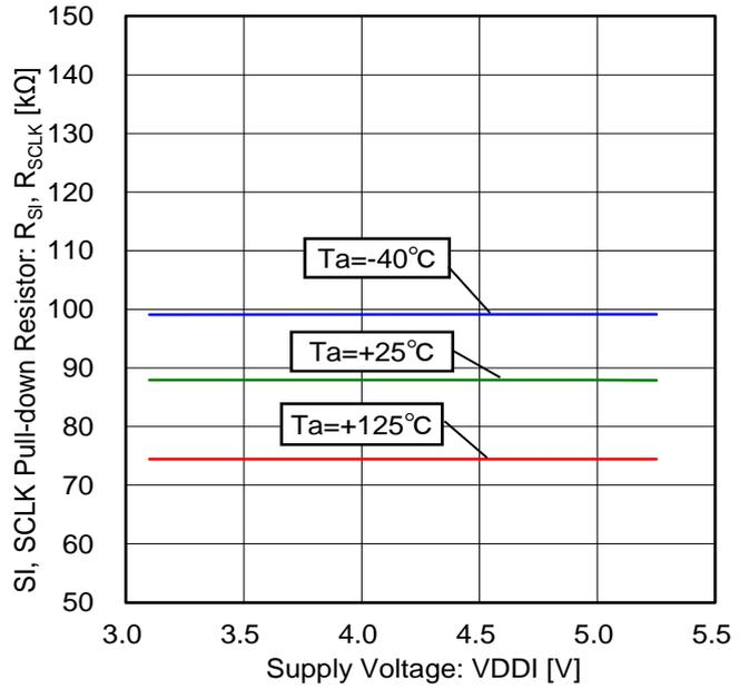
Figure 86. SI, SCLK Pull-down Resistor vs Voltage Characteristic
