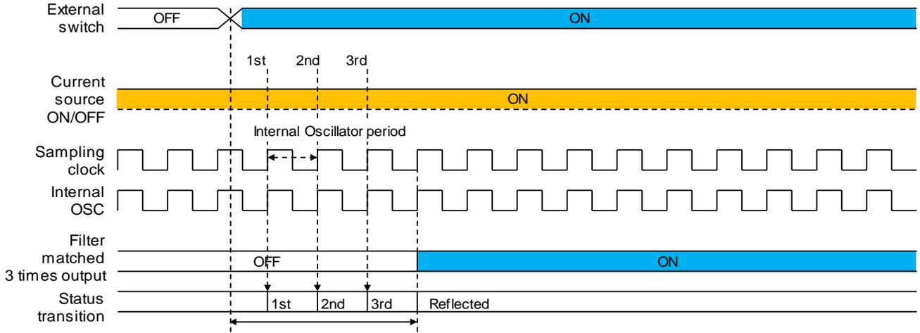
Time from Monitoring to End of Filtering:
