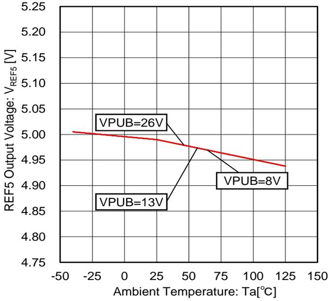
Figure 29. REF5 Output Voltage vs Temperature Characteristic
