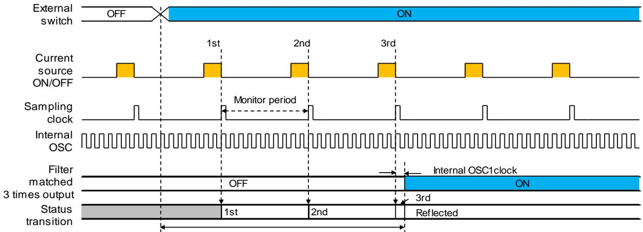
Time from Monitoring to End of Filtering:
