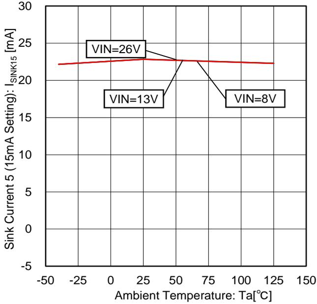
Figure 69. Sink Current 5 vs Temperature Characteristic (15mA Setting)
