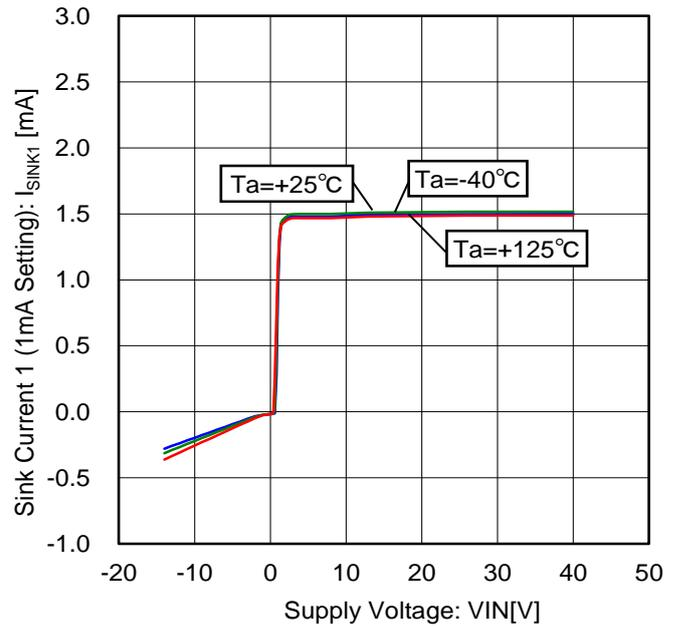
Figure 38. Sink Current 1 vs Voltage Characteristic (1mA Setting)
