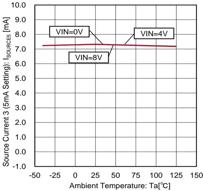
Figure 49. Source Current 3 vs Temperature Characteristic (5mA Setting)
