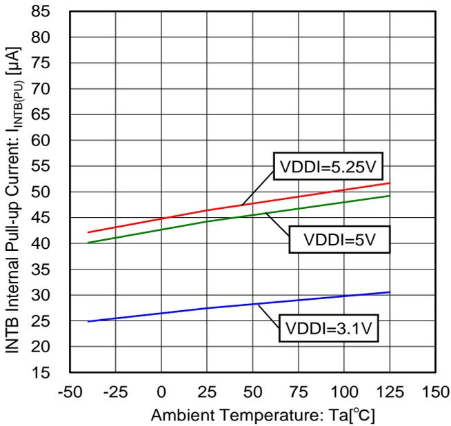
Figure 99. INTB Internal Pull-up Current vs Temperature Characteristic
