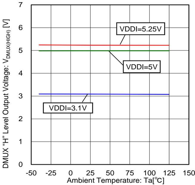
Figure 95. DMUX "H" Level Output Voltage vs Temperature Characteristic (I<sub>SOURCE</sub>=200μA)
