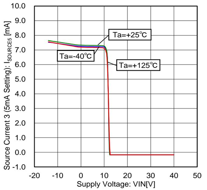
Figure 50. Source Current 3 vs Voltage Characteristic (5mA Setting)
