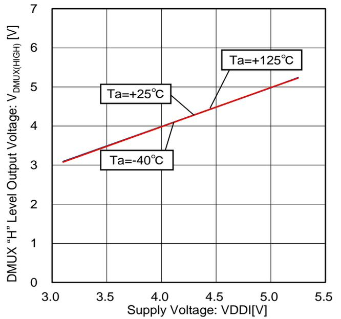
Figure 96. DMUX "H" Level Output Voltage vs Voltage Characteristic (I<sub>SOURCE</sub>=200μA)
