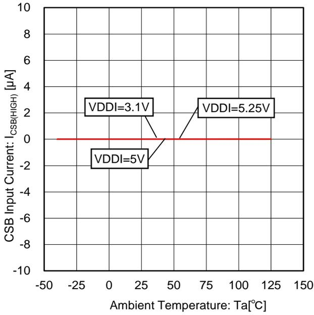
Figure 81. CSB Input Current vs Temperature Characteristic (CSB=VDDI)
