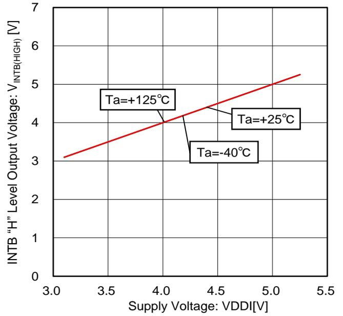
Figure 102. INTB "H" Level Output Voltage vs Voltage Characteristic (INTB=OPEN)
