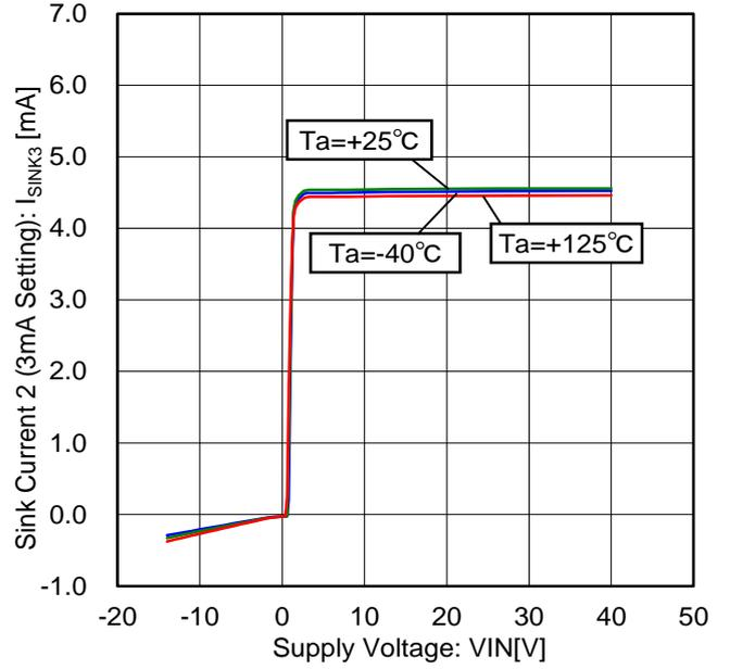
Figure 46. Sink Current 2 vs Voltage Characteristic (3mA Setting)
