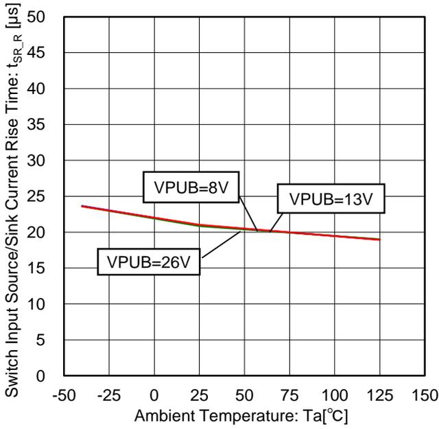
Figure 117. Switch Input Source/Sink Current Rise Time vs Temperature Characteristic (FSQ="0", FSQZ/A/B="0", 10mA Setting, Load Resistance=100 $\Omega$ )
