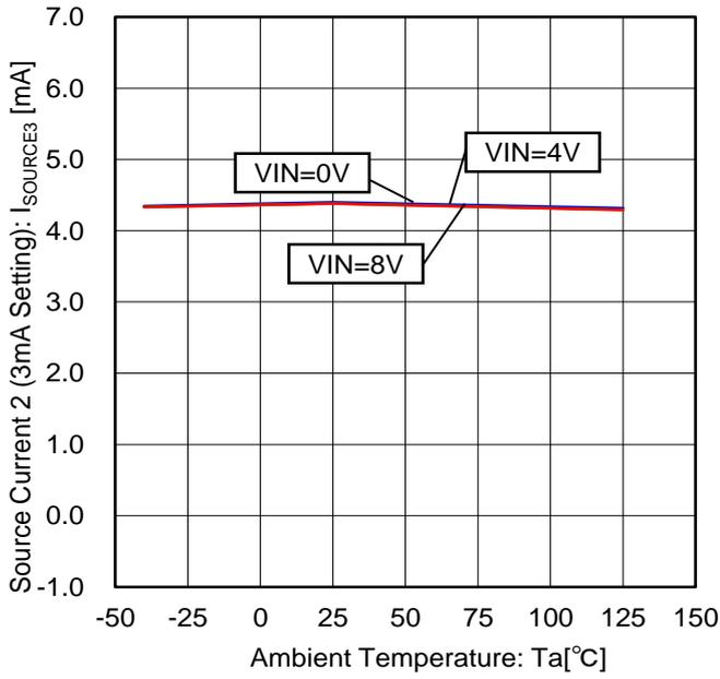
Figure 41. Source Current 2 vs Temperature Characteristic (3mA Setting)
