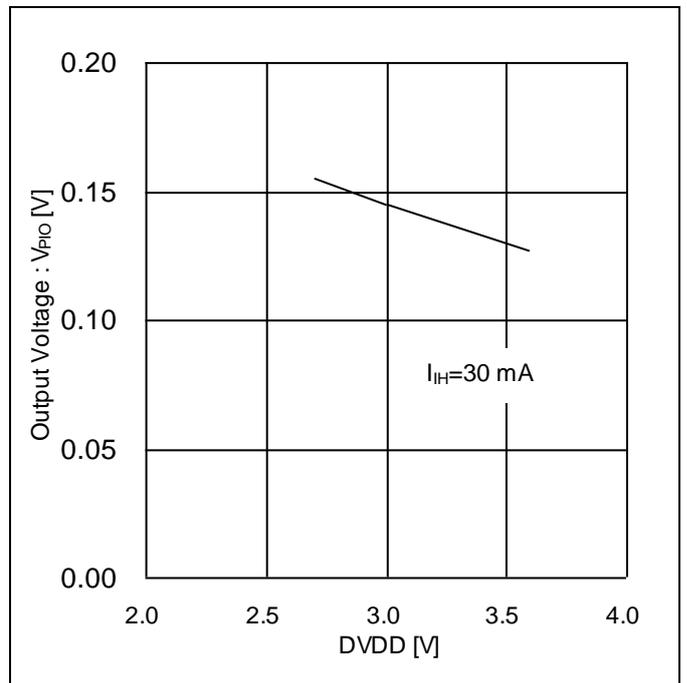
Figure 8. Output Voltage vs DVDD (PI Driver Circuit)
