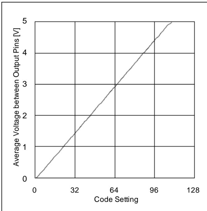
Figure 7. Average Voltage between Output Pins vs Code Setting (Voltage Driver Block)
