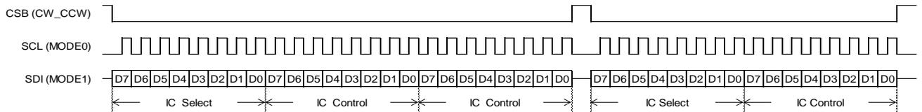
Figure 4. 3-wire Serial Communication Input Waveform
