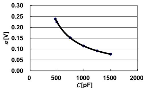
Figure 1. CR Coefficient for Calculation of Discharge Time
