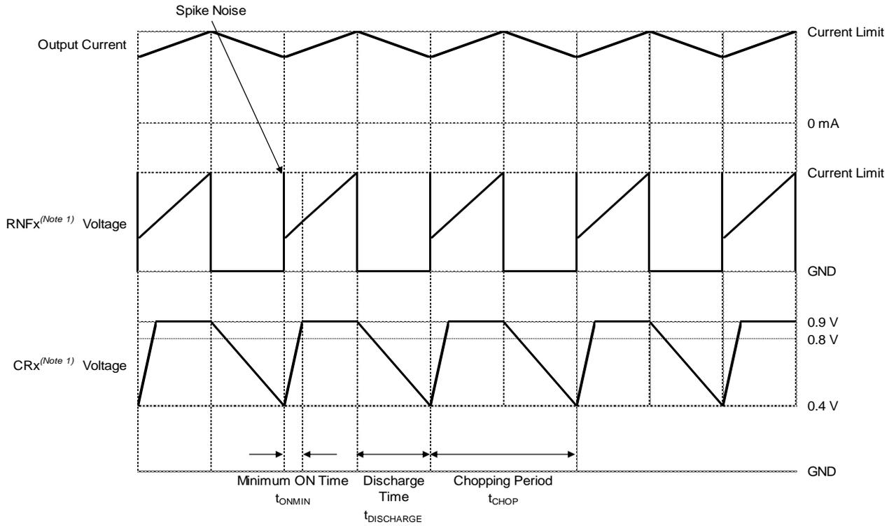
Figure 2. Timing Chart of CRx Voltage, RNFx Voltage and Output Current
