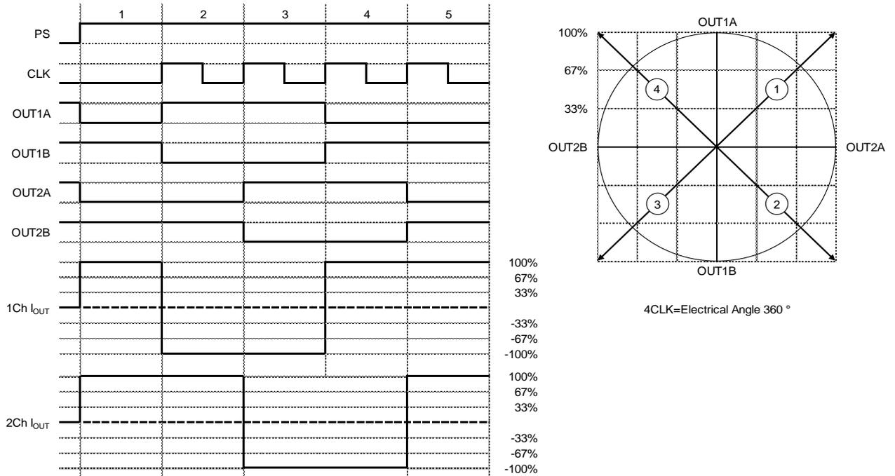
4 HALF STEP A (MODE0 = H, MODE1 = L, CW\_CCW = L, ENABLE = H)
