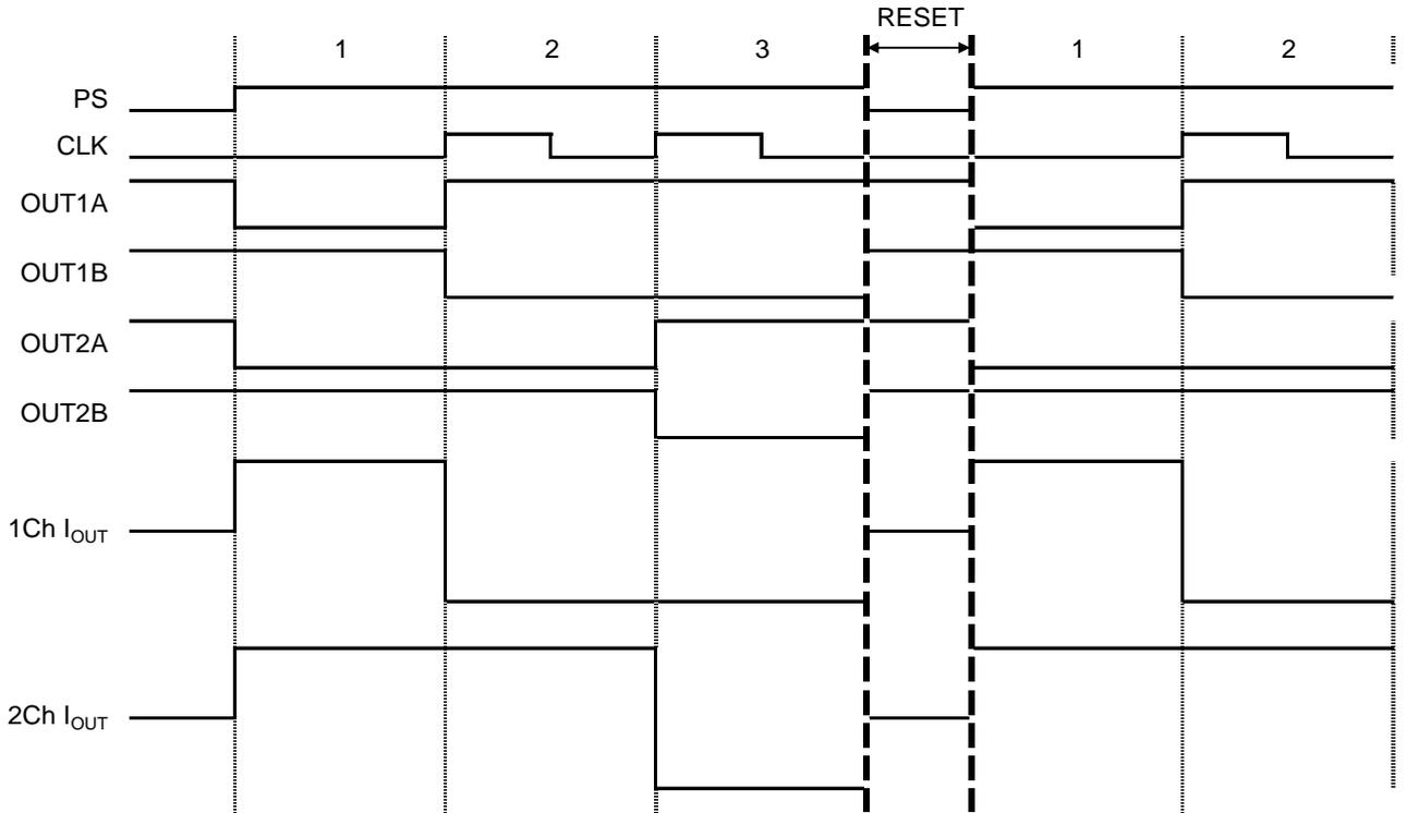
**8 CW\_CCW Switch Timing Chart (FULL STEP, MODE0 = L, MODE1 = L, ENABLE = H)**
