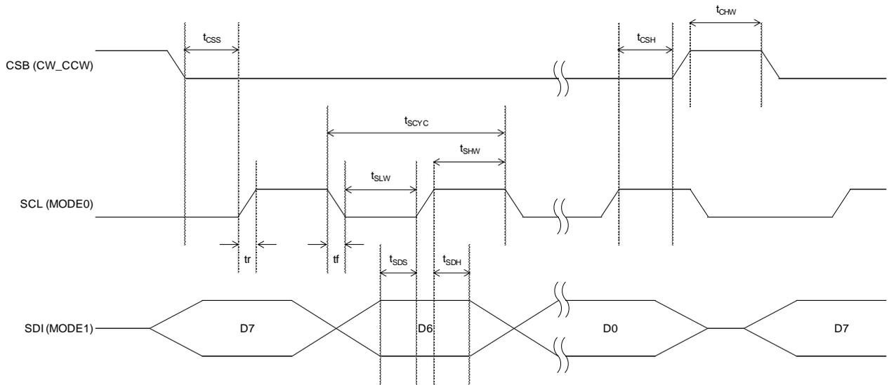
Figure 5. Input Timing
