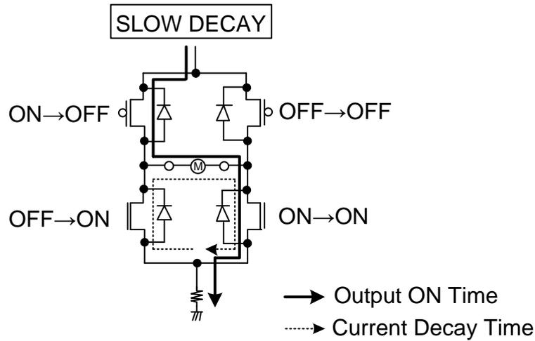
Figure 2. Route of Regenerated Current during Current Decay
