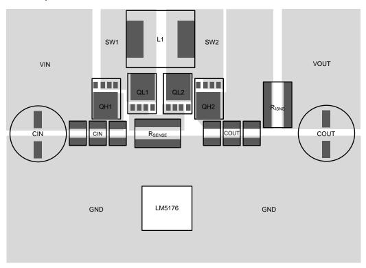
Figure 30. LM5176-Q1 Power Stage Layout
