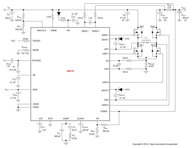
Figure 25. LM5176-Q1 Four-Switch Buck Boost Application Schematic
