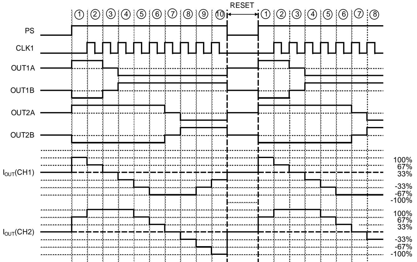
CW CCW Switch Timing Chart (FULL STEP, MODE01=L, MODE11=L, ENABLE1=H)
