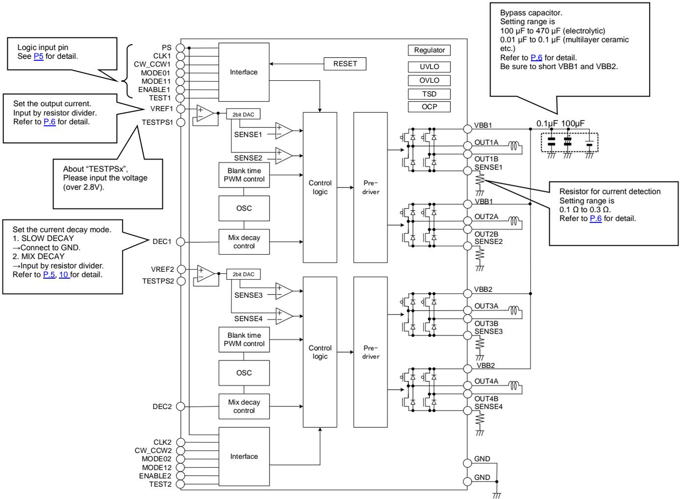
Figure 8. BD63888AEKV Block Diagram and Applied Circuit Diagram
