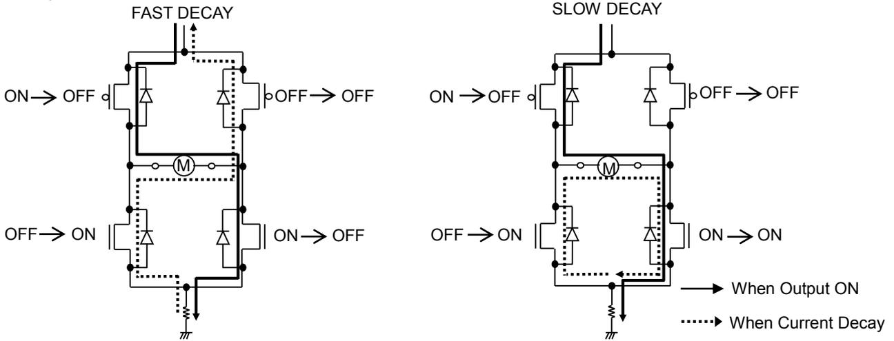
Figure 5. Route of Regenerated Current during Current Decay
