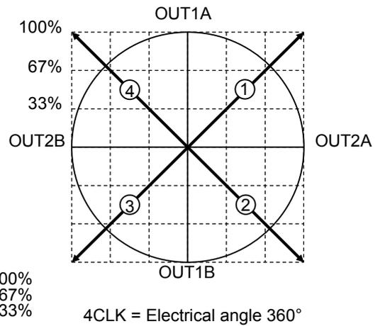
HALF STEP A (MODE01=H, MODE11=L, CW CCW1=L, ENABLE1=H)
