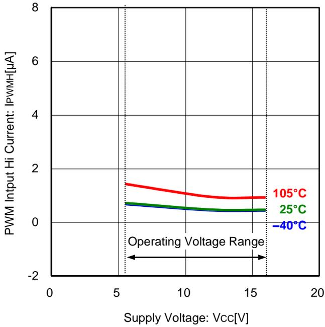
Figure 15. PWM Input Hi Current vs Supply Voltage
