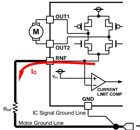
Figure 42. Setting of current limit and ground lines
