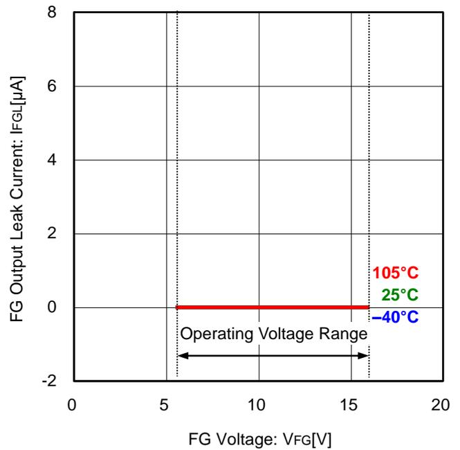
Figure 14. FG Output Leak Current vs FG Voltage
