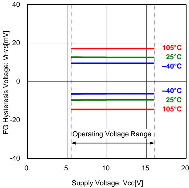
Figure 11. FG Hysteresis Voltage vs Supply Voltage
