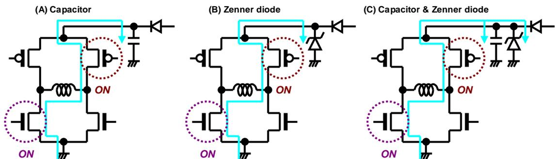
Figure 52. Measure against V<sub>CC</sub> and Motor Driving Outputs Voltage
