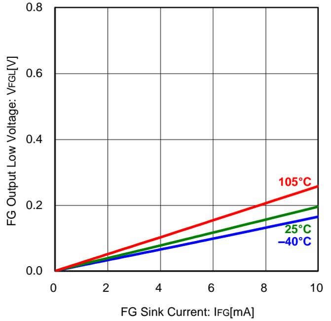
Figure 12. FG Output Low Voltage vs FG Sink Current (Vcc=12V)
