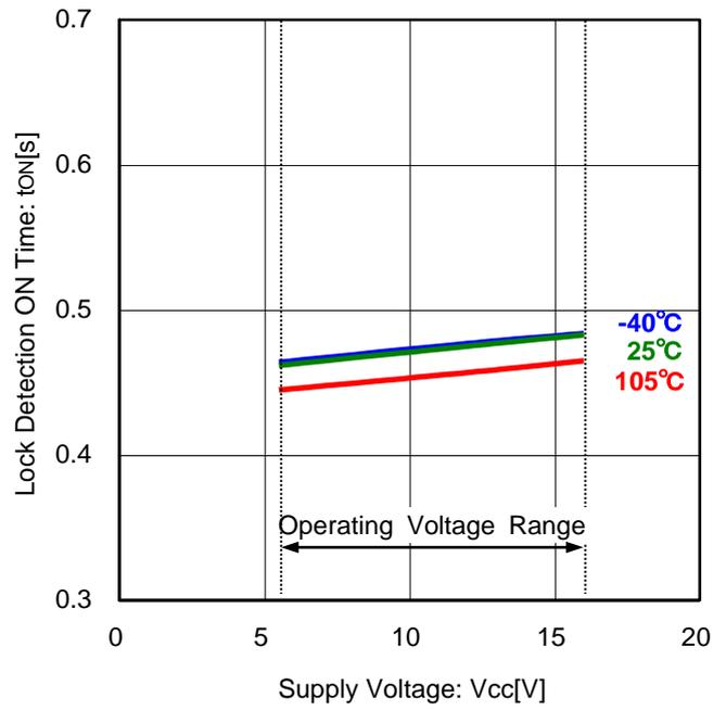
Figure 8. Lock Detection ON Time vs Supply Voltage
