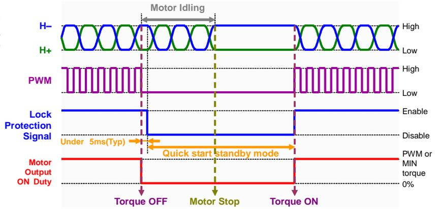
Figure 44. Quick Start Timing Chart (PWM Input Application)
