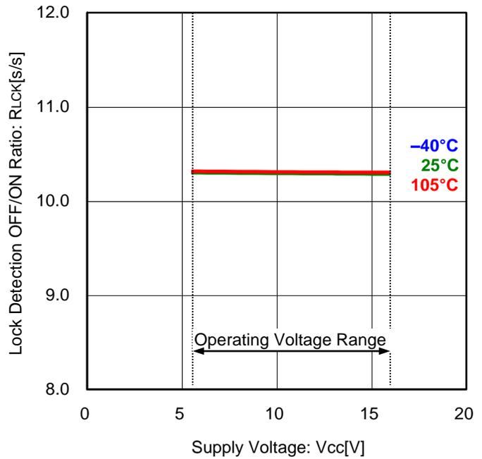
Figure 10. Lock Detection OFF/ON Ratio vs Supply Voltage
