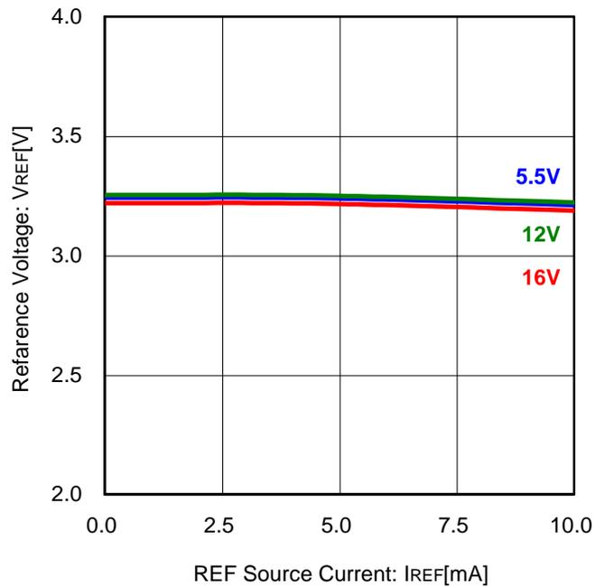
Figure 18. Reference Voltage vs REF Source Current (Ta=25°C)
