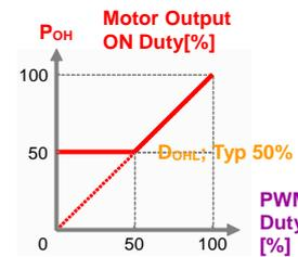
Figure 45. I/O Duty Characteristic in Start Duty Assist
