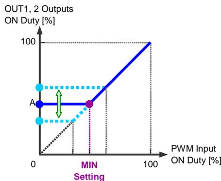
Figure 24. Setting of Minimum Output Duty
