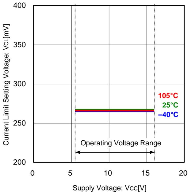
Figure 19. Current Limit Setting Voltage vs Supply Voltage
