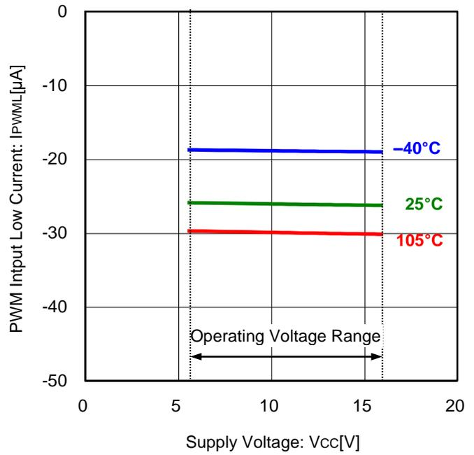
Figure 16. PWM Input Low Current vs Supply Voltage
