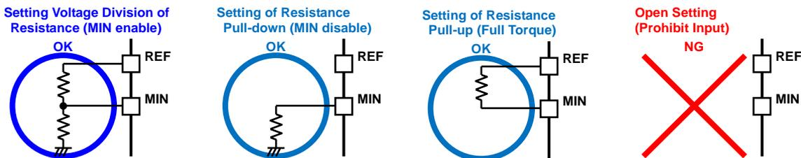
Figure 26. MIN Terminal Setting
