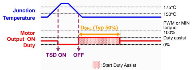
Figure 47. Timing Chart of TSD Release
