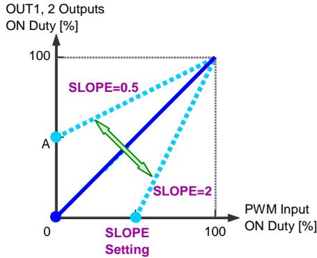
Figure 27. Adjust of Slope of I/O Duty
