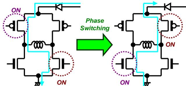
Figure 51. V<sub>CC</sub> Voltage Rise by Back Electromotive Force
