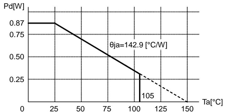
(Note) Reduce by 7.0mW/°C when operating over Ta=25°C (Mounted on 70.0mm x 70.0mm x 1.6mm glass epoxy board)
