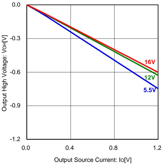
Figure 5. Output High Voltage vs Output Source Current
