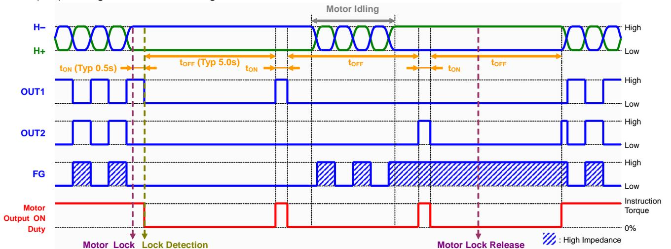
Figure 43. Lock Protection (Incorporated Counter System) Timing Chart
