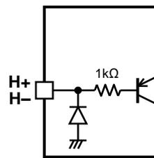
4. I/O duty slope setting terminal, Minimum output duty setting terminal, Recirculate period setting terminal and Soft switching setting terminal
