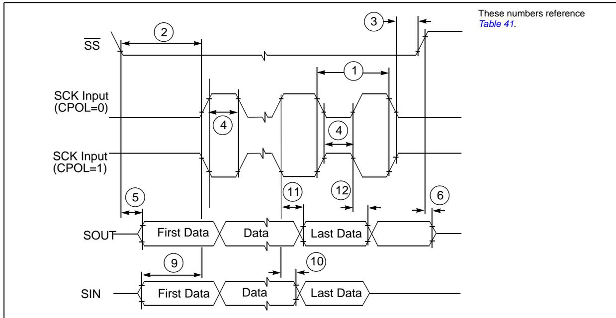
Figure 24. DSPI modified transfer format timing – slave, CPHA = 1
