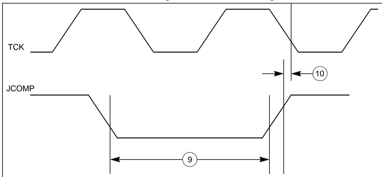
Figure 9. JTAG boundary scan timing
