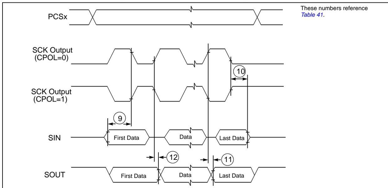
Figure 19. DSPI classic SPI timing – slave, CPHA = 0
