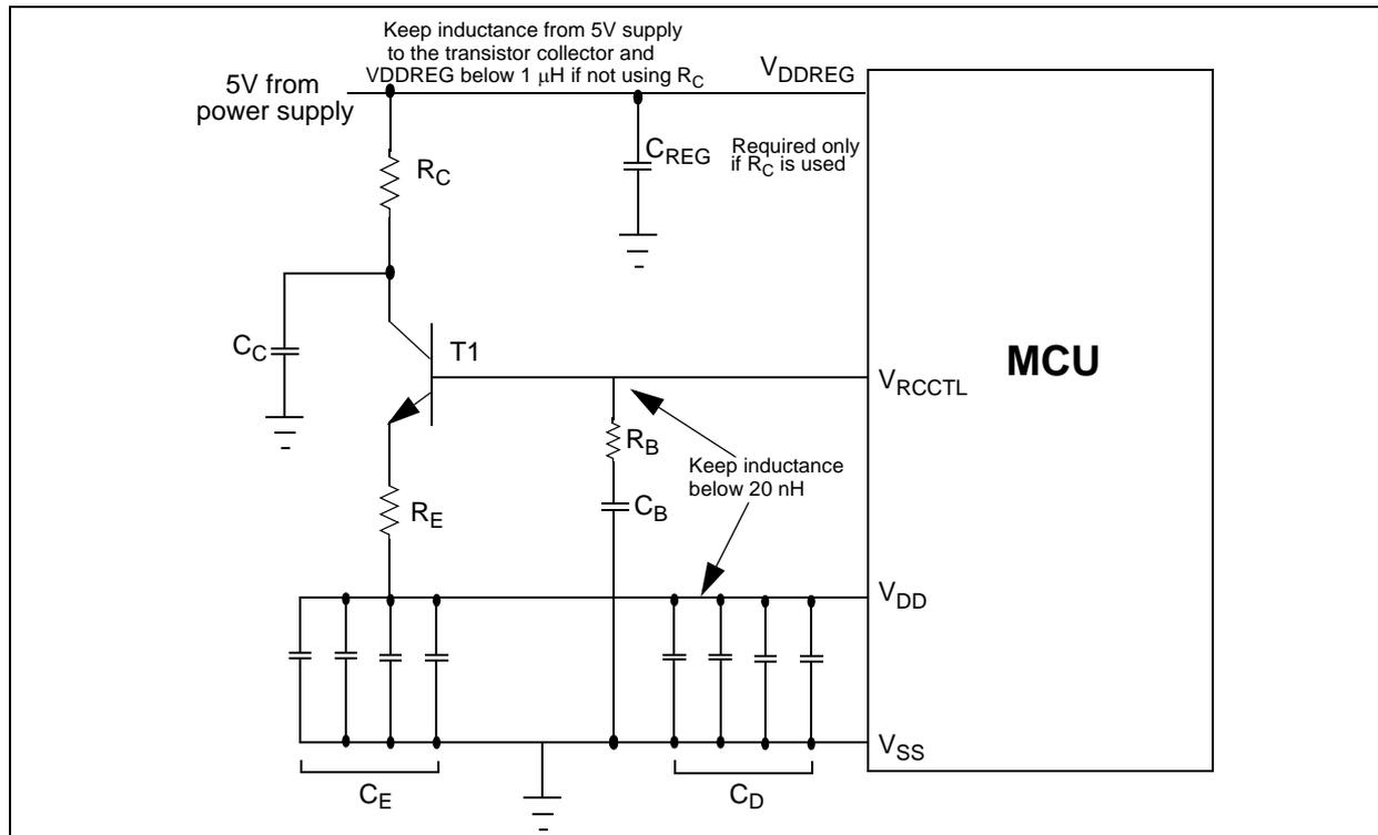
There are three options for the bypassing and compensation networks for the 1.2V regulator controller. The component values in the following table are the same for all PMC network requirements.
