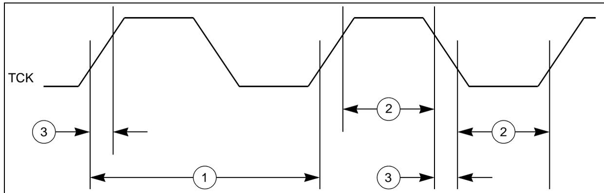
Figure 7. JTAG test access port timing
