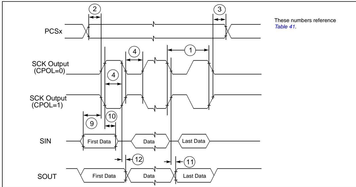
Figure 18. DSPI classic SPI timing – master, CPHA = 1
