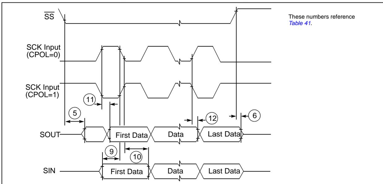
Figure 21. DSPI modified transfer format timing – master, CPHA = 0
