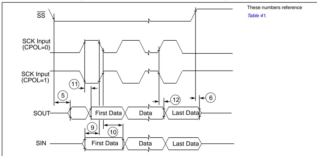
Figure 25. DSPI PCS strobe ( $\overline{PCSS}$ ) timing
