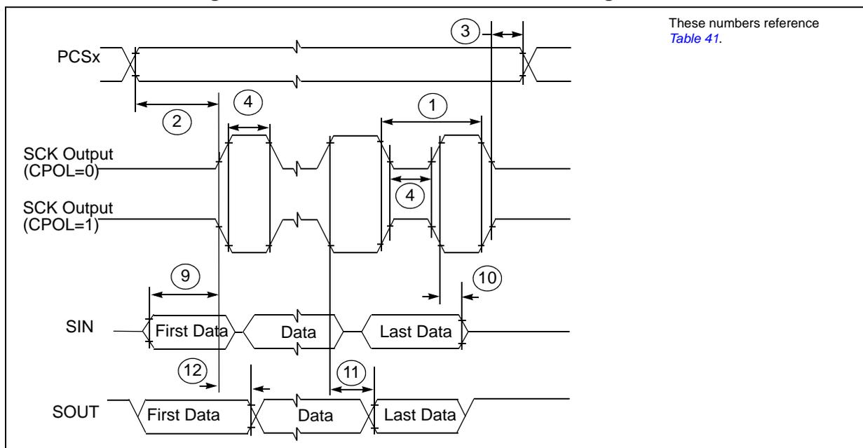
Figure 22. DSPI modified transfer format timing – master, CPHA = 1
