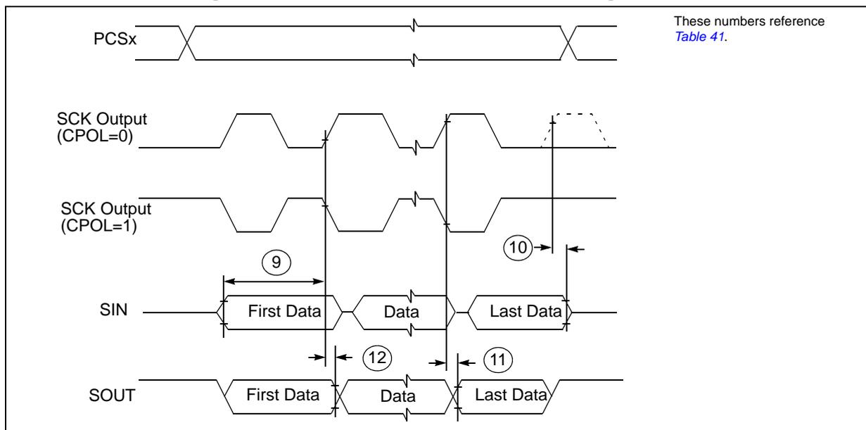
Figure 23. DSPI modified transfer format timing – slave, CPHA = 0
