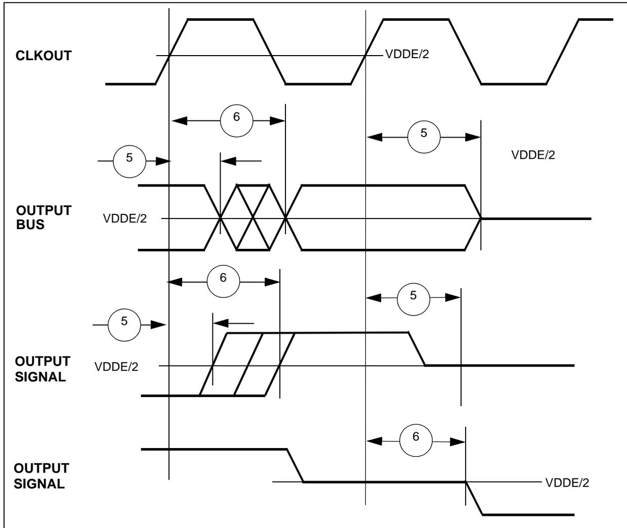
Figure 15. Synchronous input timing
