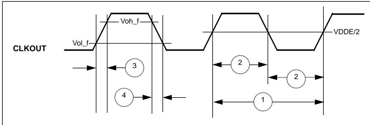
Figure 14. Synchronous output timing
