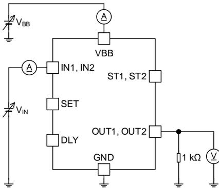
Figure 26. UVLO Detection Voltage
