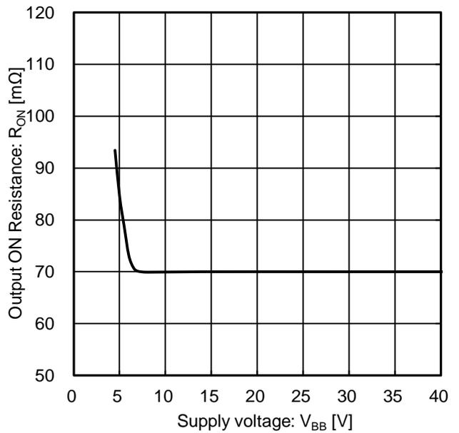
Figure 13. Output ON Resistance vs Supply Voltage
