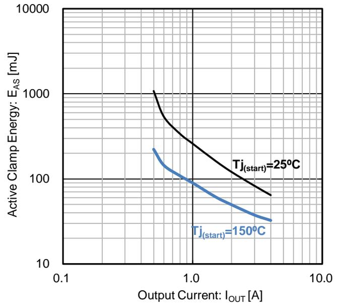
Figure 23. Active Clamp Energy vs Output Current
