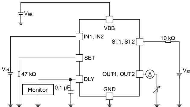
Figure 30. Fixed Over Current Limit
