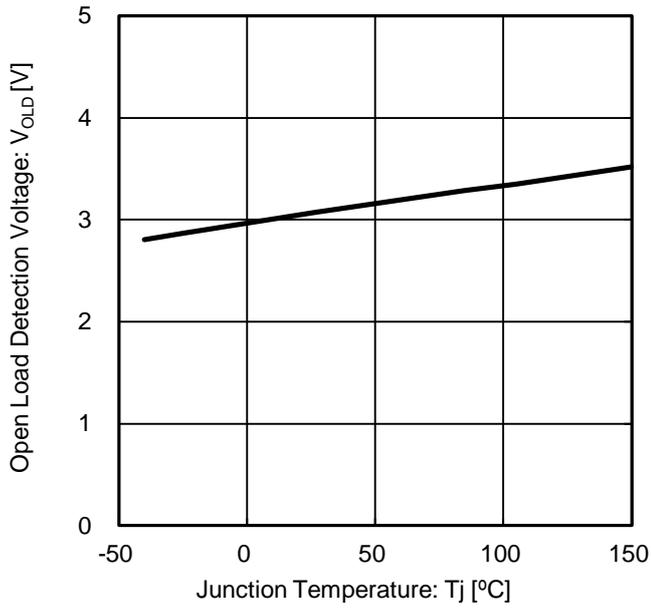
Figure 22. Open Load Detection Voltage vs Junction Temperature
