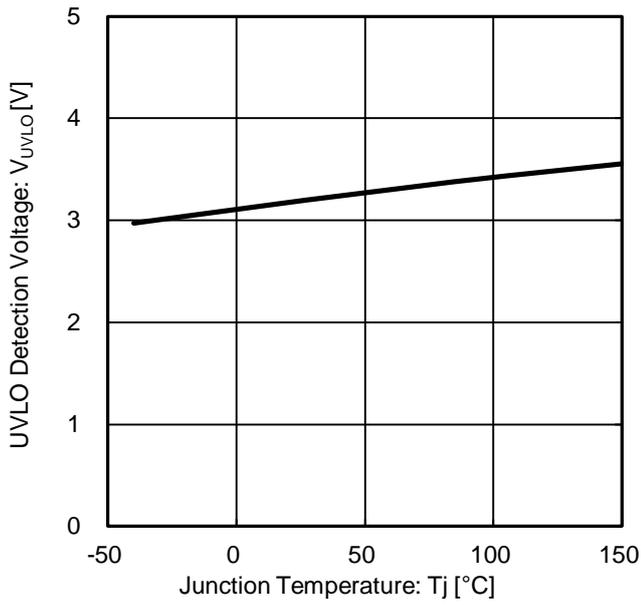
Figure 10. UVLO Detection Voltage vs Junction Temperature
