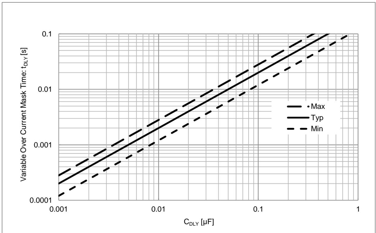
Figure 37. Variable Over Current Mask Time vs  $C_{DLY}$
