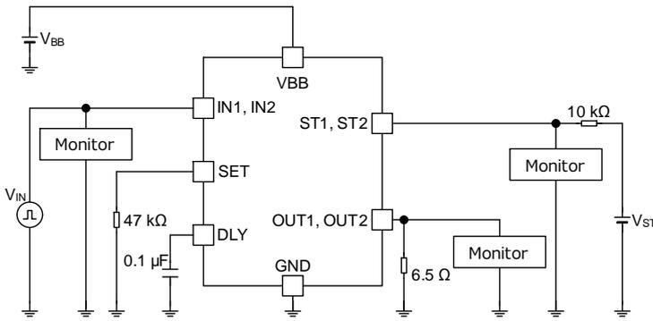
Figure 28. Output ON Slew Rate
