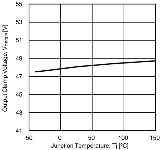
Figure 18. Output Clamp Voltage vs Junction Temperature
