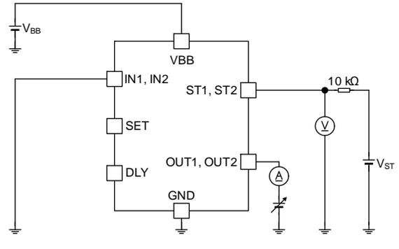
Figure 31. Open Load Detection Voltage
