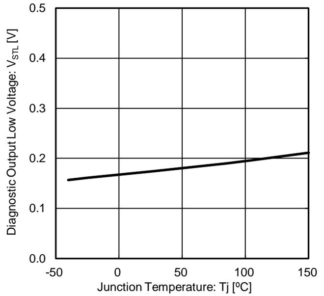
Figure 19. Diagnostic Output Low Voltage vs Junction Temperature
