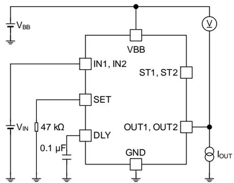
Figure 27. Output ON Resistance
