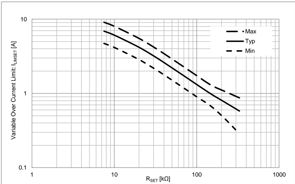
Figure 36. Variable Over Current Limit vs  $R_{SET}$
