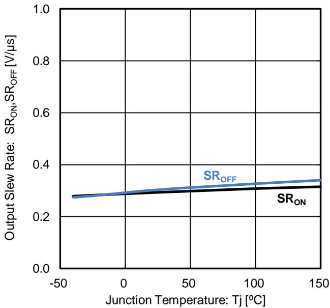
Figure 16. Output Slew Rate vs Junction Temperature
