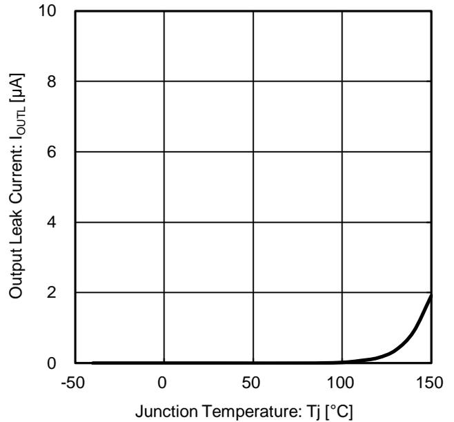
Figure 15. Output leak Current vs Junction Temperature
