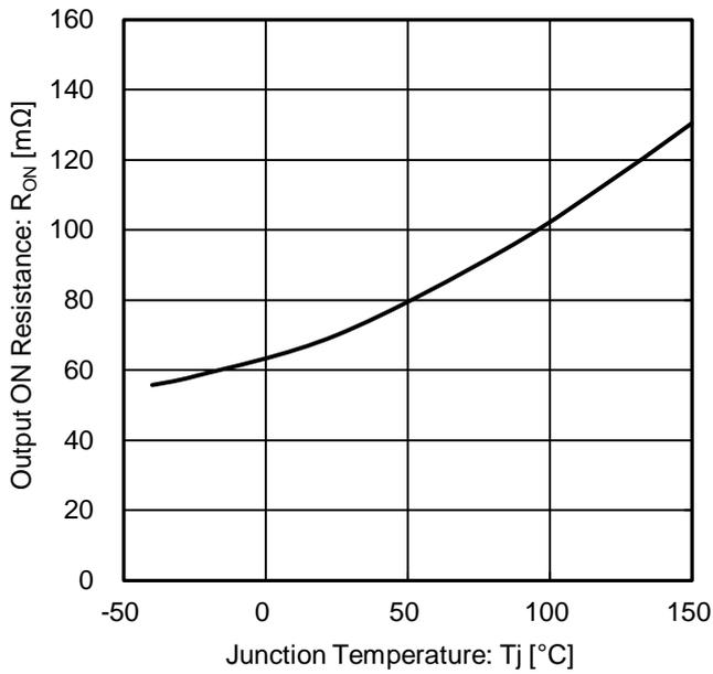
Figure 14. Output ON Resistance vs Junction Temperature
