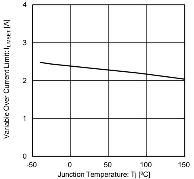
Figure 21. Variable Over Current Limit vs Junction Temperature
