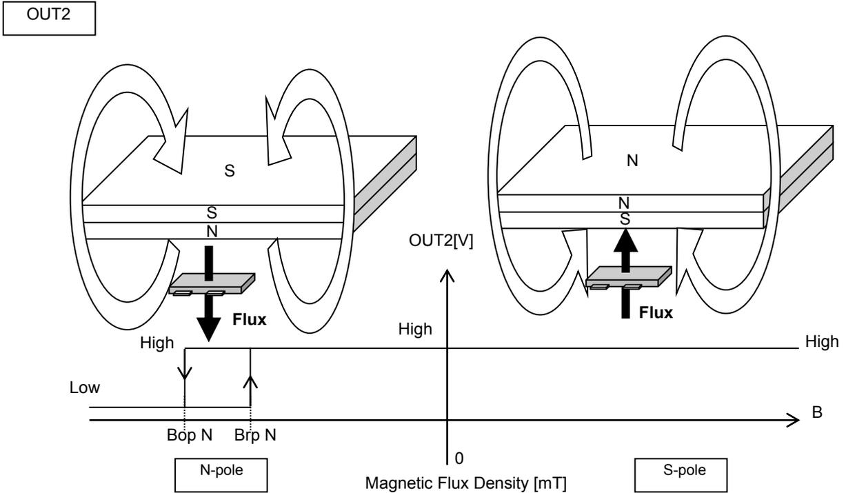
Figure 16. N-pole Detection
