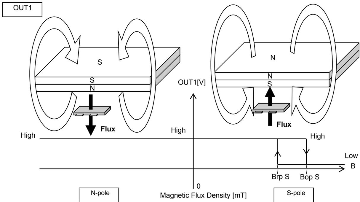
Figure 15. S-pole Detection
