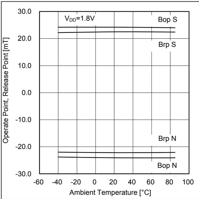
Figure 6. Operate Point, Release Point vs Ambient Temperature
