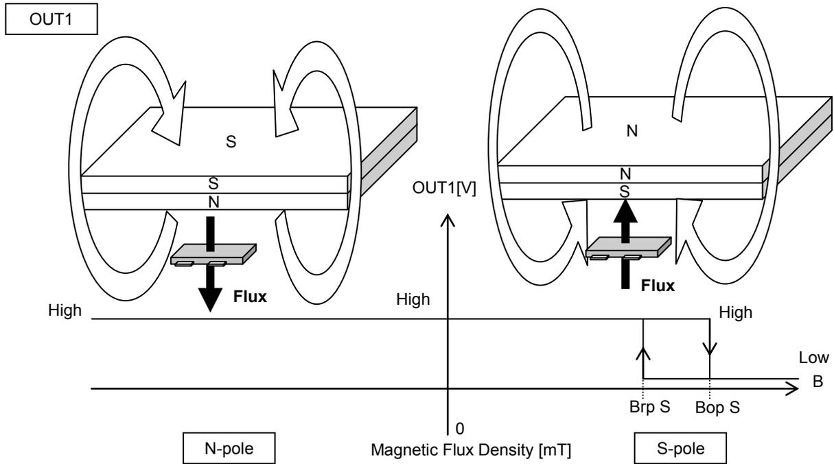
Figure 15. S-pole Detection
