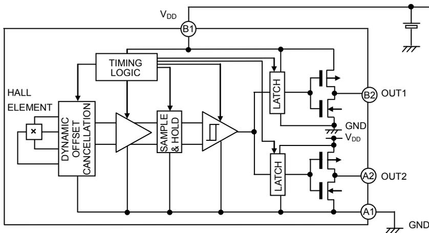
Adjust the bypass capacitor value as necessary, according to voltage noise conditions, etc.
