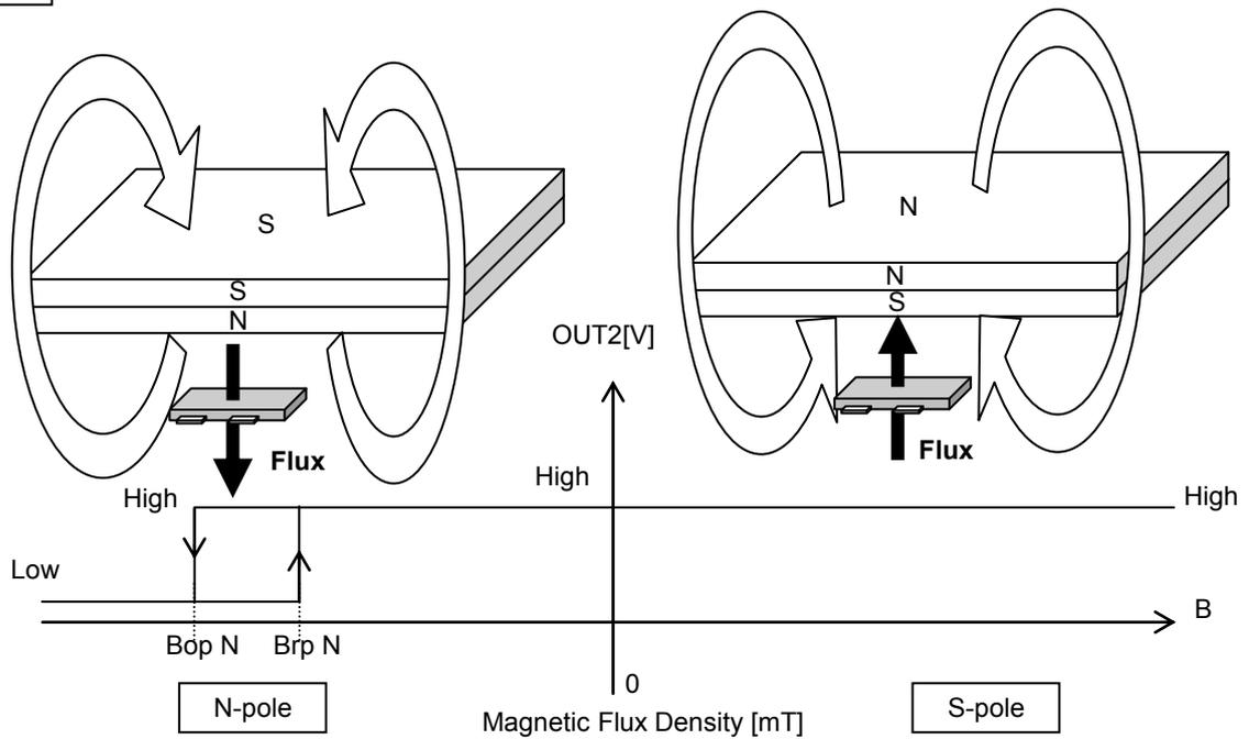
Figure 16. N-pole Detection
