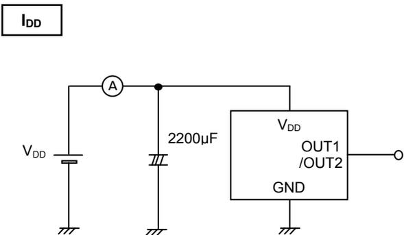
Figure 5.  $I_{DD}$  Measurement Circuit
