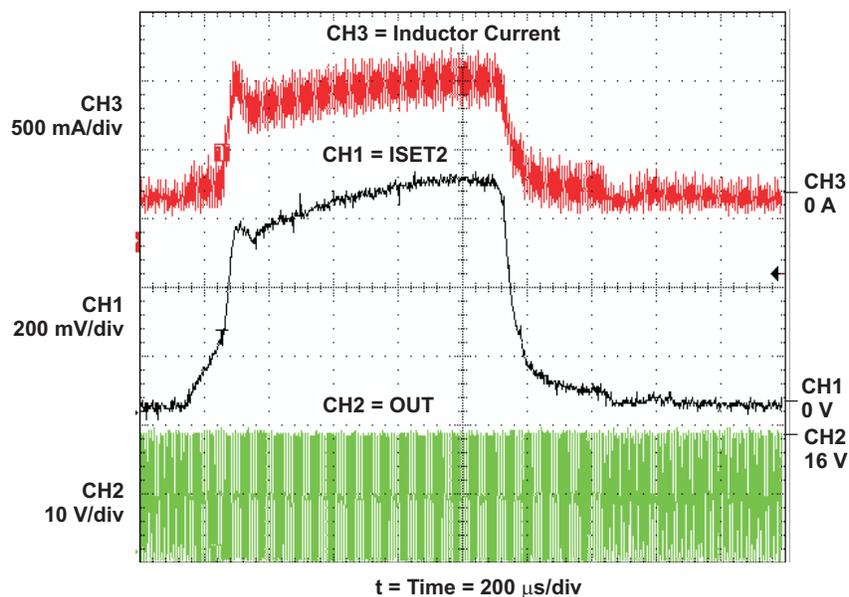
Figure 12. Current Sense Amplifier Charge Current Waveform
