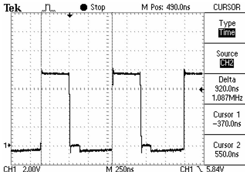
**Precharge:** The current is low in precharge; so, the bottom synchronous FET turns off after its minimum on-time which explains the step between  $\approx 0$  V and  $-0.5$  V. When the bottom FET and top FET are off, the current conducts through the body diode of the bottom FET which results in a diode drop below the ground potential. The initial negative spike is the delay turning on the bottom FET, which is to prevent shoot-through current as the top FET is turning off.
