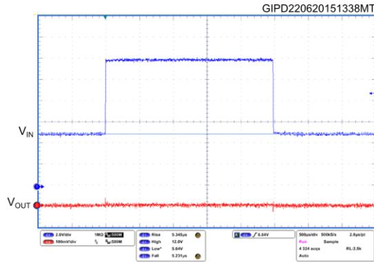
Figure 25: Line transient ( $I_{OUT} = 2\text{ A}$ ,  $V_{OUT} = 2.5\text{ V}$ )
