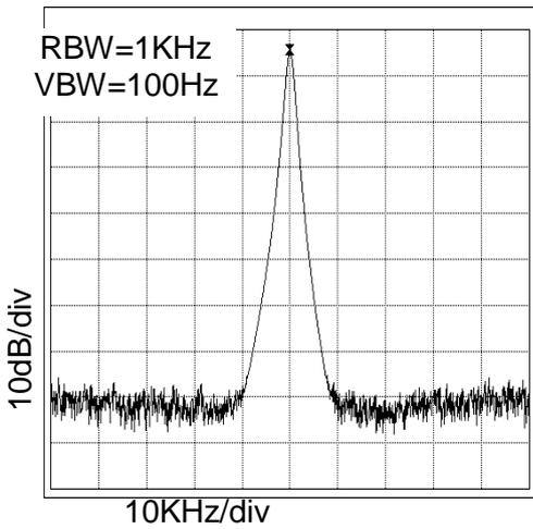
Figure 3. 54MHz Spectrum
