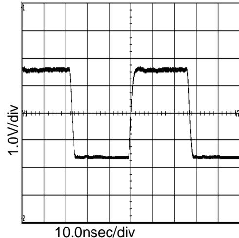
Figure 16. 18.4MHz Output Waveform
