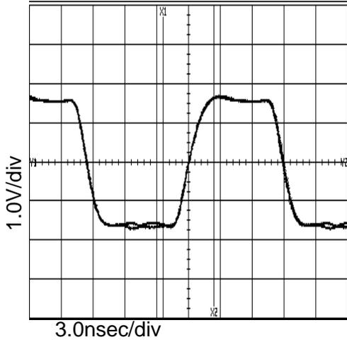
Figure 1. 54MHz Output Waveform
