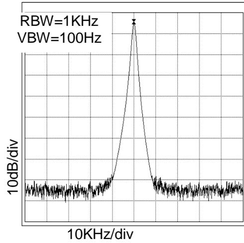
Figure 6. 27MHz Spectrum
