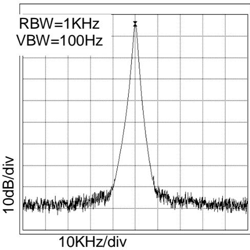
Figure 15. 36.9MHz Spectrum
