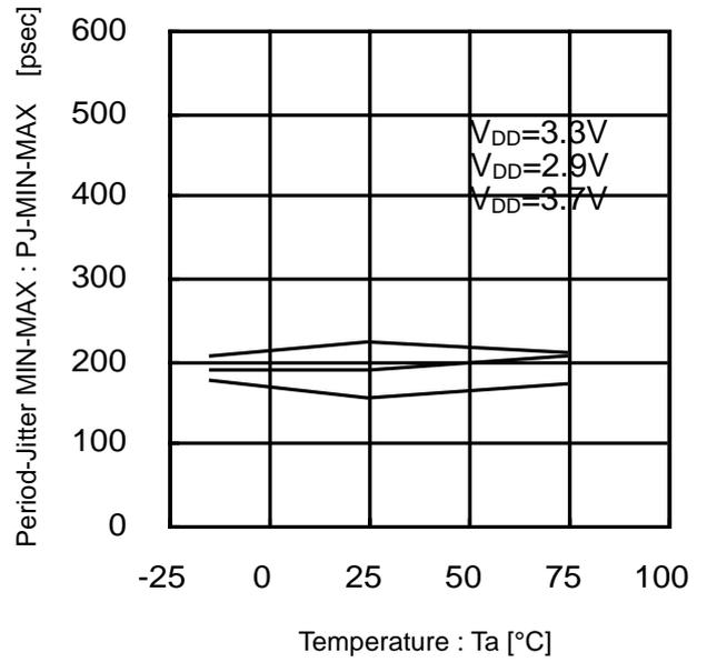
Figure 36. Period-Jitter MIN-MAX vs Temperature (18.4MHz)
