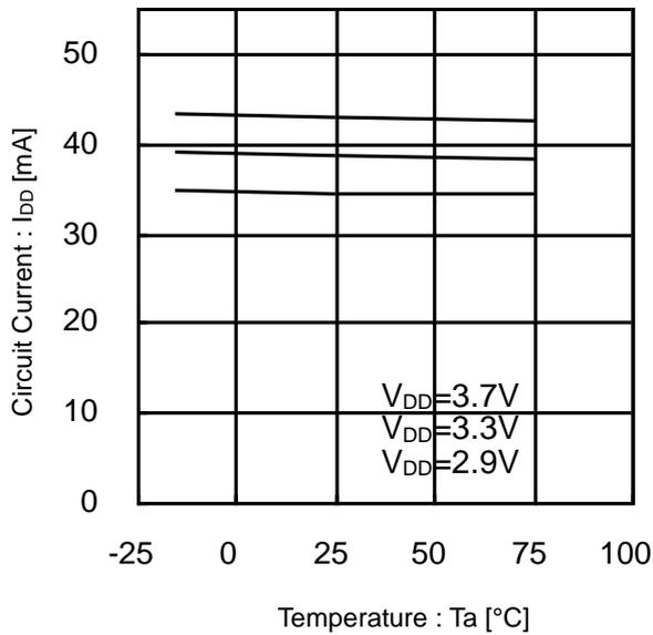
Figure 37. Consumption Current vs Temperature
