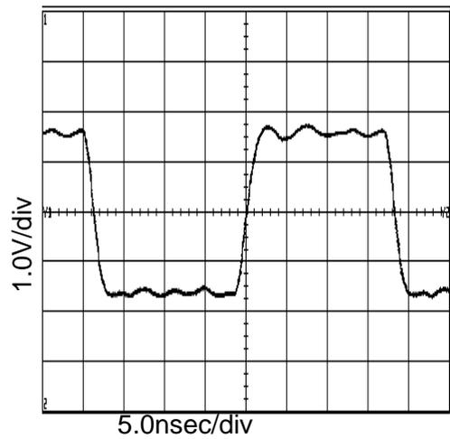
Figure 4. 27MHz Output Waveform
