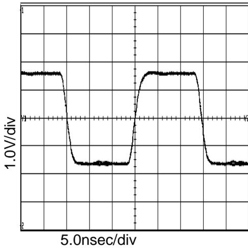
Figure 7. 33.9MHz Output Waveform
