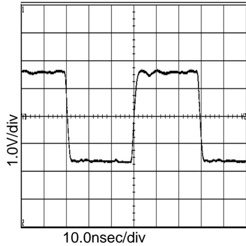
Figure 10. 16.9MHz Output Waveform
