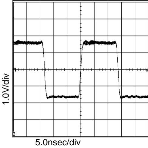
Figure 13. 36.9MHz Output Waveform
