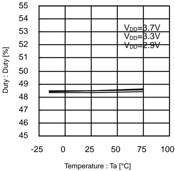
Figure 19. Duty vs Temperature (54MHz)
