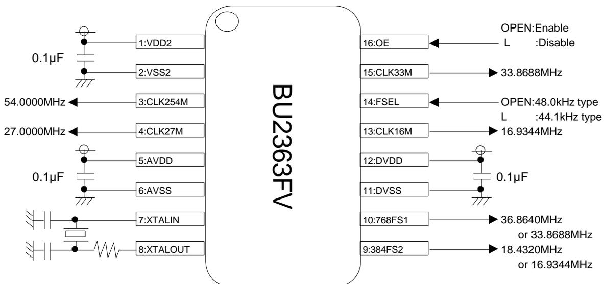
(Note) We believe that this circuit is to be recommended. However, to use it, make further thorough check for the characteristics.
