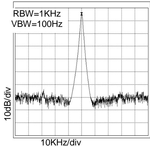
Figure 12. 16.9MHz Spectrum
