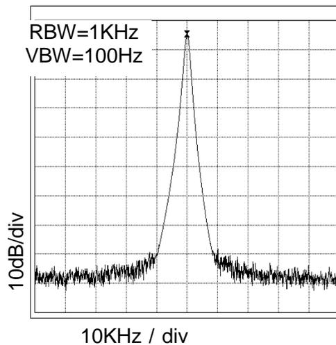
Figure 18. 18.4MHz Spectrum
