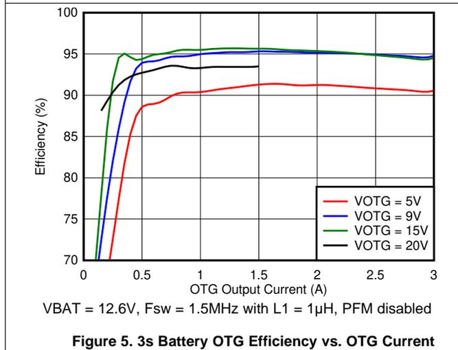
Figure 5. 3s Battery OTG Efficiency vs. OTG Current
