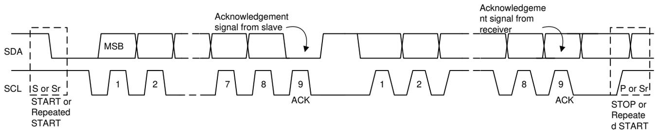
Figure 31. Data Transfer on the I<sup>2</sup>C Bus
