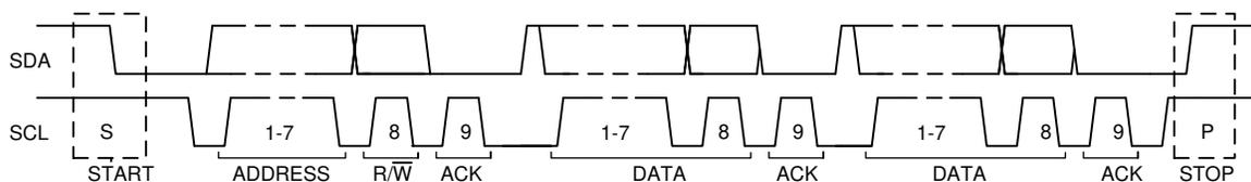
Figure 33. Complete Data Transfer on the I<sup>2</sup>C Bus
