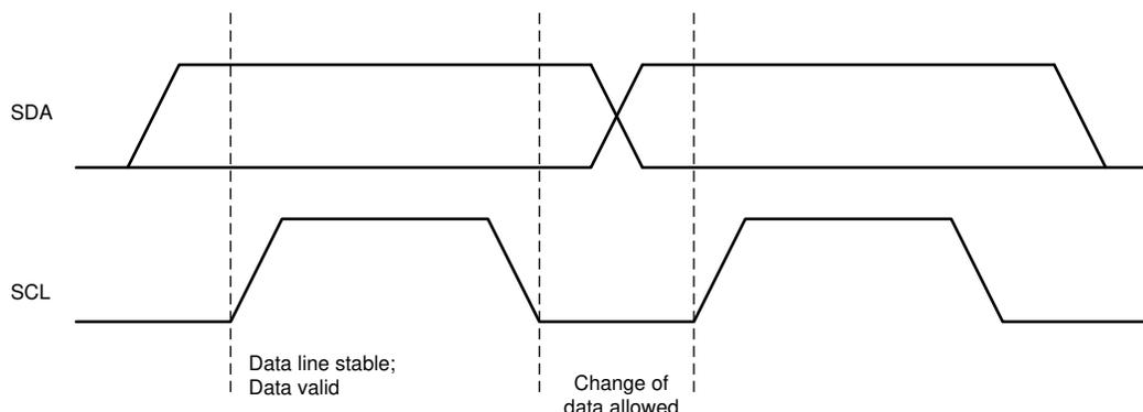
Figure 29. Bit Transfers on the I<sup>2</sup>C Bus
