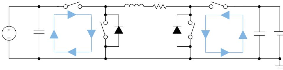
**Figure 112. Buck-Boost Converter High Frequency Current Path**
