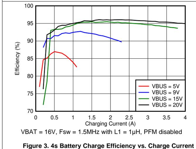
Figure 3. 4s Battery Charge Efficiency vs. Charge Current
