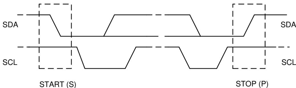
Figure 30. START and STOP Conditions on the I<sup>2</sup>C Bus
