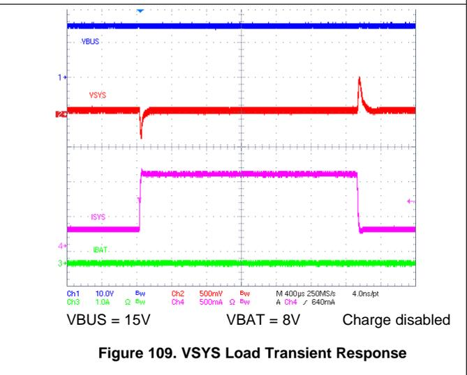
$C_{VBUS} = 2 \cdot 10 \mu\text{F}$ ,  $C_{PMID} = 3 \cdot 10 \mu\text{F}$ ,  $C_{SYS} = 5 \cdot 10 \mu\text{F}$ ,  $C_{BAT} = 2 \cdot 10 \mu\text{F}$ ,  $L1 = 1 \mu\text{H}$  (SPM6530T-1R0M120),  $F_{sw} = 1.5\text{MHz}$ .
