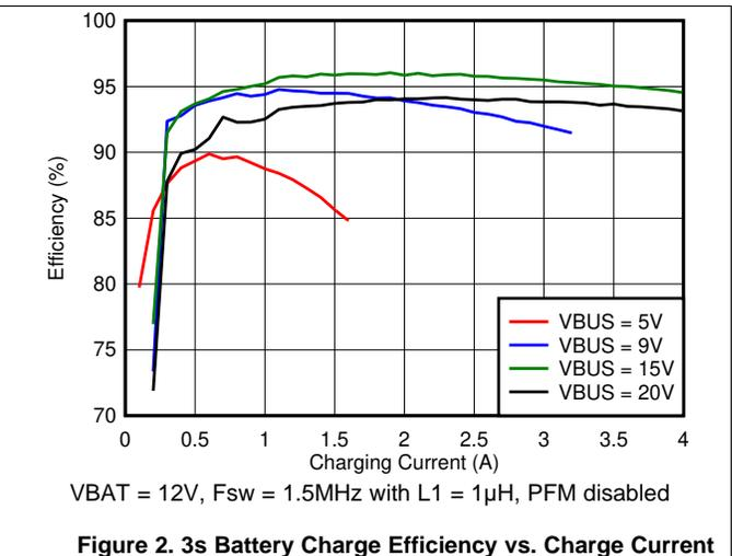
Figure 2. 3s Battery Charge Efficiency vs. Charge Current
