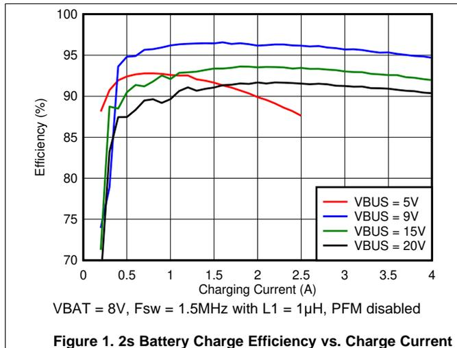
Figure 1. 2s Battery Charge Efficiency vs. Charge Current
