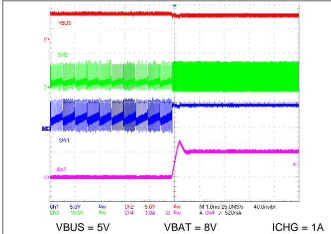
**Figure 100. Charge Enable**
