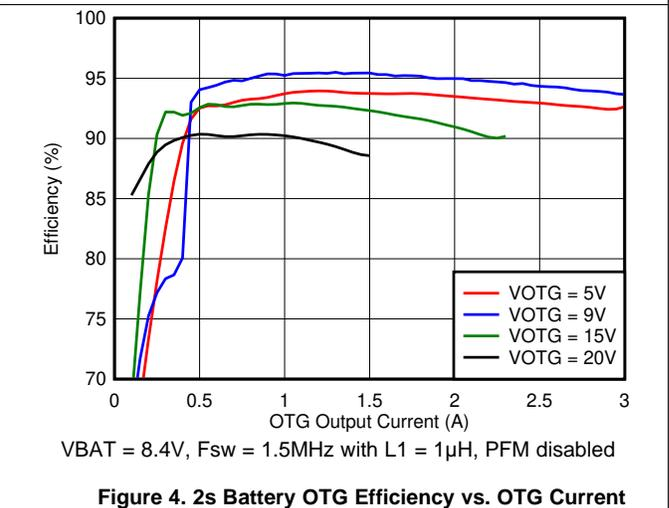
Figure 4. 2s Battery OTG Efficiency vs. OTG Current
