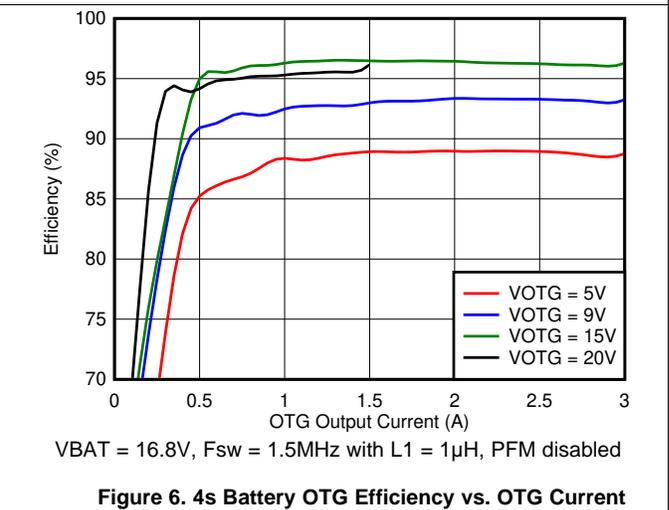
Figure 6. 4s Battery OTG Efficiency vs. OTG Current
