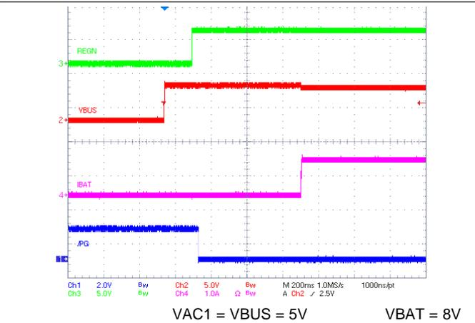
**Figure 99. Power Up from VAC1 with Charge Enabled**
