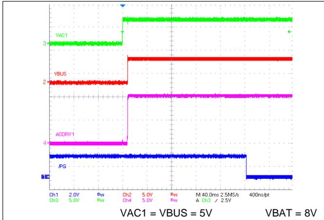
**Figure 98. ACFET1-RBFET1 Turns on at Power Up**
