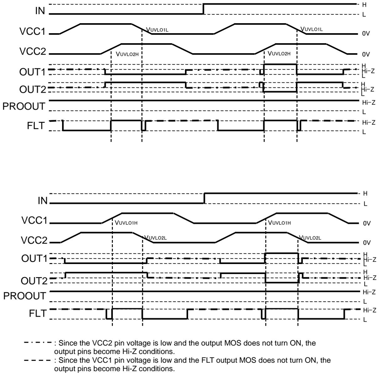
Figure 14. Power supply startup / shutoff sequence
