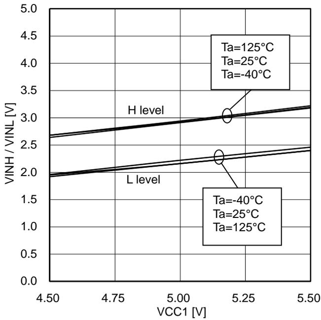
Figure 28. Logic (INA/INB) High/Low level input voltage
