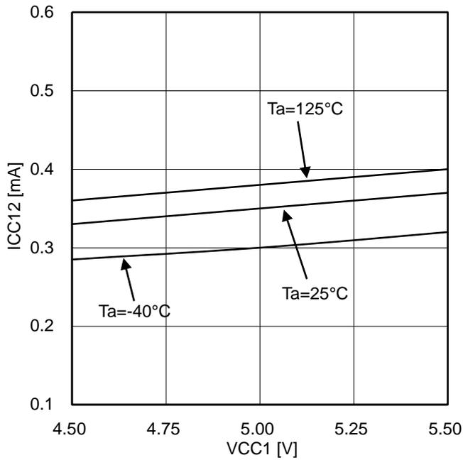
Figure 18. Input side circuit current (at OUT1=H)
