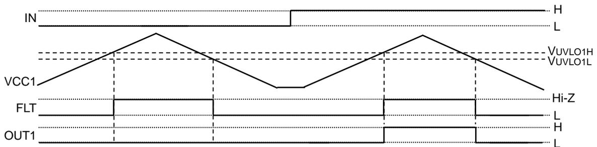
Figure 7. Input-side UVLO Function Operation Timing Chart
