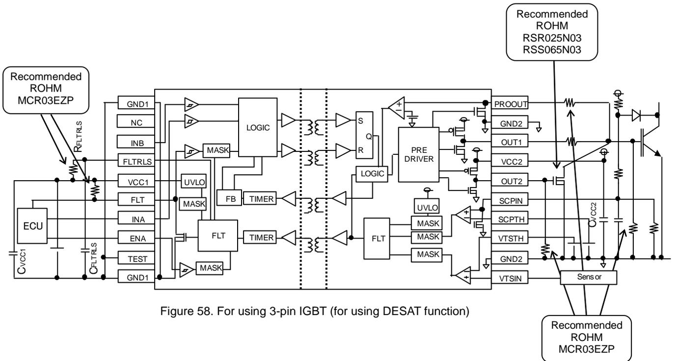
Figure 58. For using 3-pin IGBT (for using DESAT function)
