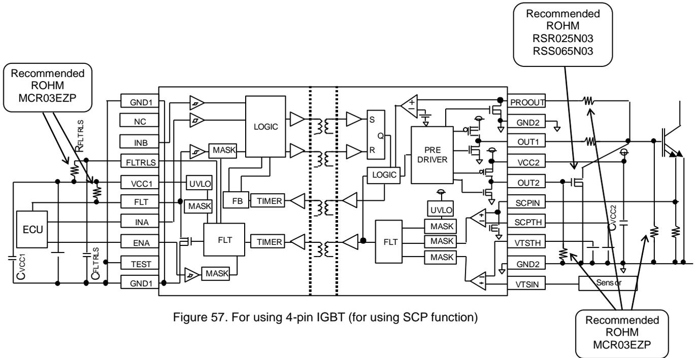
Figure 57. For using 4-pin IGBT (for using SCP function)
