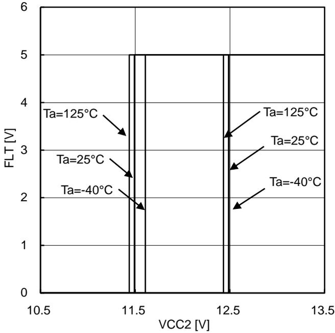
Figure 48. VCC2 UVLO ON/OFF voltage (at VCC1=5V)
