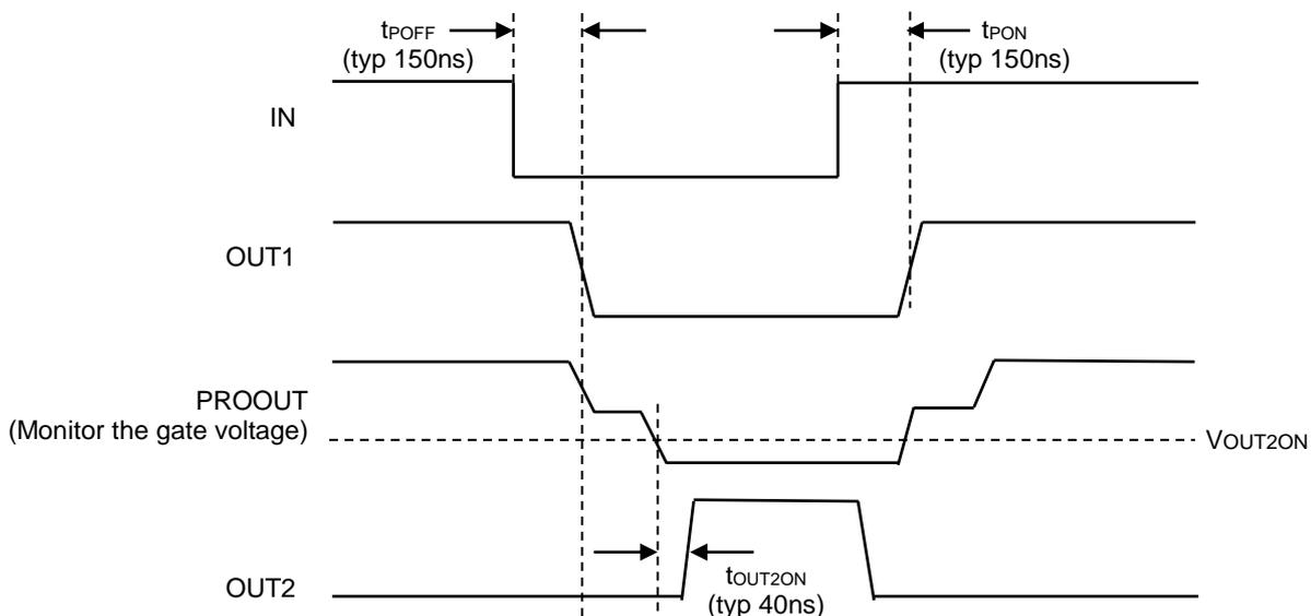
Figure 4. Timing chart of Miller Clamp function
