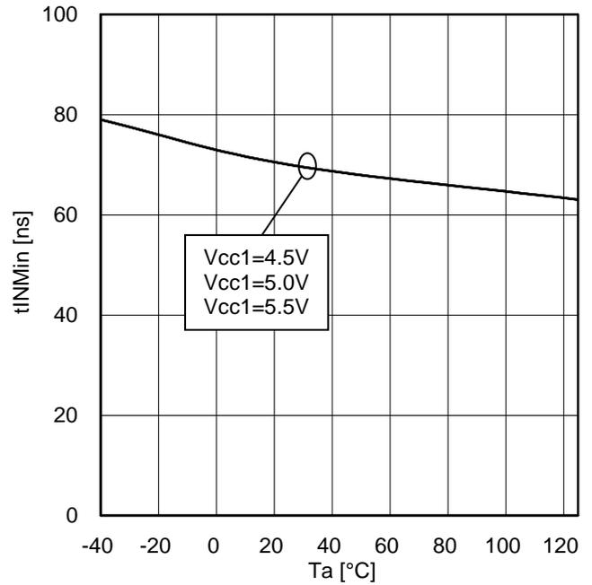
Figure 31. Logic input minimum pulse width (H pulse)
