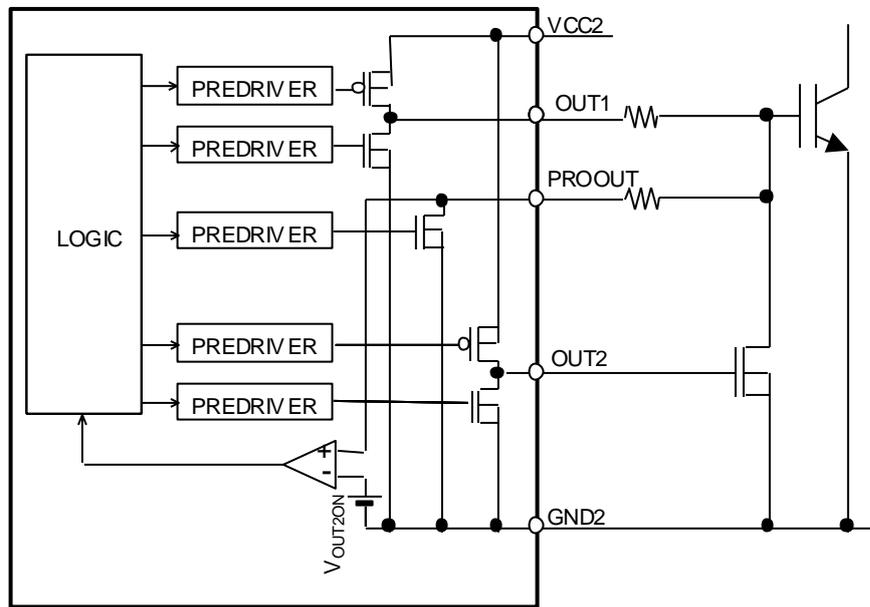
Figure 3. Block diagram of Miller Clamp function
