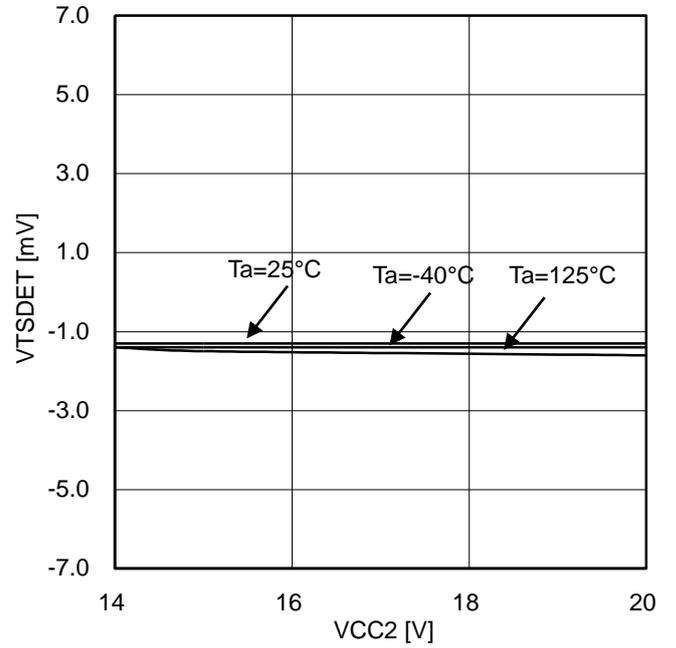
Figure 53. VTS offset voltage (at  $V_{TSTH}=1.7V$ )
