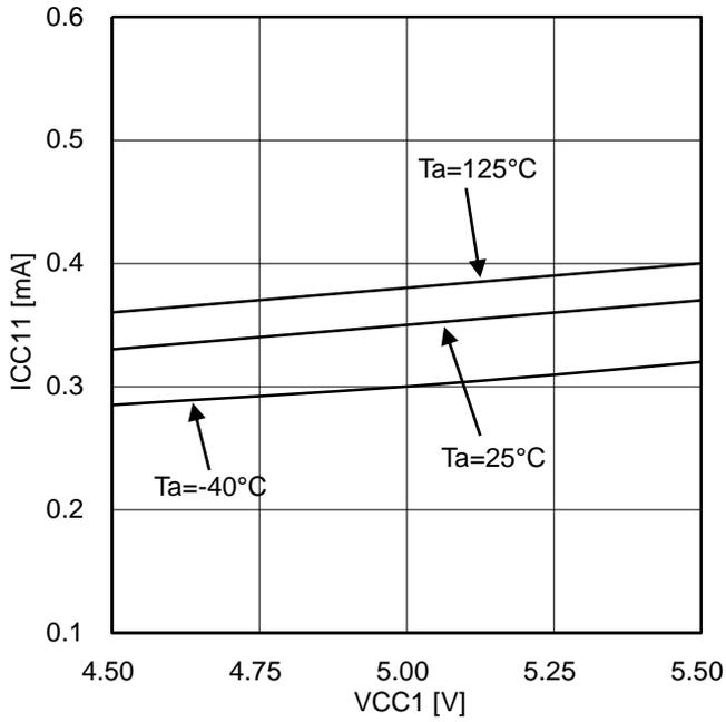
Figure 16. Input side circuit current (at OUT1=L)
