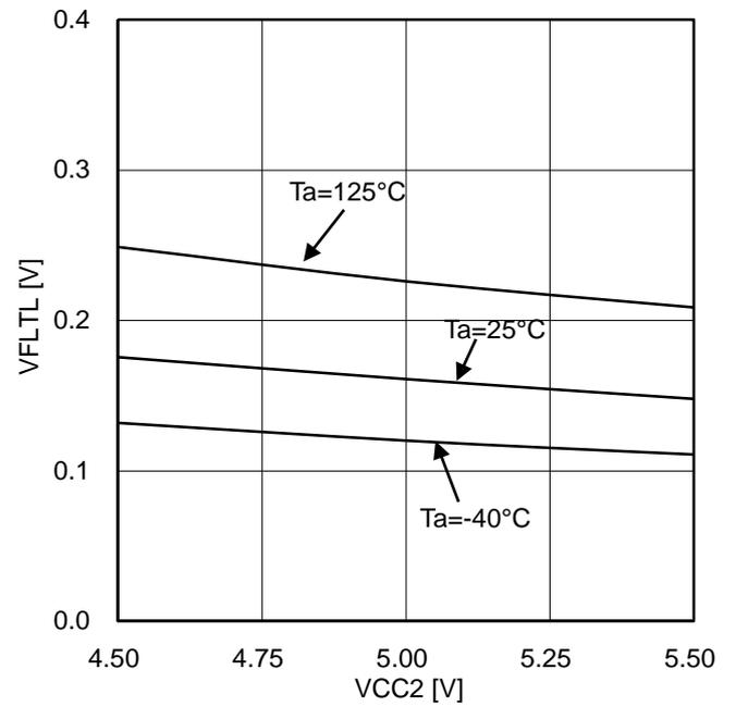
Figure 55. FLT output low voltage ( $I_{FLT}=5mA$ )
