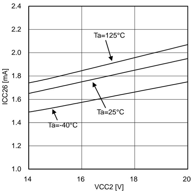
Figure 26. Output side circuit current (at OUT1=H)
