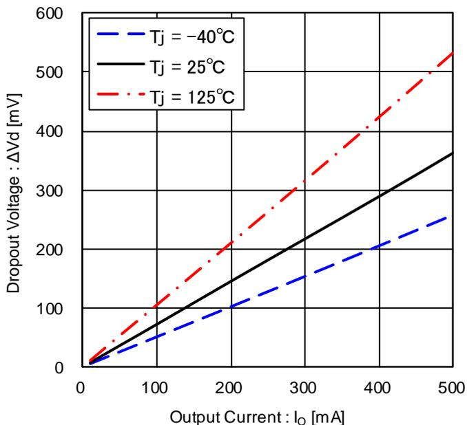
Figure 13. Dropout Voltage vs Output Current (V<sub>CC</sub> = 4.75 V)
