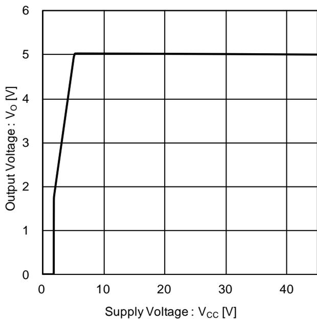
Figure 5. Output Voltage vs Supply Voltage ( $R_L = 25\ \Omega$ )
