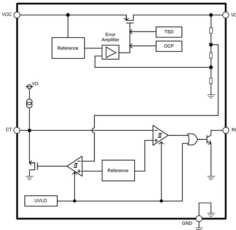
Figure 4. Block Diagram
