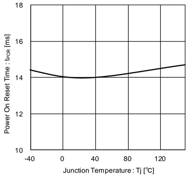
Figure 18. Power on Reset Time vs Temperature (C<sub>CT</sub> = 0.1 μF)
