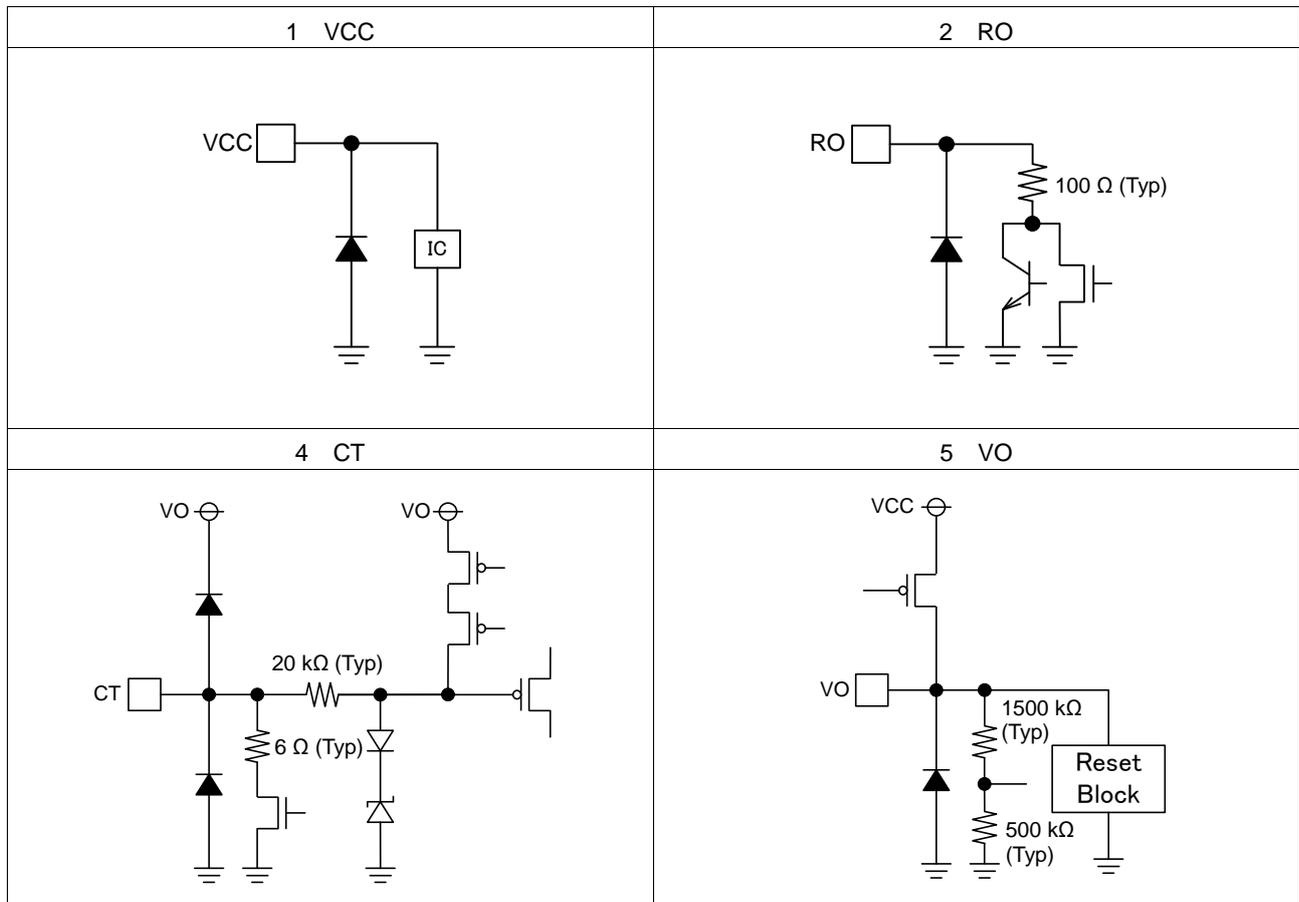
Figure 24. I / O equivalence circuits
