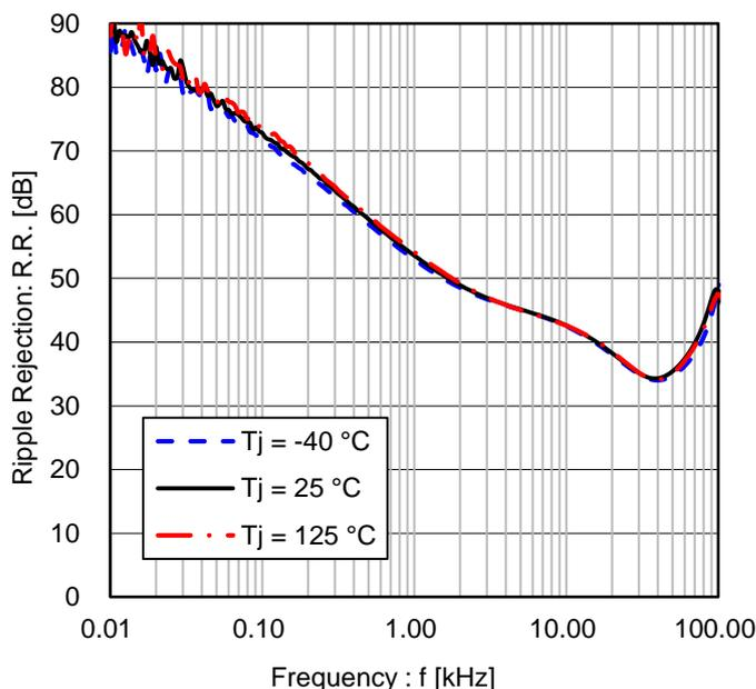
Figure 14. Ripple Rejection (e<sub>in</sub>=1V<sub>rms</sub>, I<sub>OUT</sub>=100mA)
