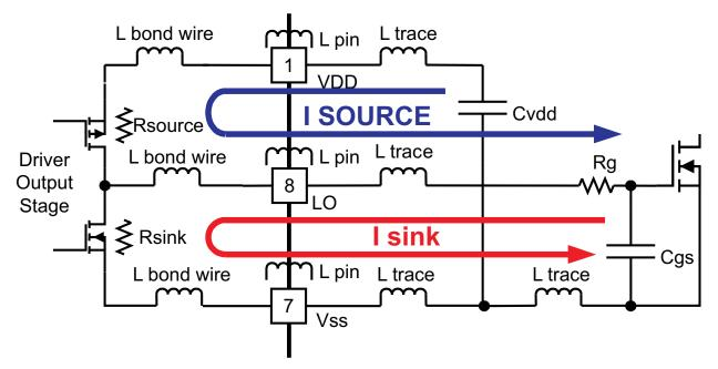
Figure 23. MOSFET Drive Paths and Circuit Parasitics
