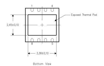
NOTE: All linear dimensions are in millimeters
