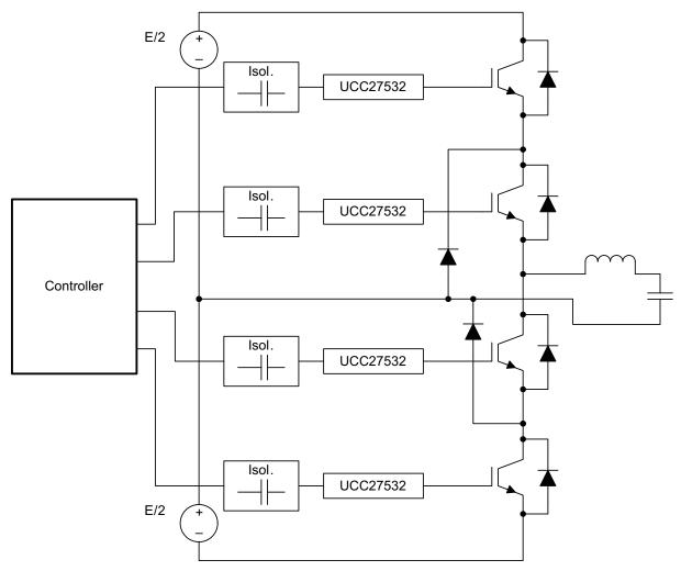
Figure 4. Using UCC27532 Drivers in an Inverter
