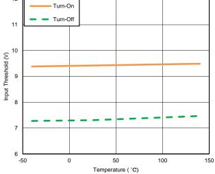
Figure 12. Input Threshold vs. Temperature
