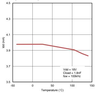
Figure 9. Start-Up Current vs. Temperature
