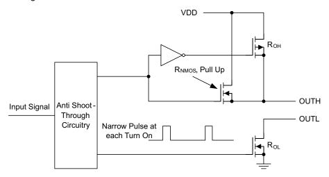
Figure 24. UCC27532 Gate Driver Output Stage
