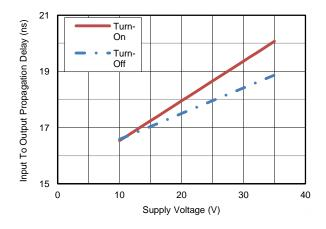
Figure 7. Propagation Delay vs. Supply Voltage
