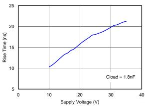
Figure 5. Rise Time vs. Supply Voltage
