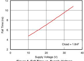
Figure 6. Fall Time vs. Supply Voltage
