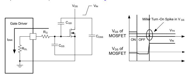
Figure 25. Low Pull-Down Impedance in UCC27532 (output stage mitigates Miller turn-on effect)
