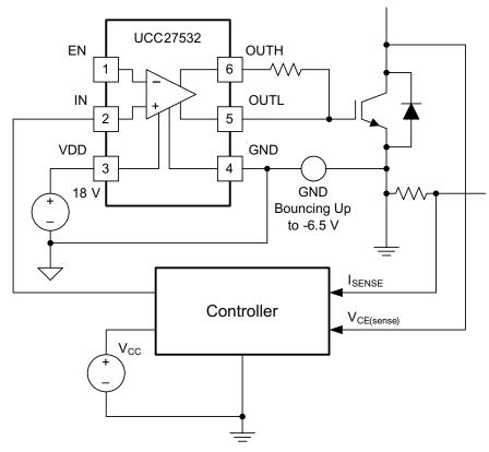
Figure 2. Driving IGBT Without Negative Bias
