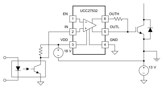
Figure 3. Driving IGBT With 13-V Negative Turn-Off Bias
