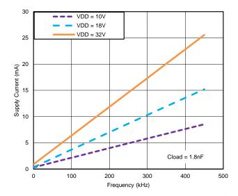
Figure 8. Operating Supply Current vs. Frequency
