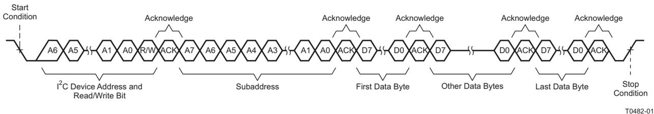
Figure 18. Multiple-Byte Write Transfer
