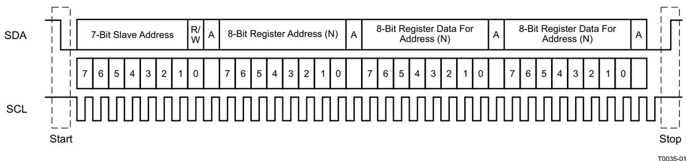
Figure 16. Typical I<sup>2</sup>C Sequence
