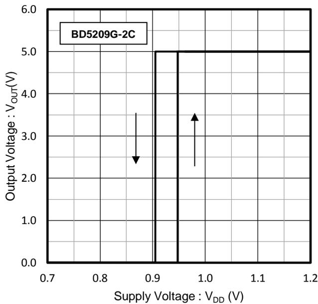
Figure 11. Detection Voltage
