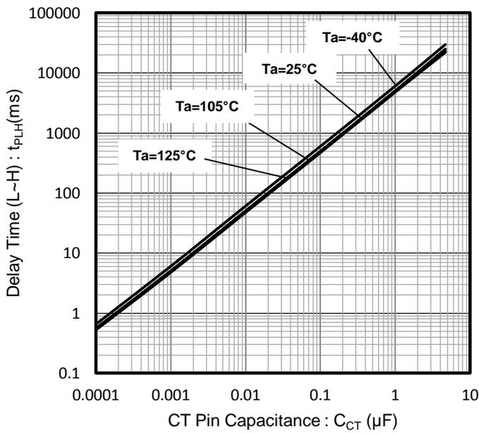
Figure 27. Output Delay Time (L to H)
