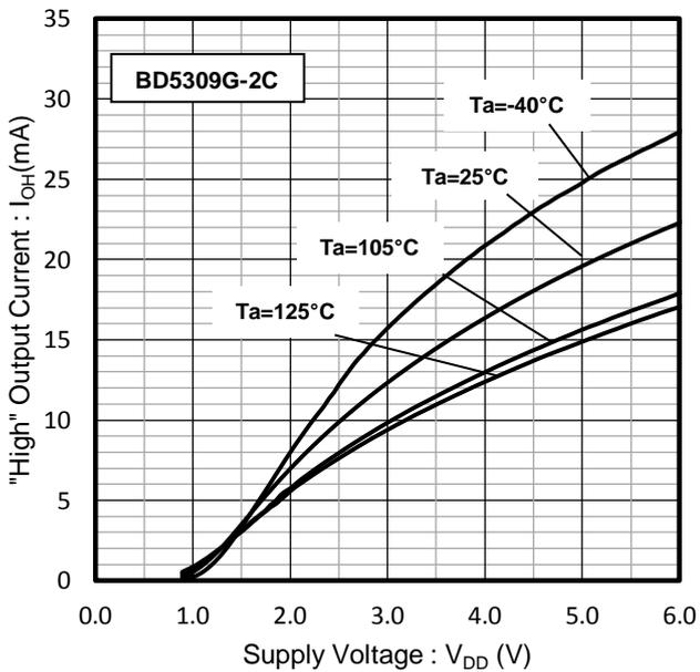
Figure 23. "High" Output Current ( $V_{DS}=0.5$ V)
