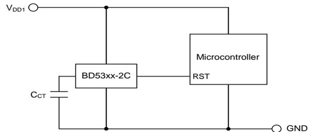
Figure 2. CMOS Output Type
