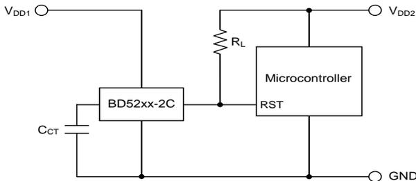
Figure 1. Open Drain Output Type
