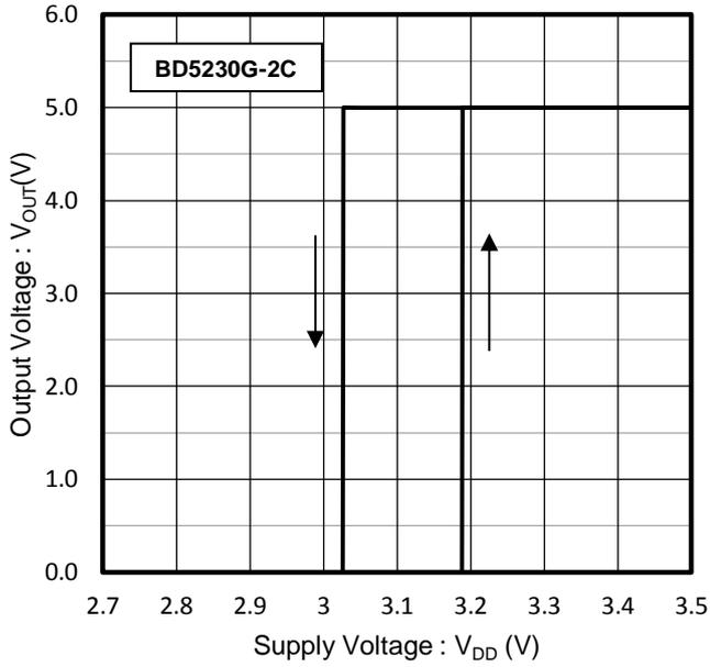
Figure 13. Detection Voltage
