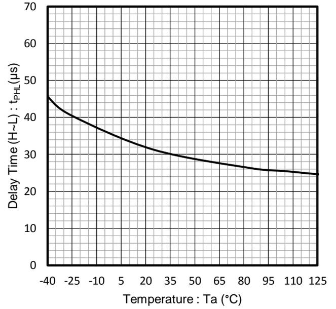
Figure 26. Output Delay Time (H to L)
