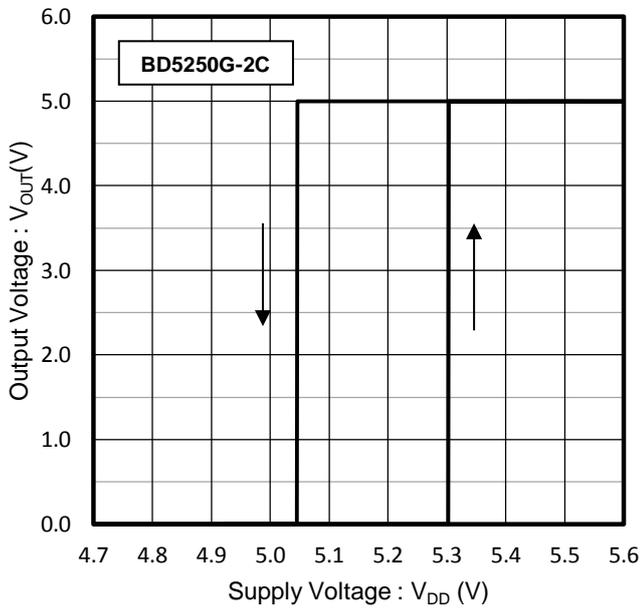
Figure 15. Detection Voltage
