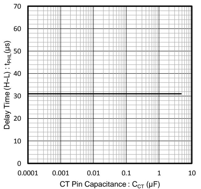
Figure 28. Output Delay Time (H to L)
