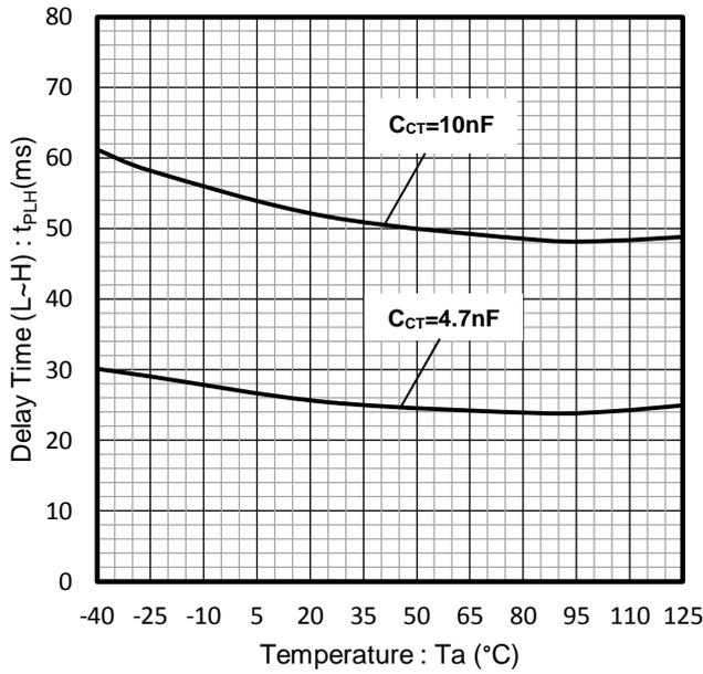
Figure 25. Output Delay Time (L to H)
