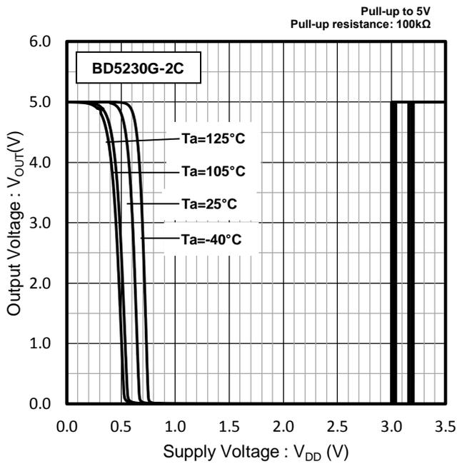
Figure 17. I/O Characteristics
