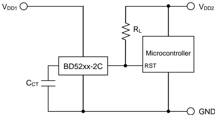
Figure 33. Open Drain Output Type
