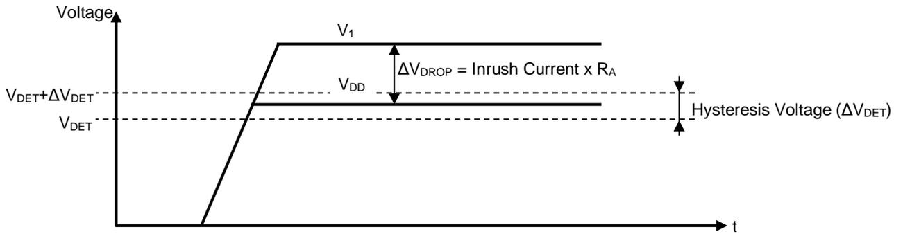
Figure 40.  $V_{DD}$  Drop Caused by Inrush Current
