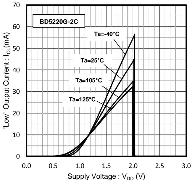
Figure 24. "Low" Output Current ( $V_{DS}=0.5$ V)
