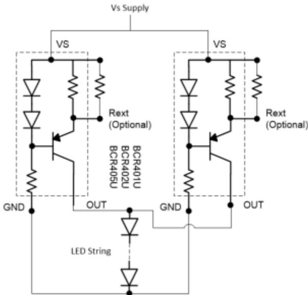
Figure 2 Application Circuit for Increasing LED Current
