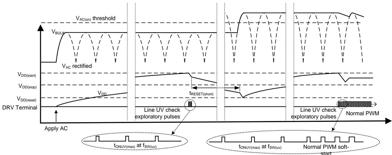
**Figure 17. AC Input UVLO Detection and Start Up**
