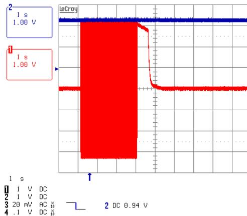
Figure 19. X-Capacitor Discharge Activation, at 230 V<sub>AC</sub>, No Load
