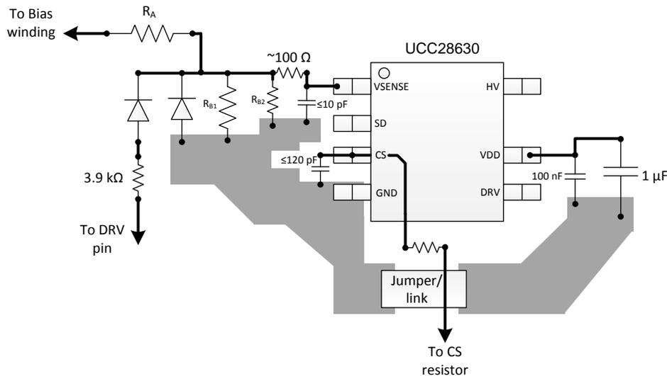
Figure 63. Recommended PCB Layout for Single-Sided Assembly
