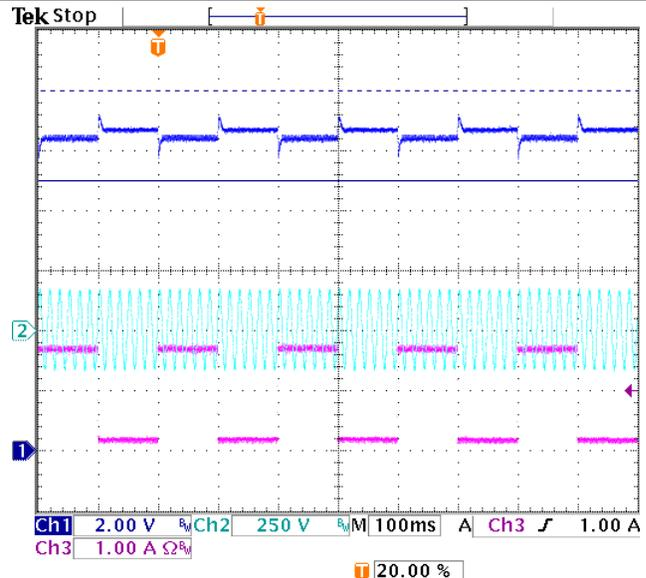
Figure 58. Transient Step 5% to 50% Load, 115 V<sub>AC</sub>
