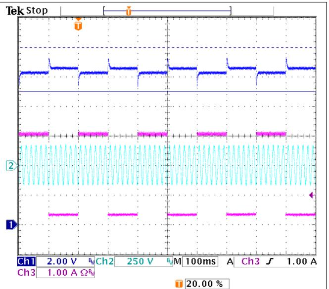
Figure 60. Transient Step 10% to 90% Load, 115 V<sub>AC</sub>
