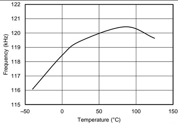
Figure 9. F<sub>SW(max)</sub> vs. Temperature
