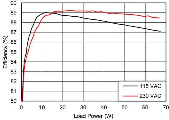
Figure 53. Efficiency vs. Load/Line (cable drop included)
