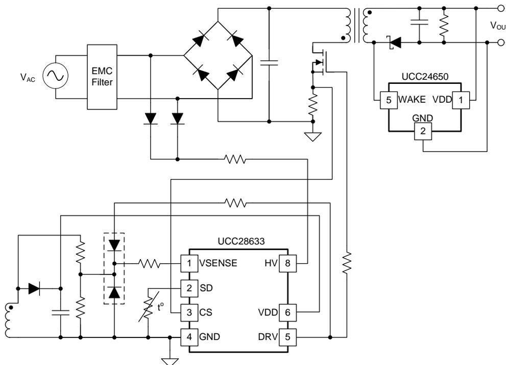
Figure 39. UCC24650 Secondary-Side Voltage Monitor and Wake-Up Circuit
