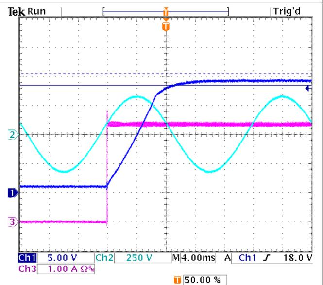
Figure 52. Output Rise-Time, 230-V<sub>AC</sub>, 3.35 A CC Load
