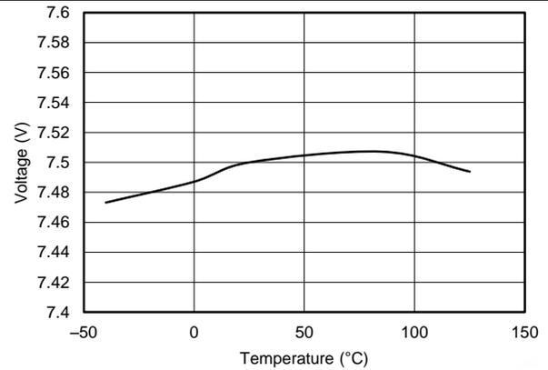
Figure 8. V<sub>OUT(ref)</sub> vs. Temperature
