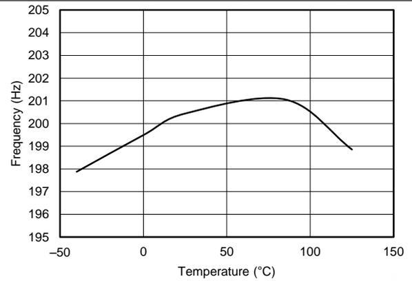
Figure 10. F<sub>SW(min)</sub> vs. Temperature
