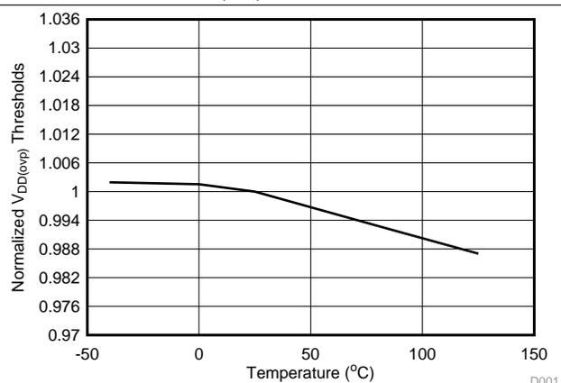
Figure 6. Normalized  $V_{DD(ovp)}$  Threshold vs. Temperature
