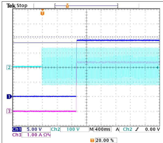
Figure 49. Start-Up from 90-V<sub>AC</sub>, 3.35-A CC Load
