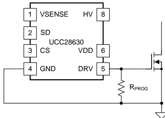
**Figure 36. Overload Timer Setting Adjustment
