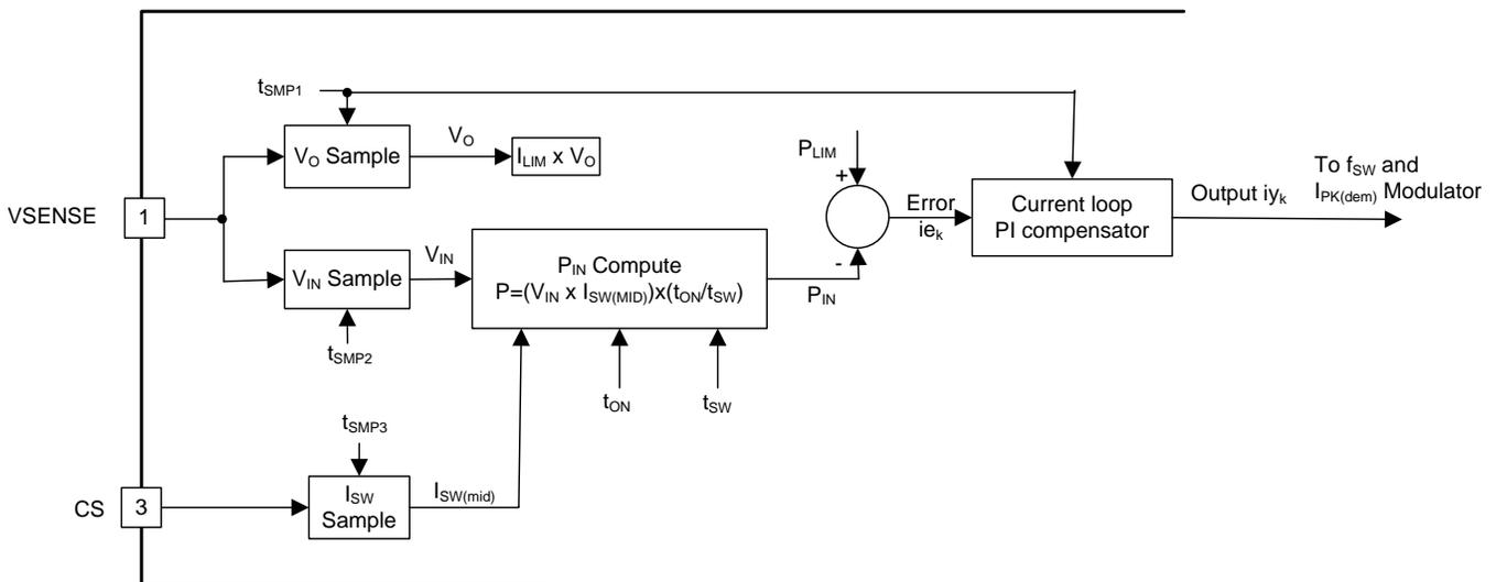
Figure 33. Digital Current Control Loop Simplified Block Diagram
