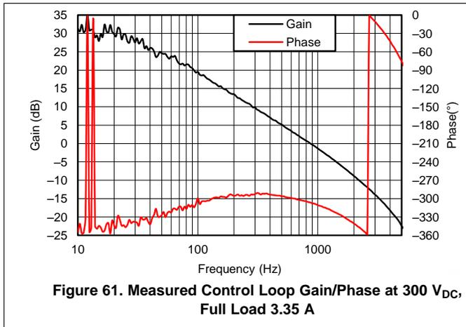
Figure 61. Measured Control Loop Gain/Phase at 300 V<sub>DC</sub>, Full Load 3.35 A
