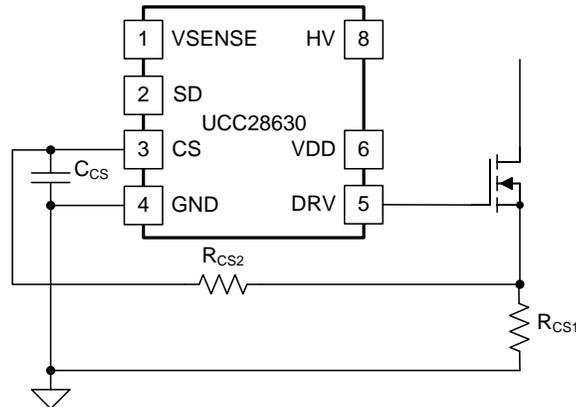
Figure 30. Primary-Side Current Sensing
