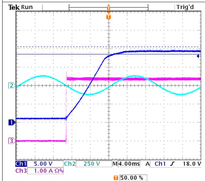
Figure 51. Output Rise-Time, 90-V<sub>AC</sub>, 3.35-A CC Load
