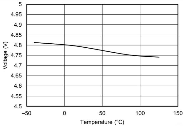
Figure 7. V<sub>DD(reset)</sub> Threshold vs. Temperature
